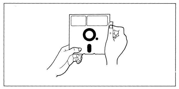
Figure 3-5 Write Protecting Diskette
