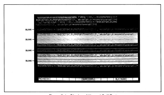
Figure 7-1 Display of Normal Self-Test
