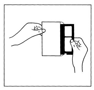
Figure 3-4 Removing Diskette From Jacket
