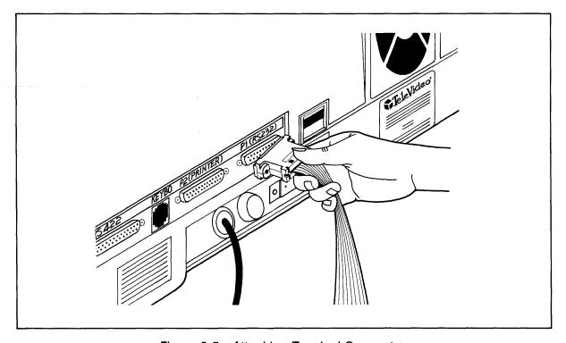
Figure 2-5 Attaching Terminal Connector
