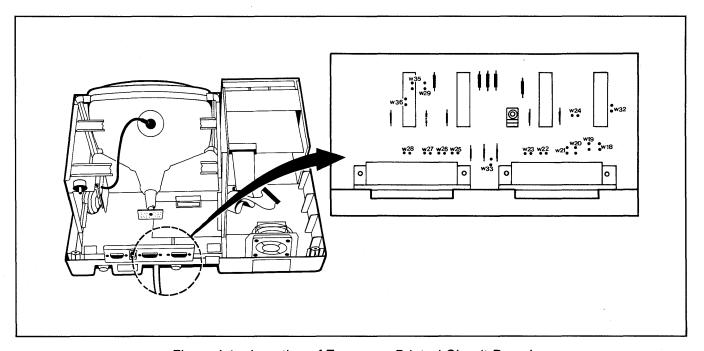
Figure I-1 Location of Traces on Printed Circuit Board
