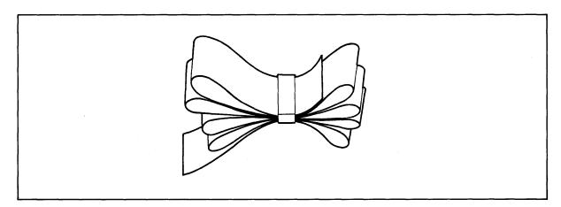
Figure 2-4 Correctly Folded Excess Cable
