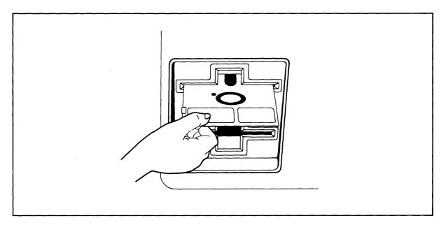
Figure 3-7 Inserting Diskette in Drive A
