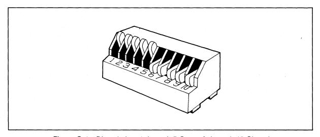
Figure G-1 Dipswitches 1 through 5 Open; 6 through 10 Closed
