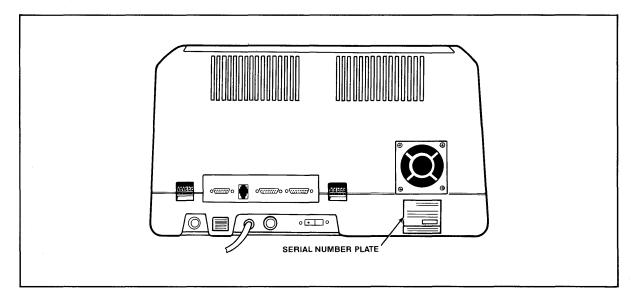
Figure 7-5 Location of Serial Number on Rear Panel
