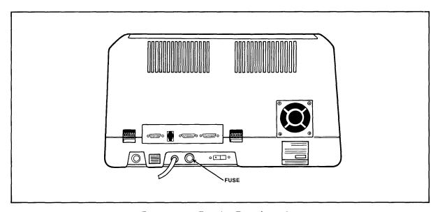
Figure 7-2 Exterior Fuse Location
