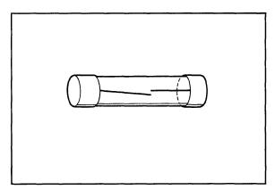
Figure 7-4 Burned Out Fuse
