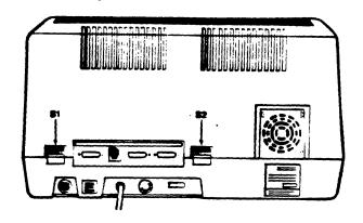
Figure 2-6 Location of Switches on Rear Panel
