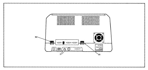
Figure 2-6 Location of Switches on Rear Panel
