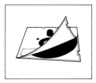
Figure 1-3 Diskette Inside Permanent Plastic Enclosure
