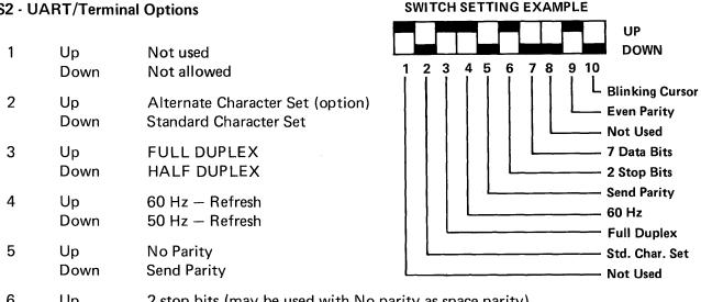
6 Up 2 stop bits (may be used with No parity as space parity) Down 1 stop bit
