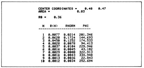
Running a Fourier series computation for unequally spaced data for 10 harmonics on the digitized crater produced the center of gravity, average area and average radius of the crater in the plane of interest. The amplitude, amplitude normalized for an average radius  $R \mathcal{D}$  of one, and the phase for each harmonic was also computed.
