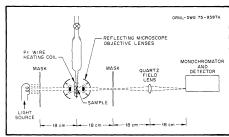
Fig. 1. Schematic diagram of microscope spectrophotometer.
