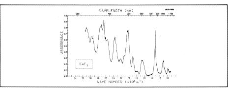
Fig. 11. Absorption spectrum of EsF $_3$ .
