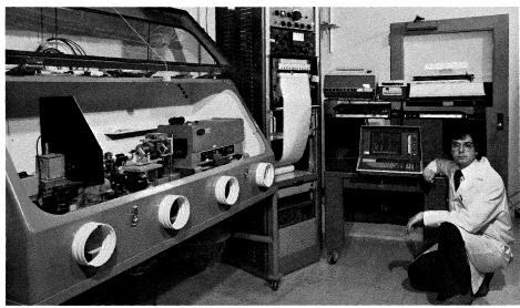
Fig. 2. Microscope spectrophotometer and Tektronix 4051 system.
