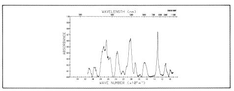
Fig. 12. Absorption spectrum (flattened) of EsF<sub>3</sub>.
