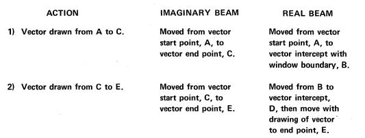
Fig. 3.1. Imaginary and Real Beams.
