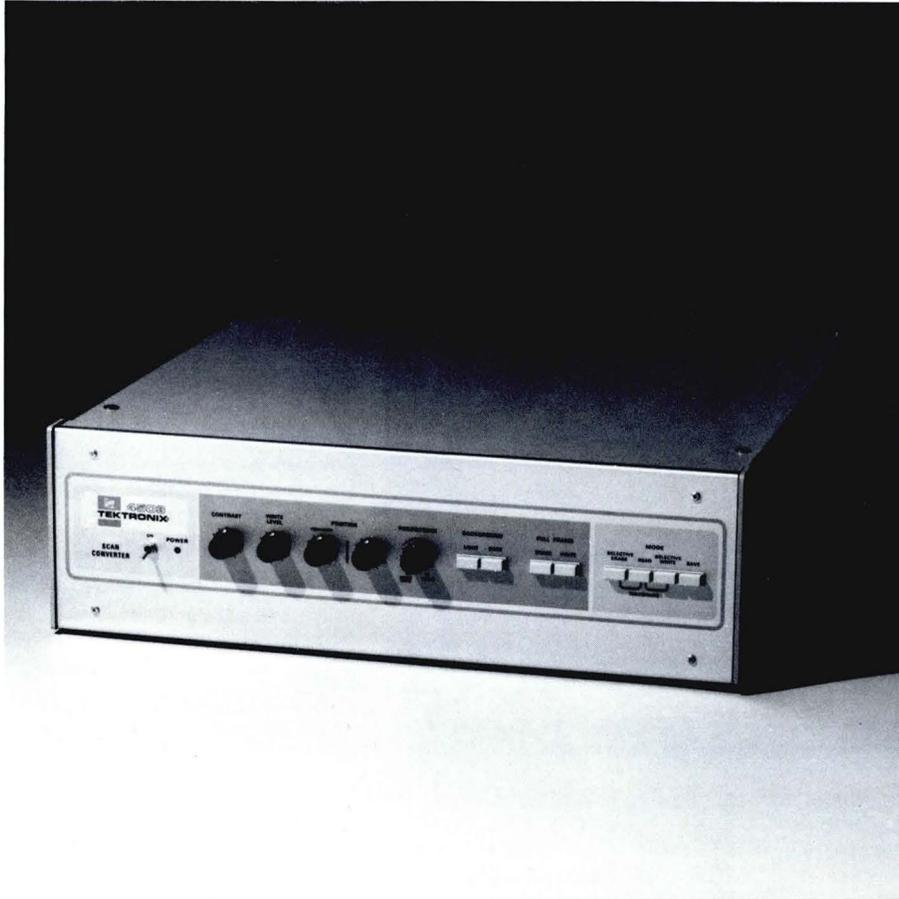
The 4503 Scan Converter stores and converts analog input signals to a television video waveform for displaying on large screen TV monitors. It can integrate low level Z Axis input signals, frame freeze a vertical frame of video, selective erase portions of a display, store grey levels, and operate in a variable persistence mode.
