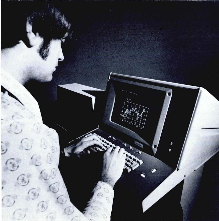
The 4012 Computer Display Terminal adds keyboard selection of the full ASCII set of 96 upper and lower case printing characters, or the 63 character TTY subset. In addition, the 4012 offers higher resolution graphics in two operational modes. Another advantage of the terminal is copying capability from the 4610 Hard Copy Unit.
