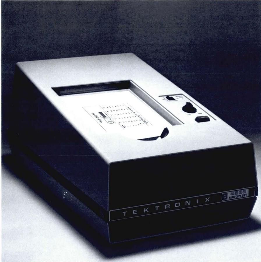
The 4632 Video Hard Copy Unit is designed to provide permanent hard copies from standard composite video signals and from digital video signals of refreshed alphanumeric/graphic terminals. The copies may be either high-contrast (black and white) or grey scale copies. Operation is simple and quiet, with dry-process development within one lightweight unit.
