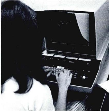
The 4002A Display Terminal offers three graphic modes (vector, point plot, and incremental plot) for graphic display flexibility. In alphanumeric operation, both upper and lower case alphabets are offered, with the full ASCII character set of 96 printing characters, plus the TTY upper case subset.
