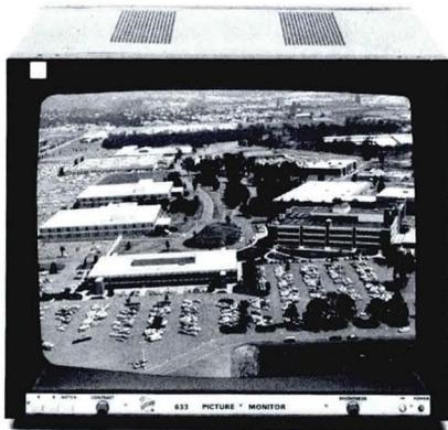
The 633 Monochrome Picture Monitor, when used with the 4503 Scan Converter, provides large screen display capabilities with excellent resolution.
