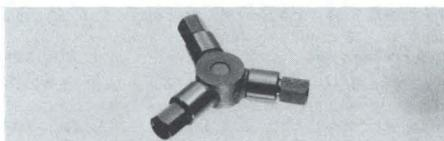
This coaxial tee is designed for use in broad-band 50 Ω systems where the mismatch introduced by ordinary "Tee" connectors is undesirable. Load isolation is nominally 6 dB while the voltage attenuation ratio is nominally 2X (input to either load arm, other load arm terminated in a standard 50 Ω termination). Maximum vswr is 1.50 from dc to 12.00 GHz and 1.90 from 12.01 to 18.00 GHz.
