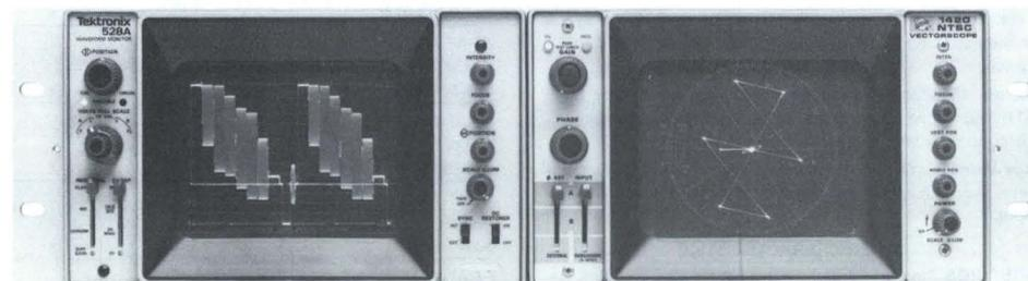
528A Waveform Monitor mounted side-by-side with a 1420 Vectorscope in optional rack adaptor.
