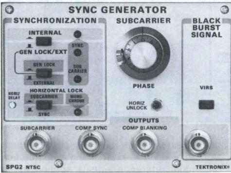
The SPG2 and SPG12 Sync Generators have gen-lock capability. The almost identical SPG1 and SPG11 do not.
