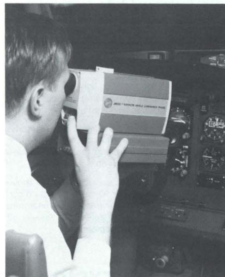
Measuring Luminance with the Tektronix J16/J6523.
