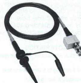
The P6125 is a low-capacitance, 5X attenuation passive probe specially designed for use with counter/timers. It makes possible more accurate time interval measurements of high speed logic signals. Five-times attenuation provides an optimum match between the counter input characteristics and the voltage levels of all common logic families. The low input capacitance permits acquisition of high frequency signals with minimum loading of the circuits under test.
