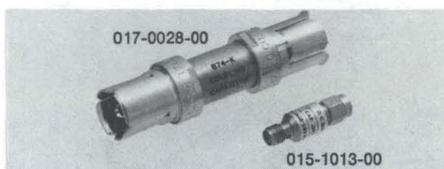
The coupling capacitor is a short length of coaxial line with a disk capacitor (4700 pF, ±20%) in series with the inner conductor. Reflection ratio (in 150 ps tdr system), is 0.03 maximum. Voltage rating is 200 V.
