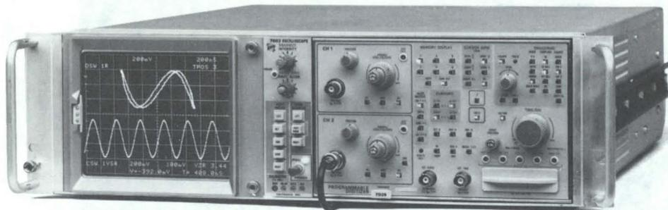
The R7603 requires only 5.25 in of rack height in a standard 19 in rack. It is fan cooled and comes complete with slide-out chassis tracks.
