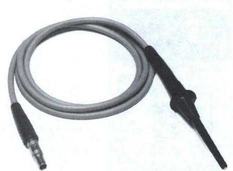
The P6601 Probe is a temperature measuring device designed to operate with the DM 502A and DM 501A Digital Multimeters. The temperature sensing element consists of a thin-film platinum resistor on the tip of the probe. Measurements are made by touching the sensing element to the surface whose temperature is in question. The thermal signal is transmitted to the associated digital multimeter through a two-conductor cable.
