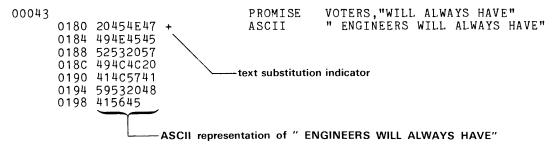
When the macro is invoked, the assembler processes the lines of the macro definition. The assembler listing shows us only the one source line that generates object code, namely:
