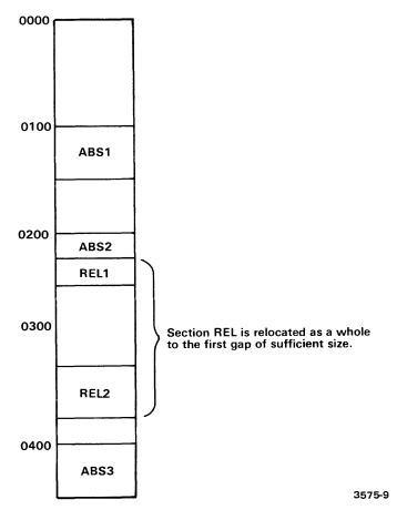
Notice that section REL is placed between blocks ABS2 and ABS3 of section ABS. Notice also that block REL2 began on a page boundary before it was relocated, but not after.
