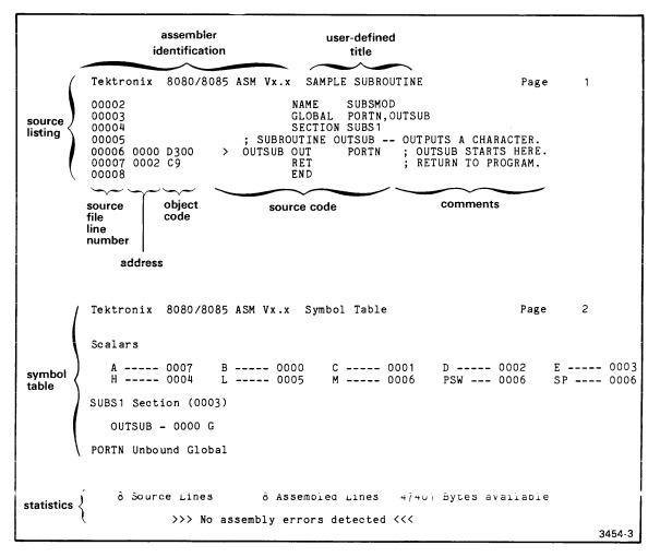
Fig. 1-3. Assembler listing for the sample subroutine.
