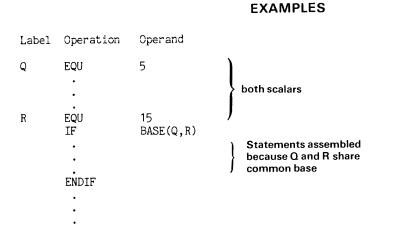
In this example, the two scalar values Q and R are compared. Since both Q and R represent scalar values, they share a common base. The function BASE(Q,R) returns a -1 (true) and the statement lines between IF and ENDIF are assembled.
