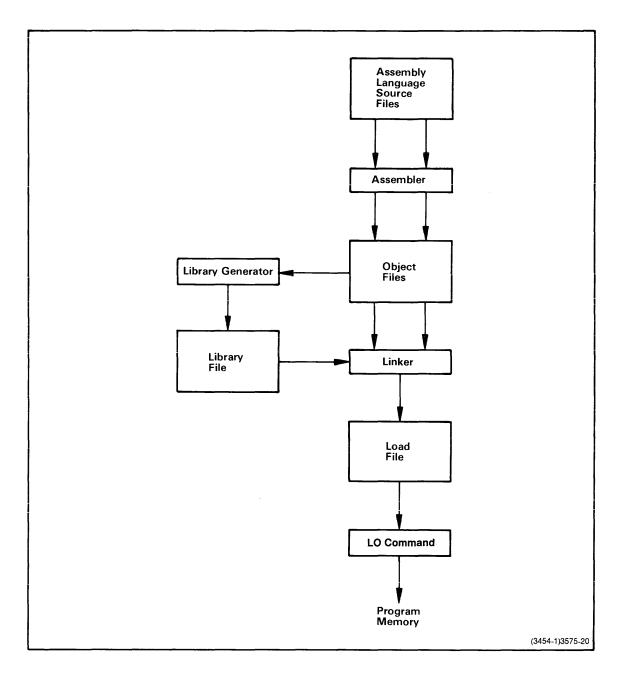
Fig. 1-1. Assembler programming process.
