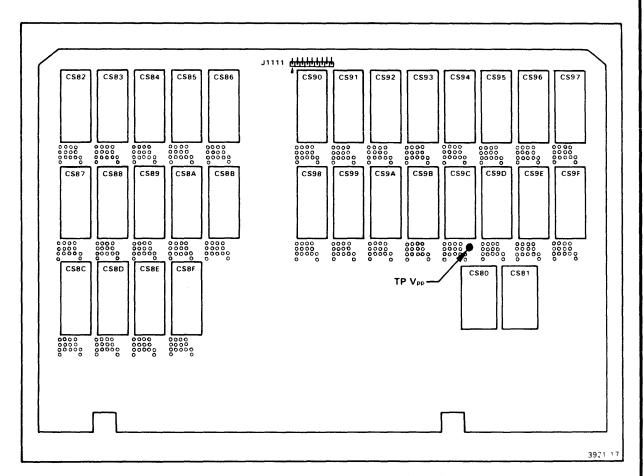
Fig. 3-4. System ROM Board socket locations.
