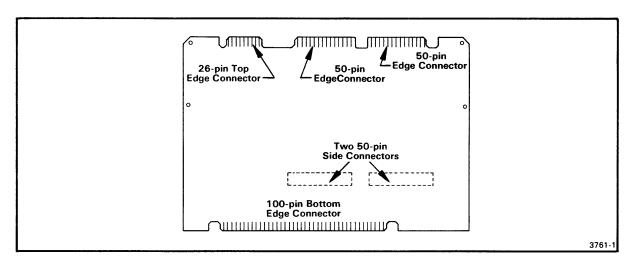
Fig. 1-1. TTA Circuit Board #1.
