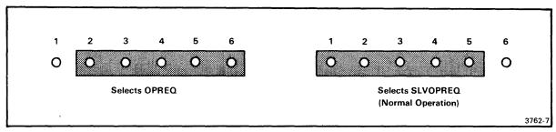
Fig. 2-3. OPREQ/SLVOPREQ selection: J1031.
