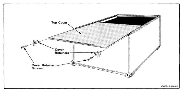
Fig. 3-1. Removing/installing the mainframe top cover.
