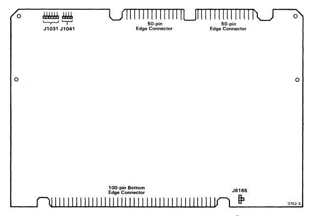
Fig. 2-1. Jumper locations, TTA Circuit Board #2.
