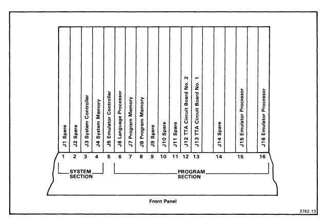
Fig. 3-2. Recommended circuit board arrangement.
