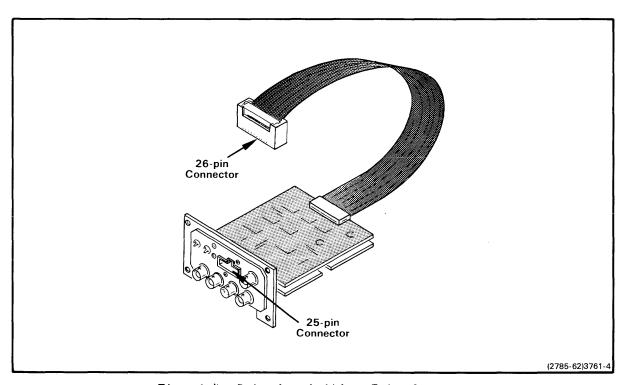
Fig. 1-4. Data Acquisition Interface.
