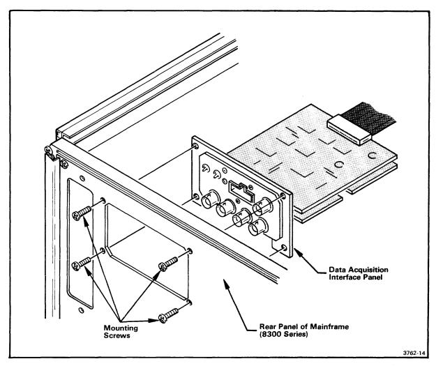
Fig. 3-3. Installing the Data Acquisition Interface.
