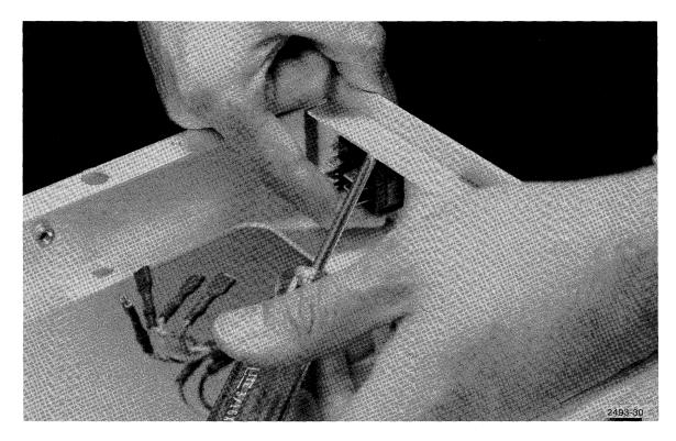
Figure 7-4. Removing power switch.
