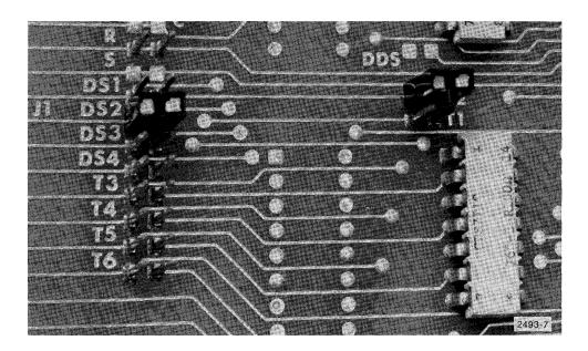
Figure 3-4. Setting for device address 1 (DS2).
