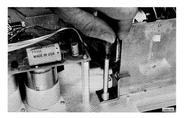
Figure 7-2. Loosening drive clamp.
