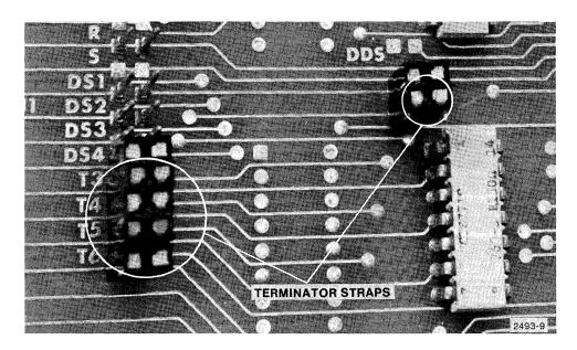
Figure 3-6. Setting for device address 3\* (DS4).
