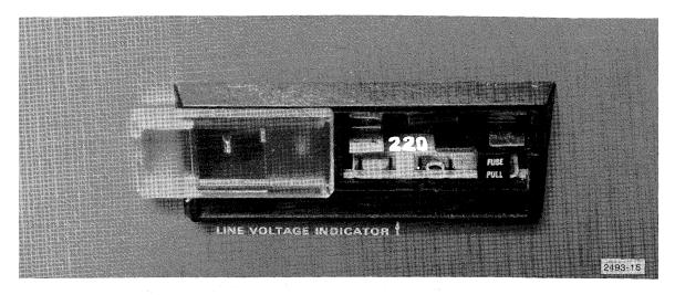
Figure 3-12. Card position for 220 V.
