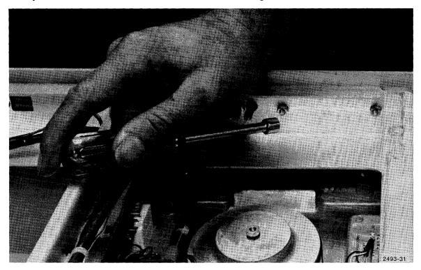
Figure 7-5. Removing front panel.
