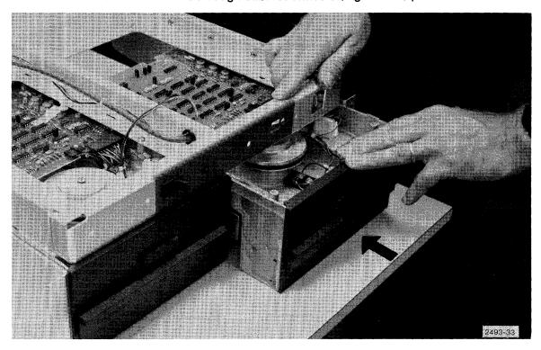
Figure 7-7. Sliding drive into chassis.
