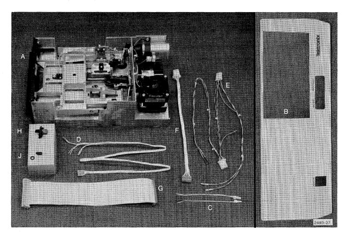
Figure 7-1. Field upgrade kit components.
