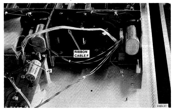
Figure 7-15. Installing ribbon cable F.
