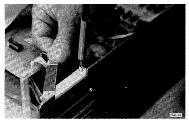
$\label{figure 5-3.} \textbf{Installing strain relief cable and clamp assembly}.$
