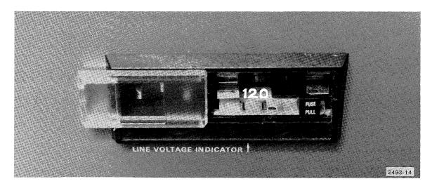
Figure 3-11. Card position for 120 V.
