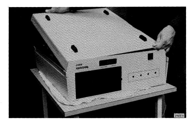
Figure 3-1. Removing base of drive cabinet.
