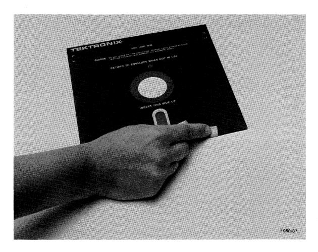
Figure 4-1. Covering the write-protect hole with tape.
