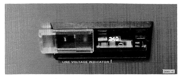
Figure 3-13. Card position for 240 V.
