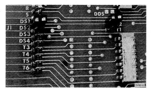
Figure 3-3. Setting for device address 0 (DS1).
