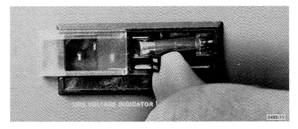
Figure 3-8. Removing fuse.
