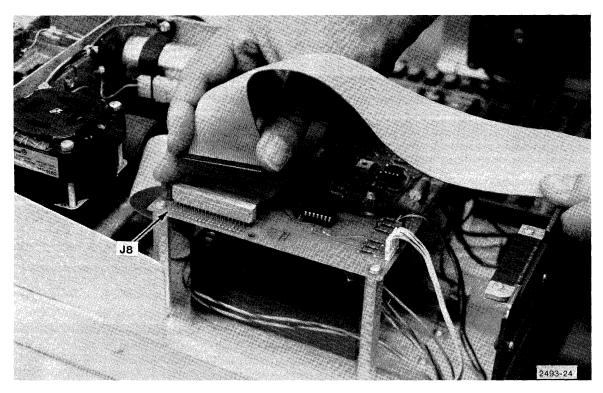
Figure 5-2. Connecting ribbon cable to J-8.
