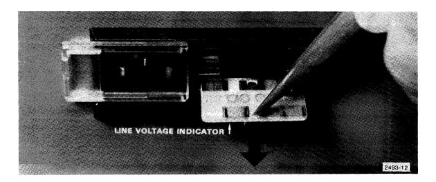
Figure 3-9. Removing line voltage selector card.
