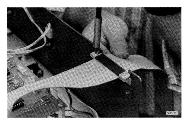
Figure 5-4. Securing ribbon cable at rear of main 4907 cabinet.
