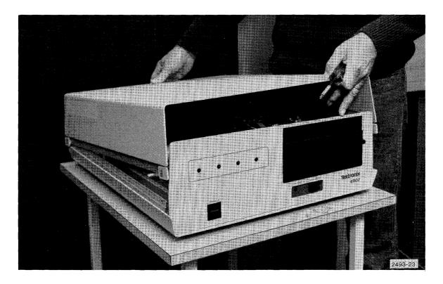
Figure 5-1. Removing main 4907 cabinet cover.
