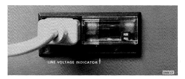
Figure 3-14. Attaching line cord to rear of cabinet.
