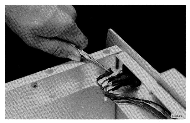
Figure 7-3. Removing power switch connectors.
