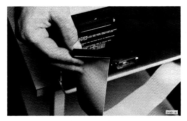
Figure 5-5. Attaching ribbon cable to J-1.
