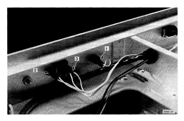
Figure 7-11. Connecting front panel leads of cable D.
