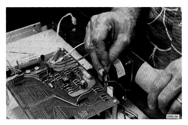
Figure 7-13. Connecting ribbon cable D to J-11.
