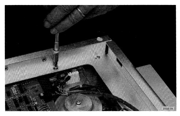
Figure 7-8. Reinstalling drive screws.
