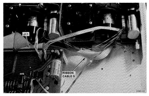
Figure 7-16. Installing ribbon cable G.
