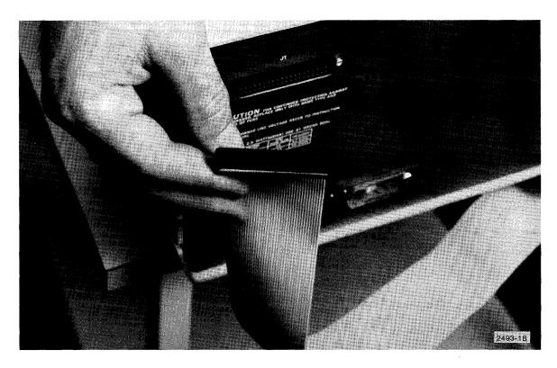
Figure 3-15. Plugging ribbon cable to connector J-1 on auxiliary cabinet.
