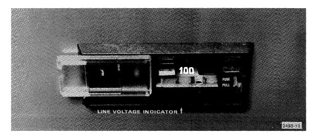
Figure 3-10. Card position for 100 V.
