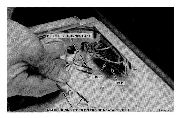
Figure 7-12. Placing new leads on line filter.
