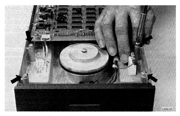
Figure 7-6. Removing screws from kit drive chassis.
