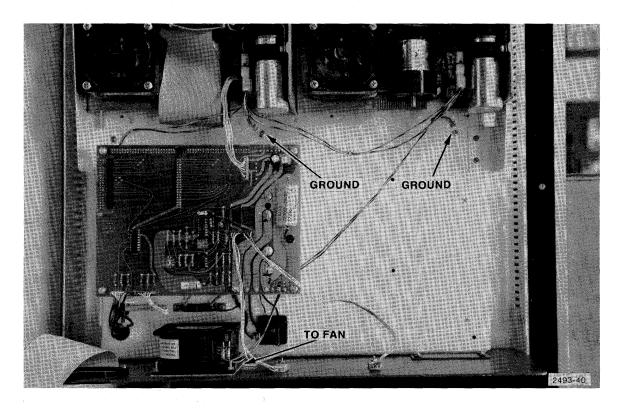
Figure 7-14. Wire set E in place including a single connector to each drive, two ground connections and two leads to the fan.
