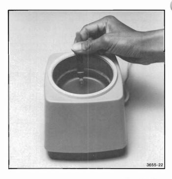
Figure 4-12. Using the Ultrasonic Tank to Clean Pen Tips.
