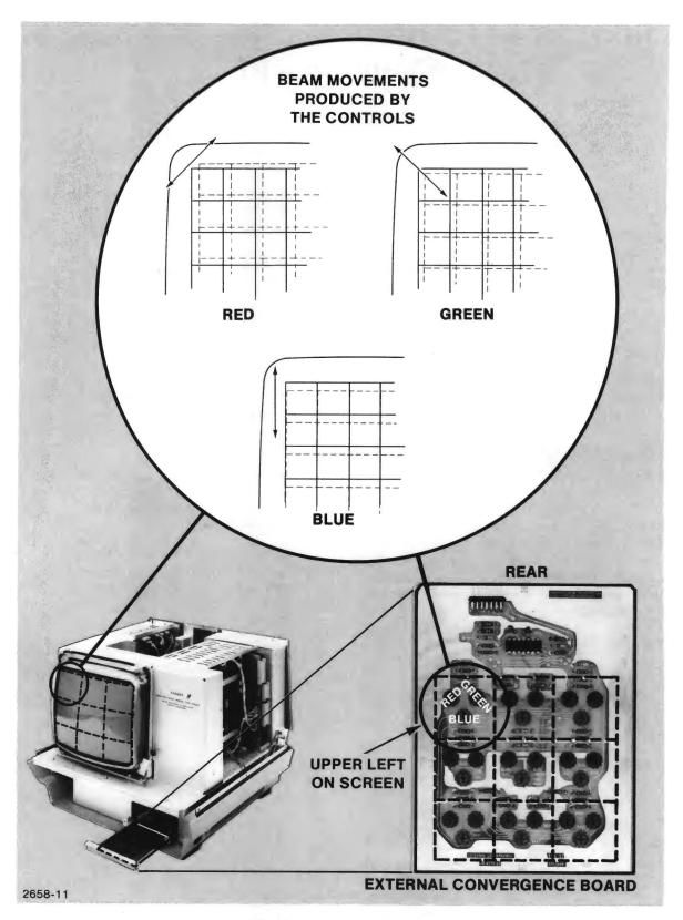
Figure I-1. Adjusting the External Convergence Board.
