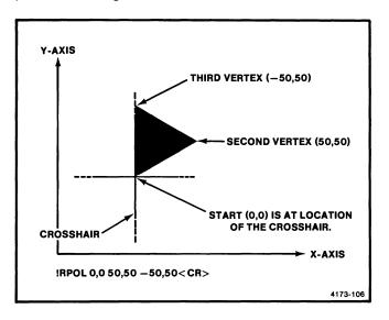
Figure 8-5a. AN RPOLY Command Using 0,0 as the First Coordinate Pair.
