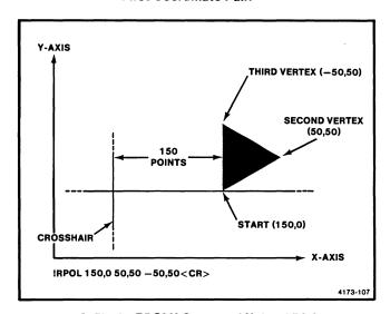
Figure 8-5b. An RPOLY Command Using 150,0 as the First Coordinate Pair.
