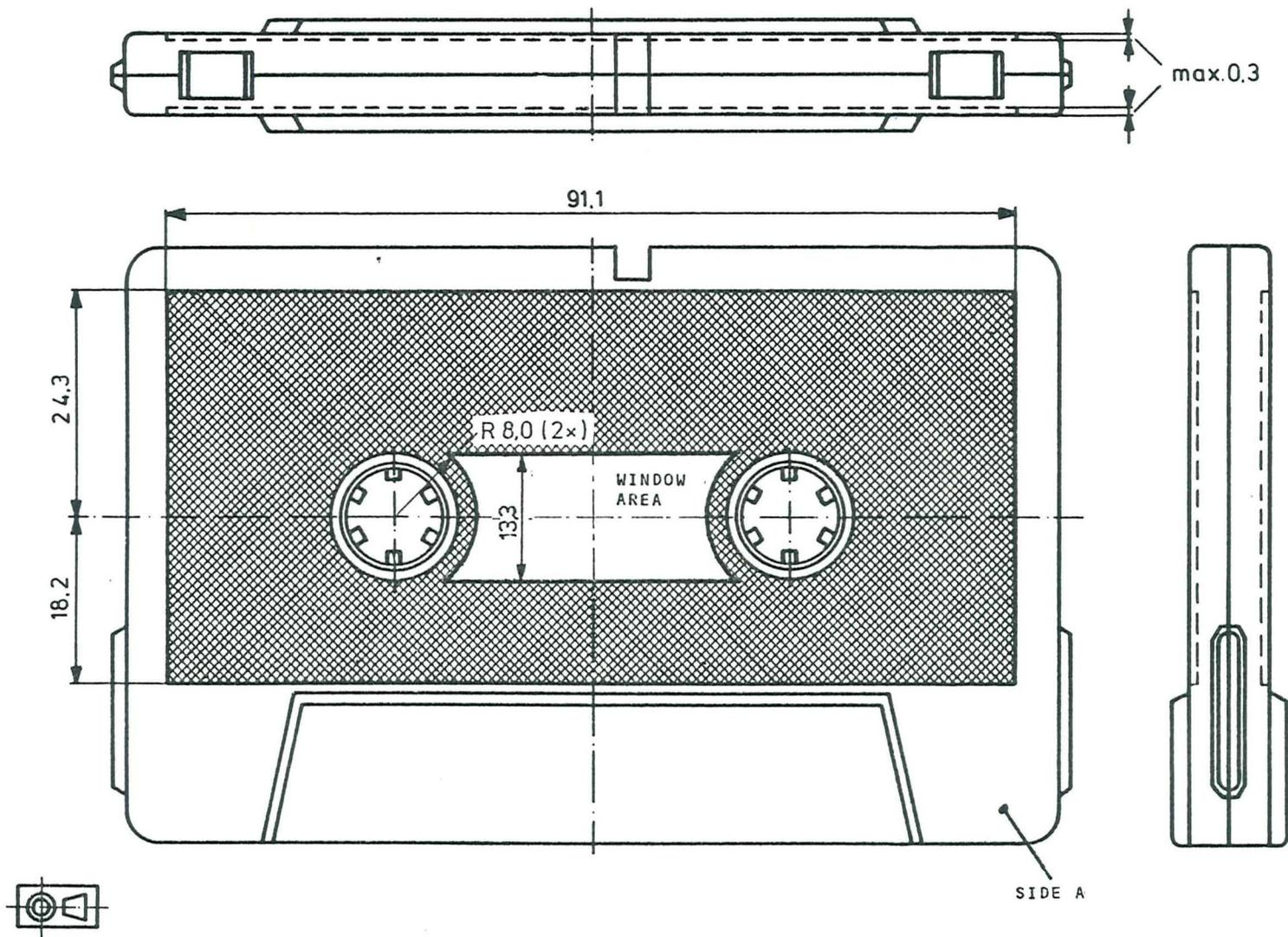
Fig. 6 Maximum label and window area dimensions
