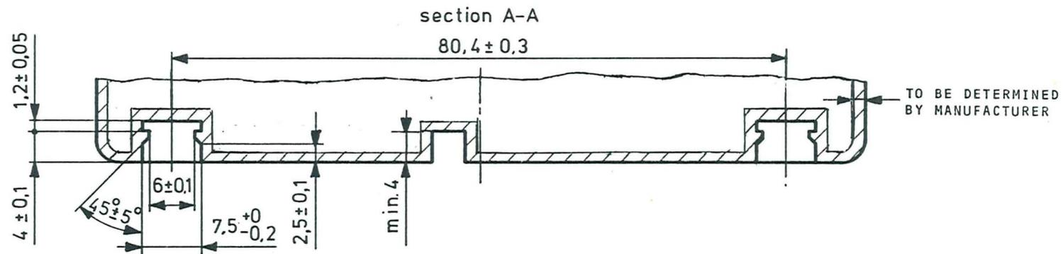
Fig. 1 Sides, track, holes and asymmetrical slot
