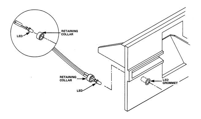
Figure 5-12 Activity LED Assembly Retaining Collar and Grommet
