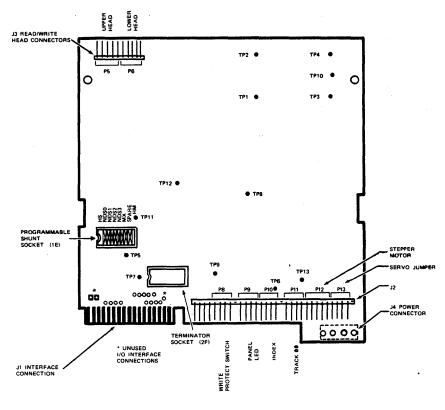
Figure 3-1 Logic PCBA
