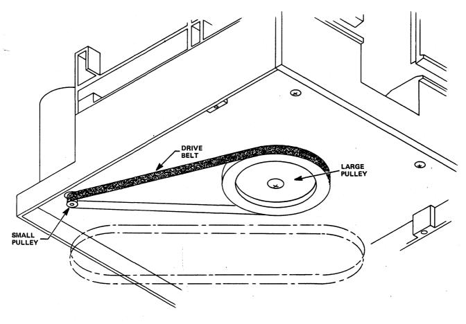
Figure 5-1 Drive Belt and Pulleys
