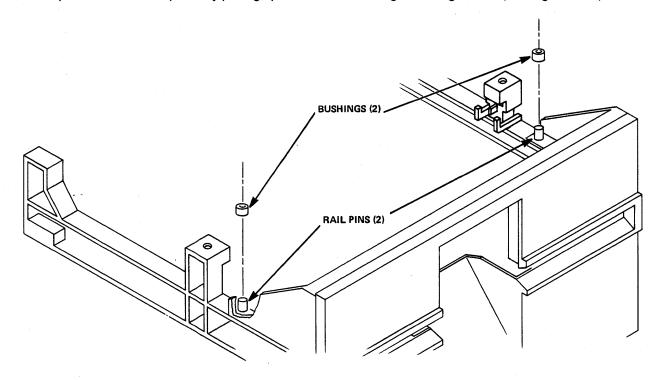
Figure 5-11 Front Panel Bushings
