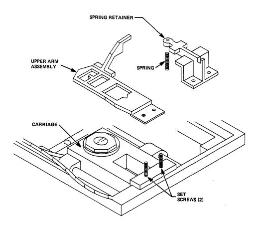
Figure 5-27 Upper Arm Assembly Parts
