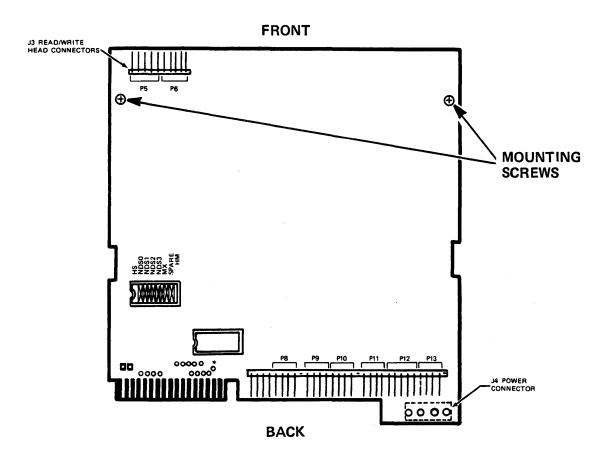
Figure 5-2 Logic PCBA Connectors and Mounting Screws
