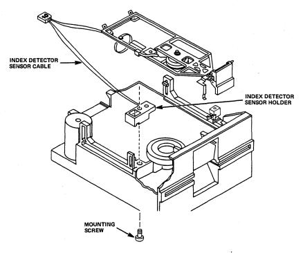
Figure 5-16 Index Detector Sensor Mounting Screw and Cable
