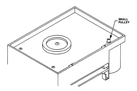
Figure 5-19 Drive Motor Assembly Pulley
