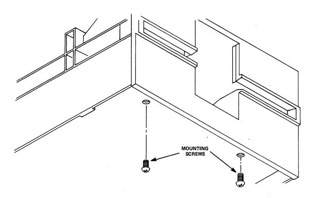
Figure 5-13 Front Panel Mounting Screws
