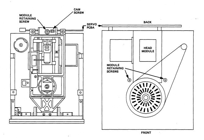
Figure 2-6 Head Module Retaining and Cam Screws
