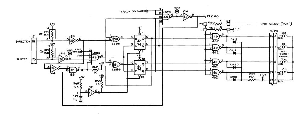
Figure 3-5 Direction and Step Lines Schematic Diagram
