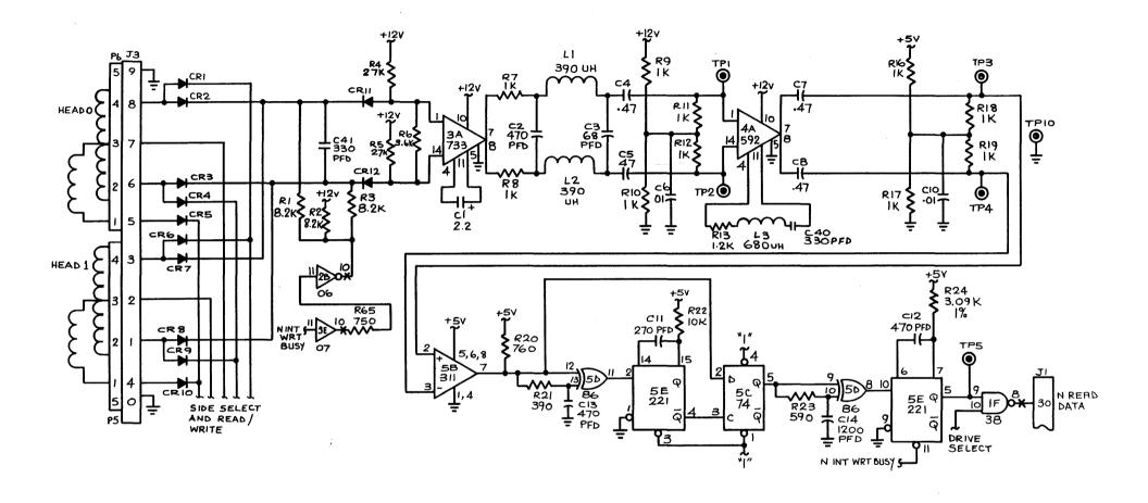
Figure 3-13 Read Data Schematic Diagram
