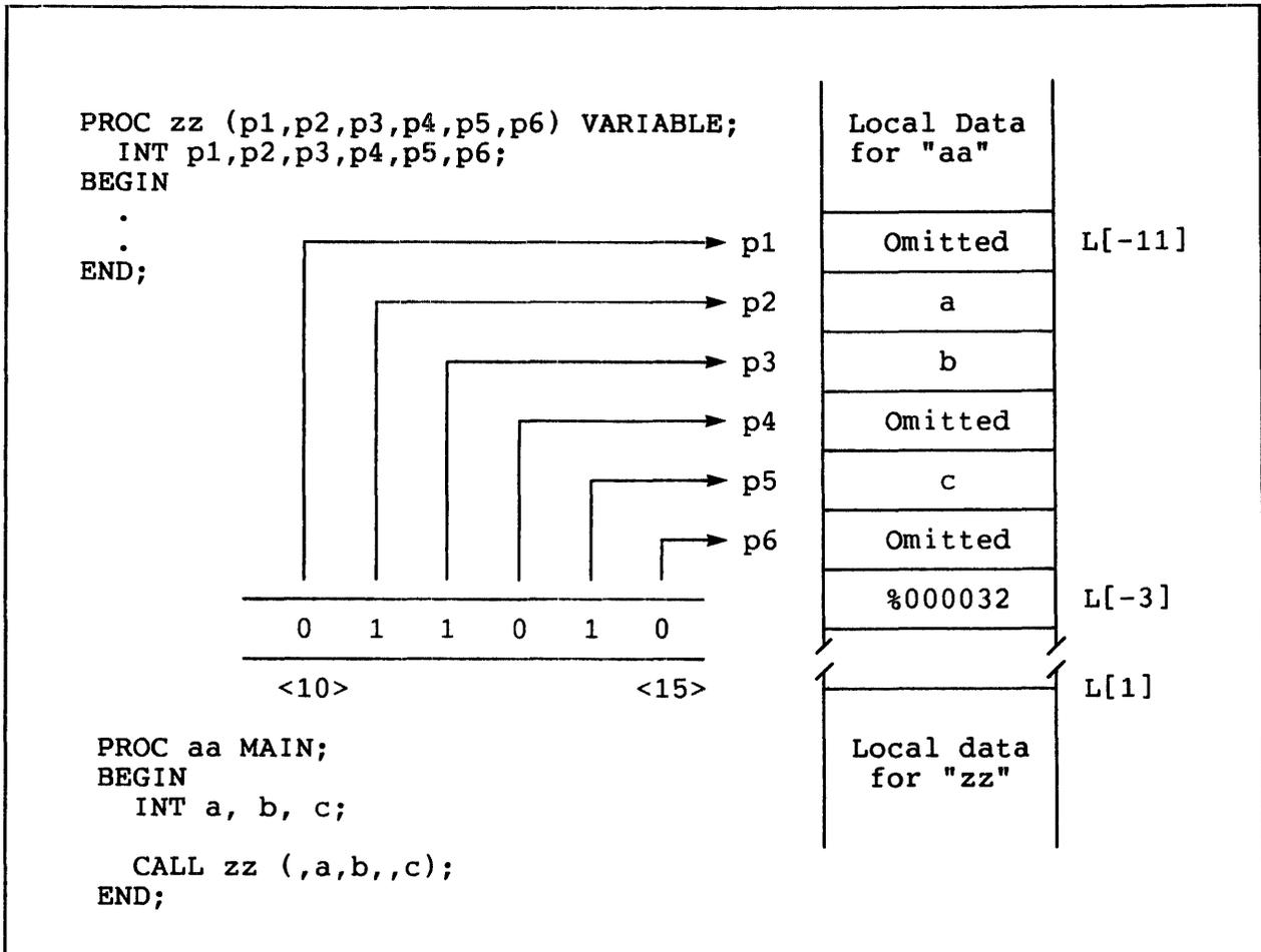
Figure 16-1. VARIABLE Single-Word Parameter Mask
