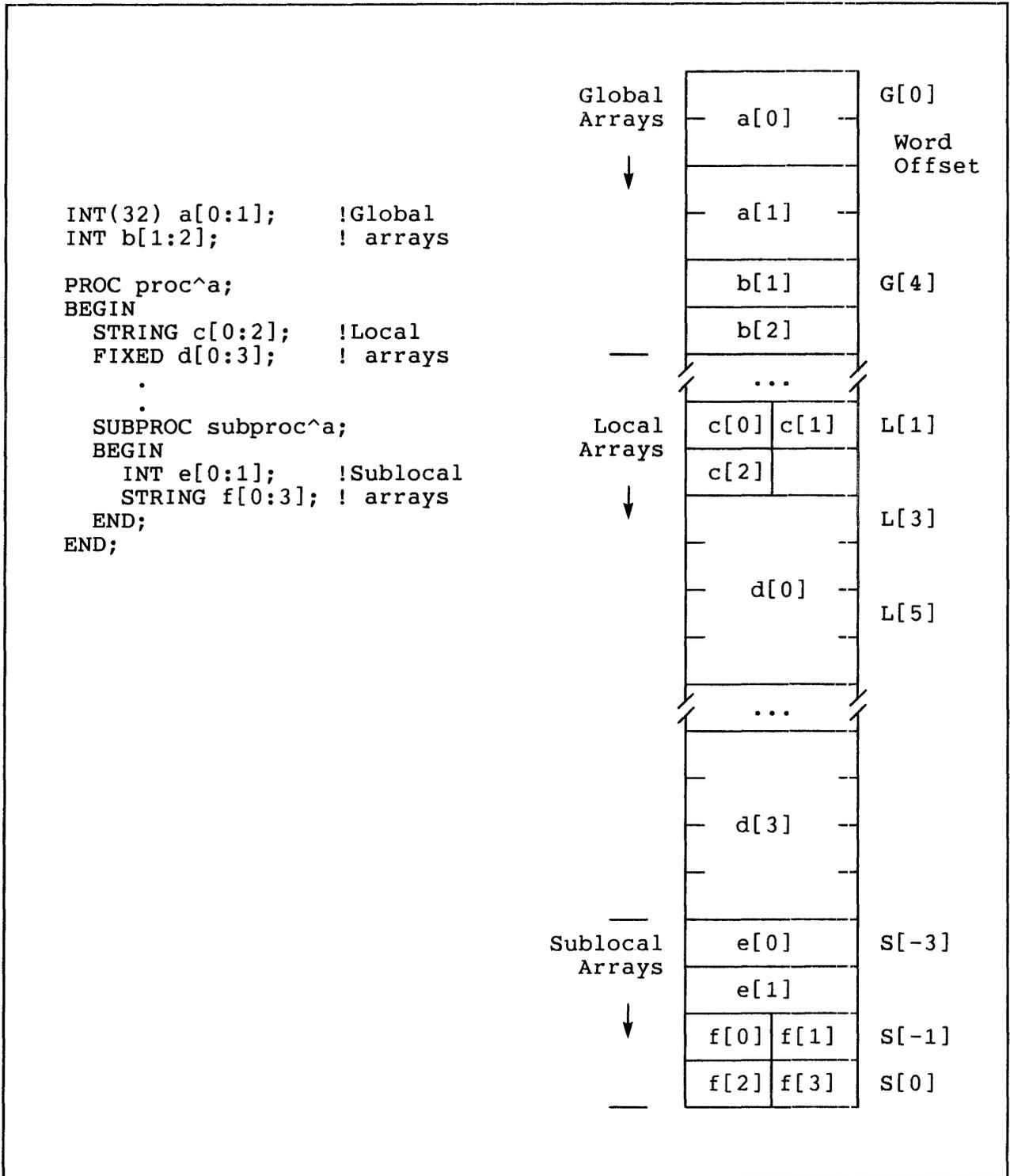
Figure 9-1. Storage Allocation for Direct Arrays
