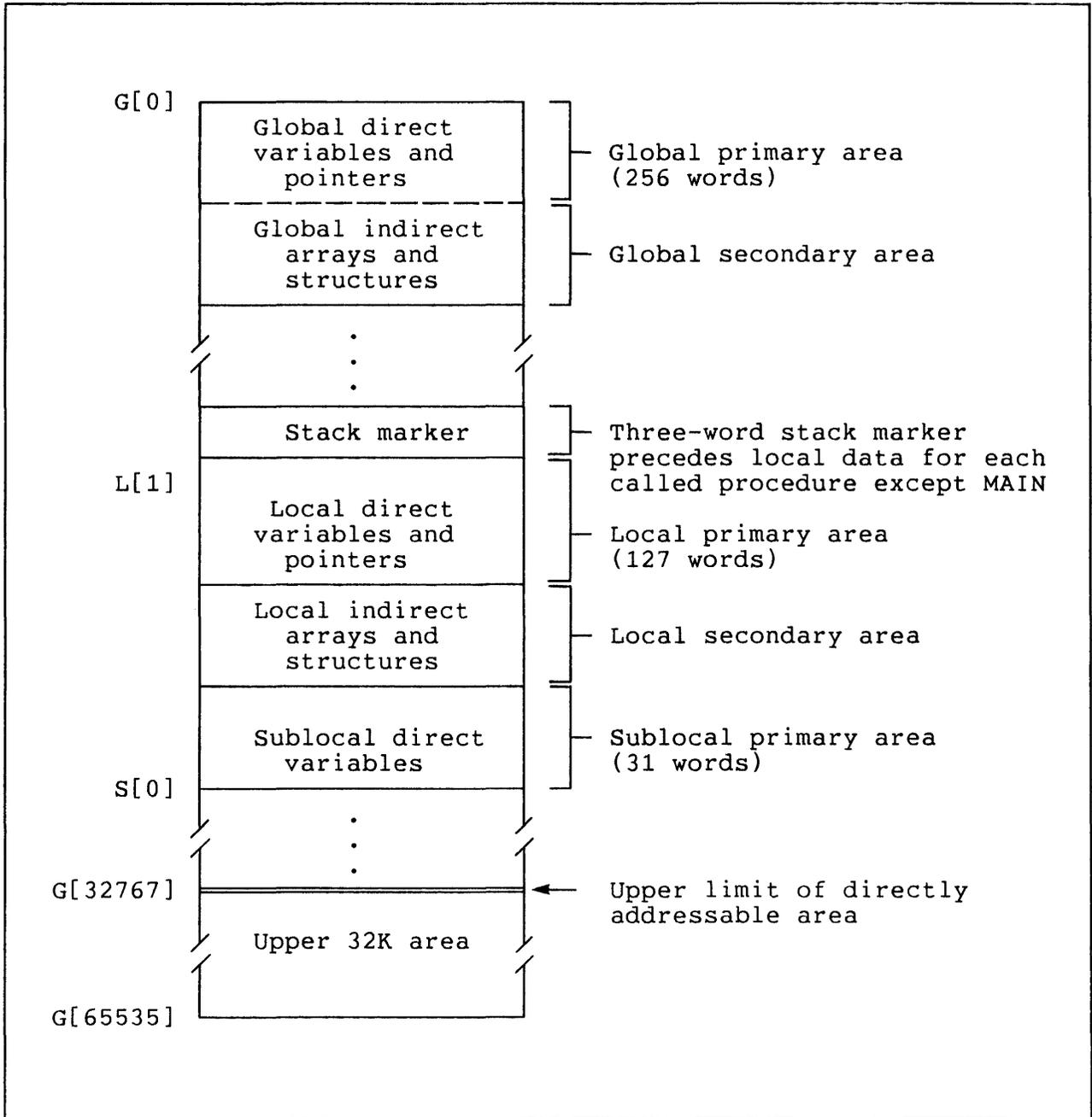
Figure 5-4. Primary and Secondary Storage in User Data Segment
