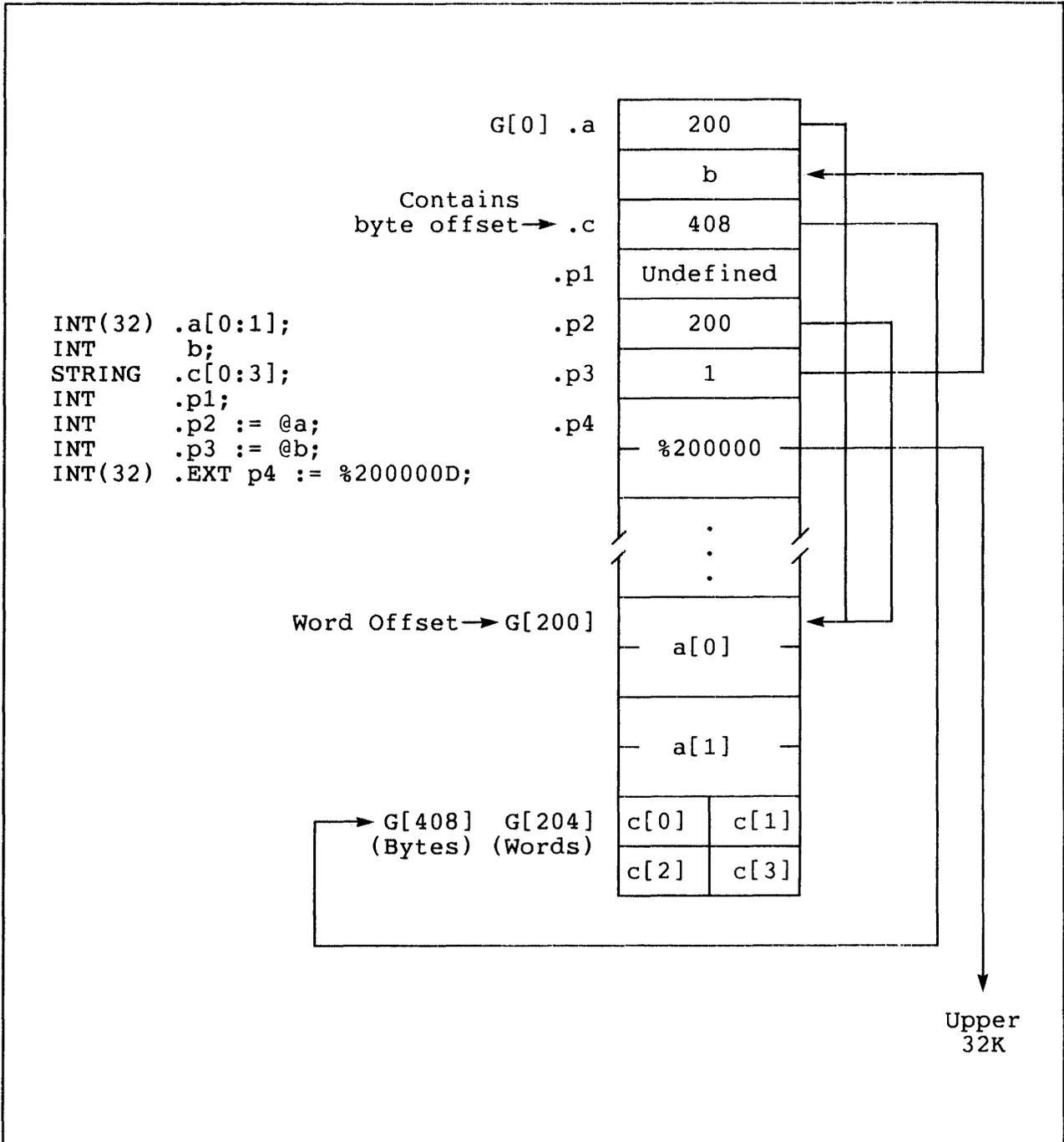
Figure 10-1. Pointer Storage Allocation
