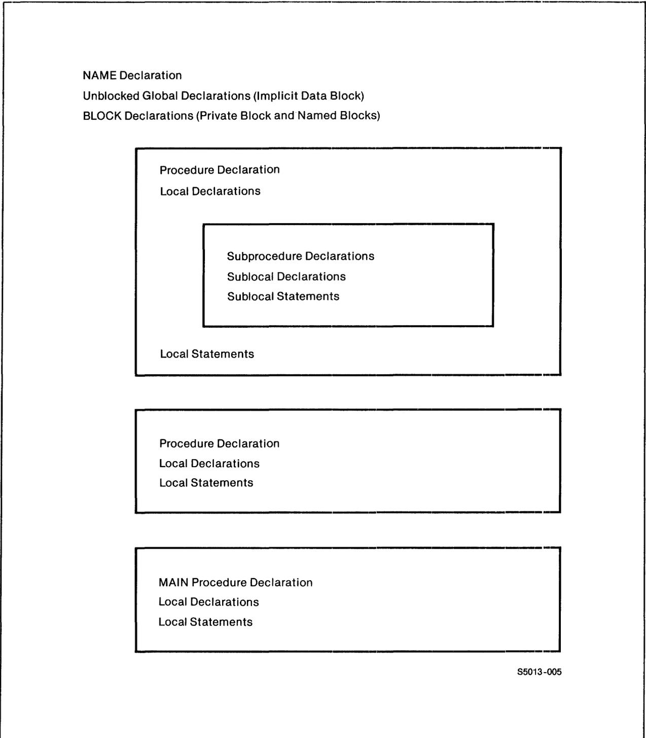
Figure 2-2. Structure of a Source Module
