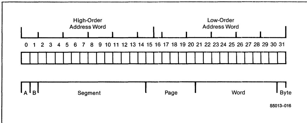
Figure A-1. Format of Extended Pointer
