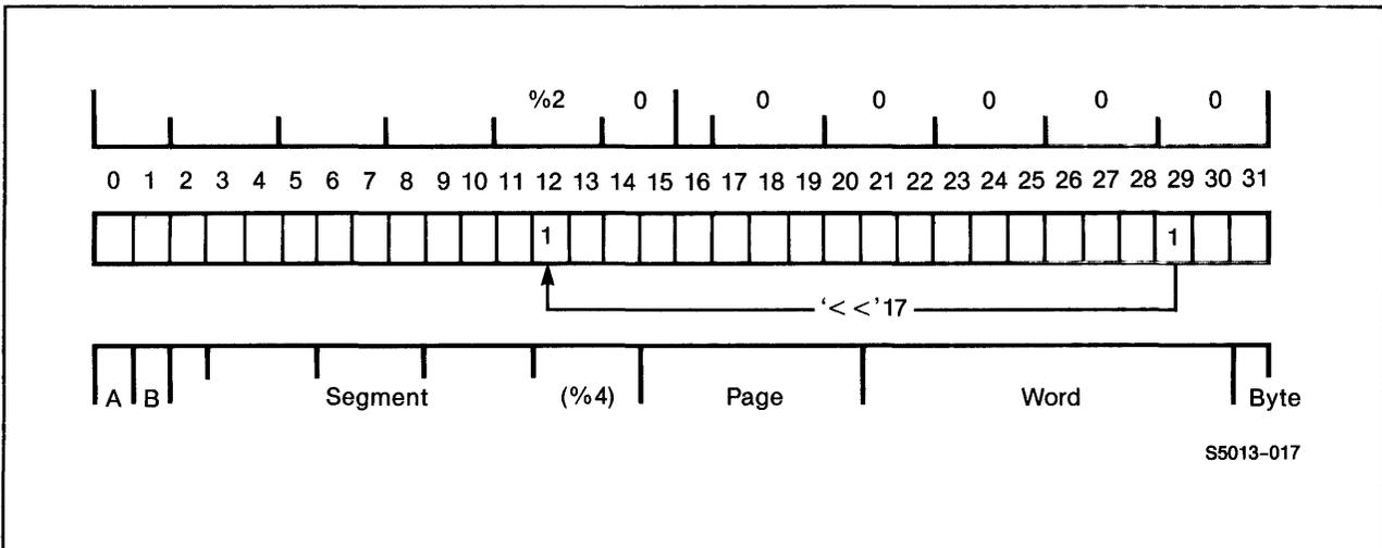
Figure A-2. Format of Extended Segment Base Address
