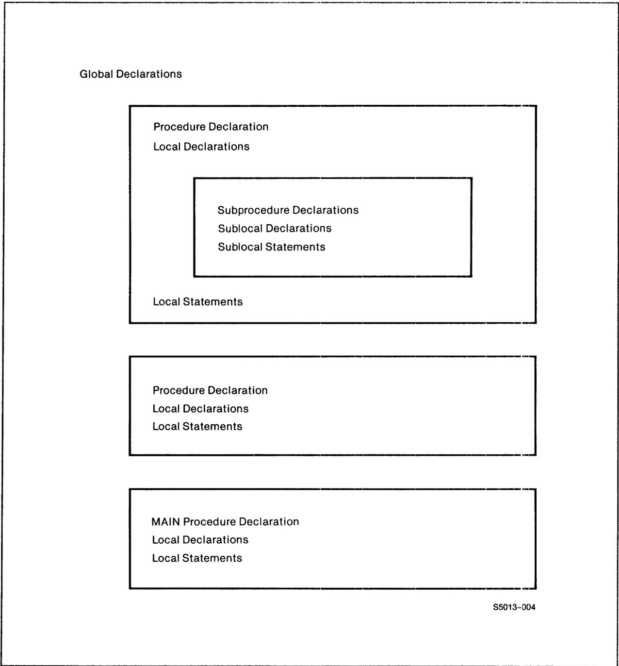
Figure 2-1. Structure of a Nonmodular Source Program
