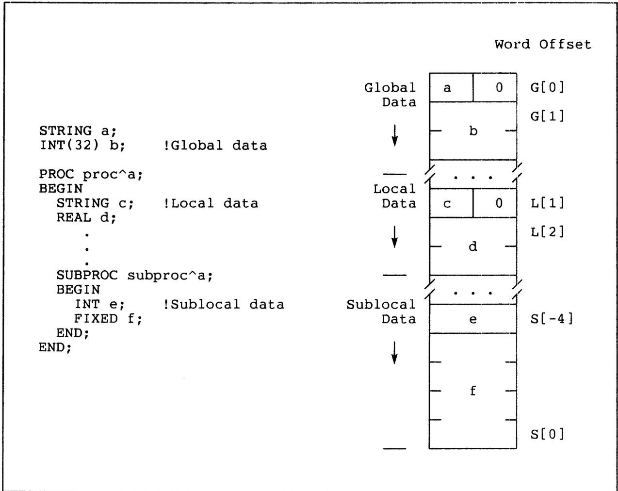
Figure 8-1. Storage Allocation for Simple Variables
