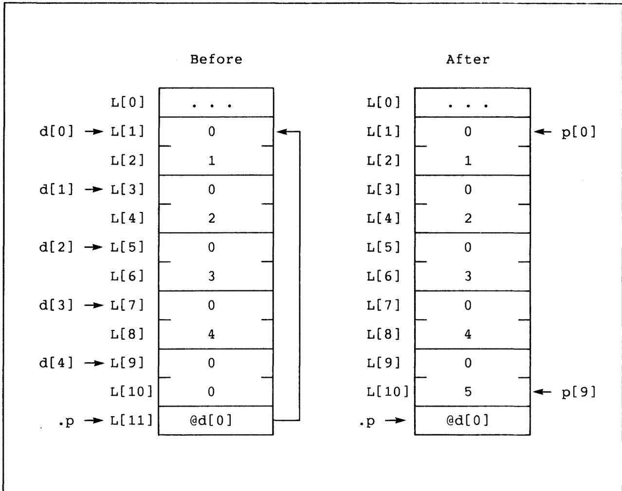
Figure 5-5. Indexing a Pointer
