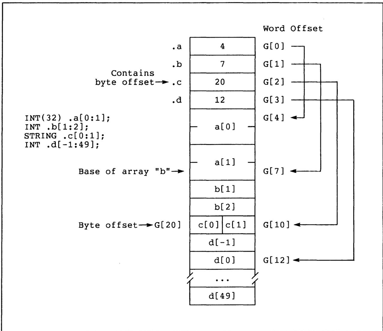
Figure 9-2. Storage Allocation for Indirect Arrays
