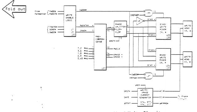
Simplified detail of Write Circuit.
