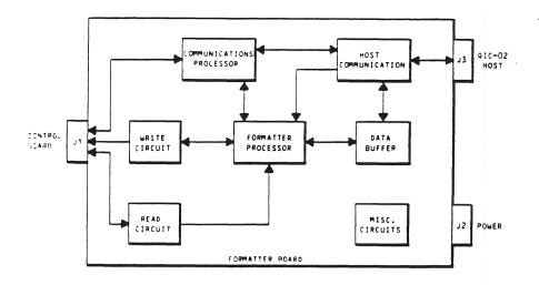
Overall block diagram of the Formatter board
