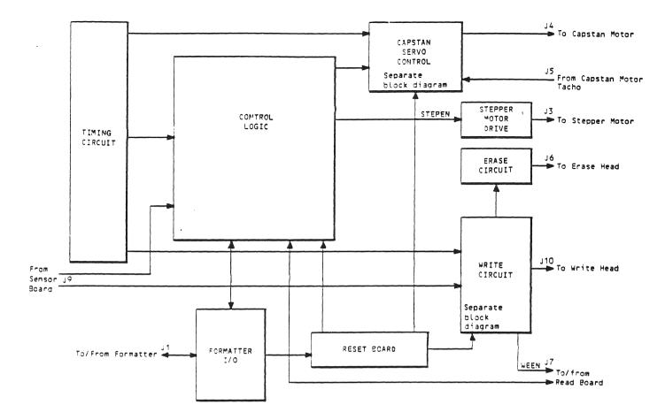
Block diagram of the Control board.
