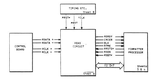
Signal connections between this circuit diagram sheet and other sheets of the Formatter circuit diagram.
