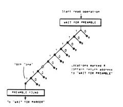
Path through the Read Sequencer PROM when searching for preamble in the DI bit stream.
