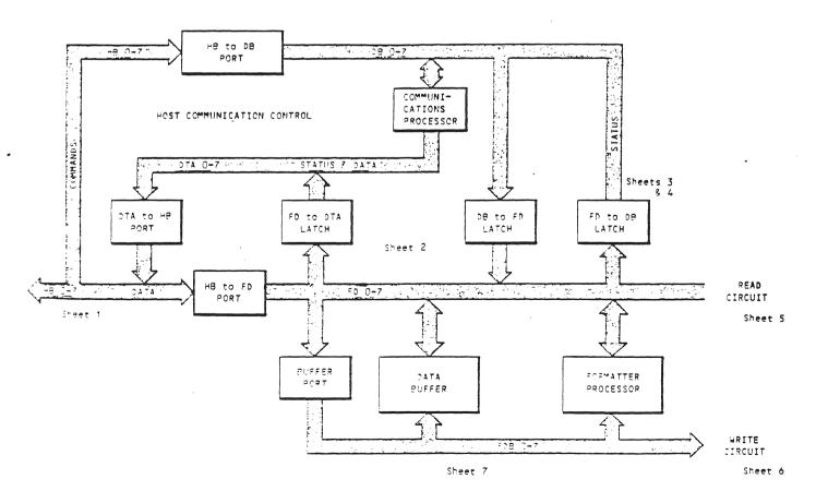
Block diagram of Formatter bus connections.
