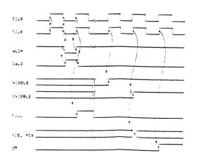
Write FIFO Controller timing.
