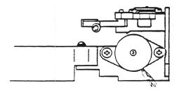
NOTE! Ensure correct orientation of the cable when replacing the motor. Check that the door moves freely when everything has been reassembled.
