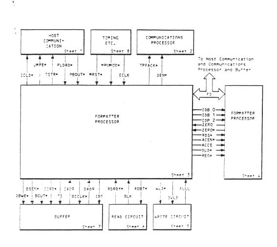
Signal connections between this circuit diagram sheet and other sheets of the Formatter circuit diagram.
