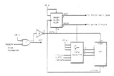
Simplified detail of Reset Circuit.
