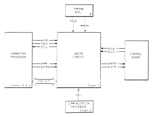
Signal connections between this circuit diagram sheet and other sheets of the Formatter circuit diagram.
