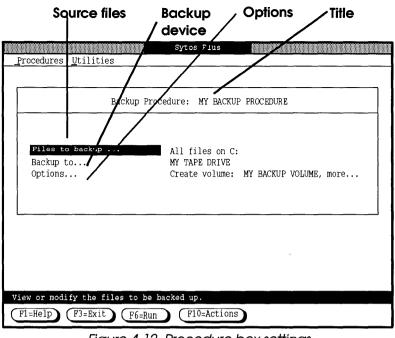
Figure 4-12 Procedure box settings
