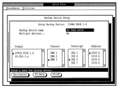
Figure 15-33 A tape system set up as a backup device
