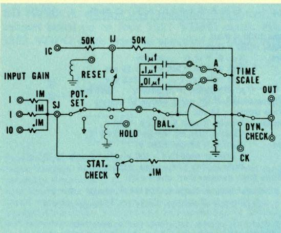
Feedback Capacitors (in oven)  $1 \mu\text{F}$ ,  $0.1 \mu\text{F}$ : Trimmable to better than 0.01%.
