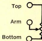
All other groups are 2-terminal with the bottom of the potentiometer internally grounded. The input voltage to the potentiometer is applied to the top terminal and the output is available at the arm terminal.
