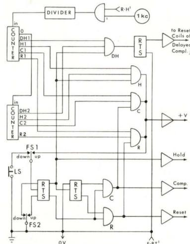
Figure 2. Iterative Operation Logic Control Circuit
