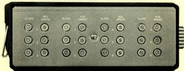
**Fixed Function Cards:** The 3351 VDFG (shown) and the high-resolution 3352 VDFG can be supplied with fixed functions, e.g., sine  $\pm 90^\circ$ , cosine  $\pm 90^\circ$ , Log  $|X|$  (range of X 1 to 100 volts). Each VDFG channel is terminated on the patchboard on Models 3321, 3322, and 3325.
