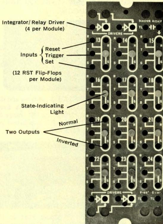
The flip-flop module contains 12 identical RST flip-flops and four relay drivers. Five patchboard terminals are available for each flip-flop, plus a state indicating lamp.
