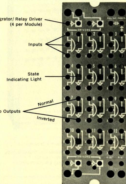
The Model 3327 contains 12 identical AND gates and four relay drivers. Each gate has three input terminals, two output terminals and a state indicating lamp.
