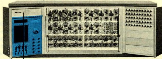
Function Generator Receptacle holds up to 15 Model 3351 (or 10 Model 3352 high resolution) V.D.F.G. plug-in cards.
