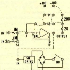
(CONNECTIONS SHOWN FOR COMPARATOR AMPLIFIER.)
