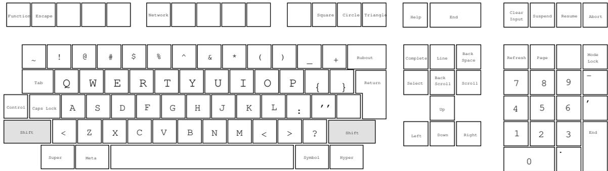
Figure 4. Open Genera Interpretation of the DEC LK401 AA Keyboard Using the Shift Key
