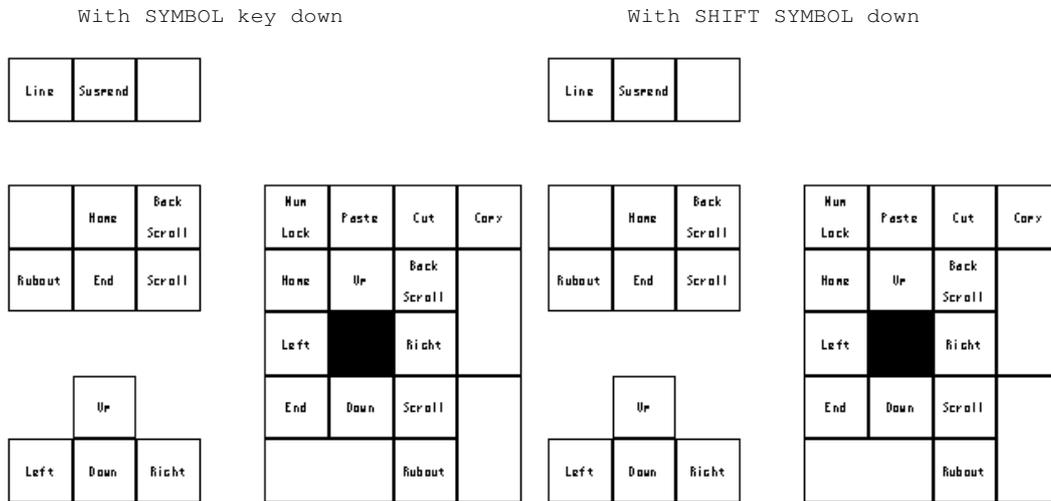
Figure 112. The with the Symbol Key as Modifier
