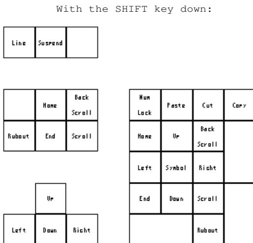
Figure 111. The Keypad with the Shift Key as Modifier
