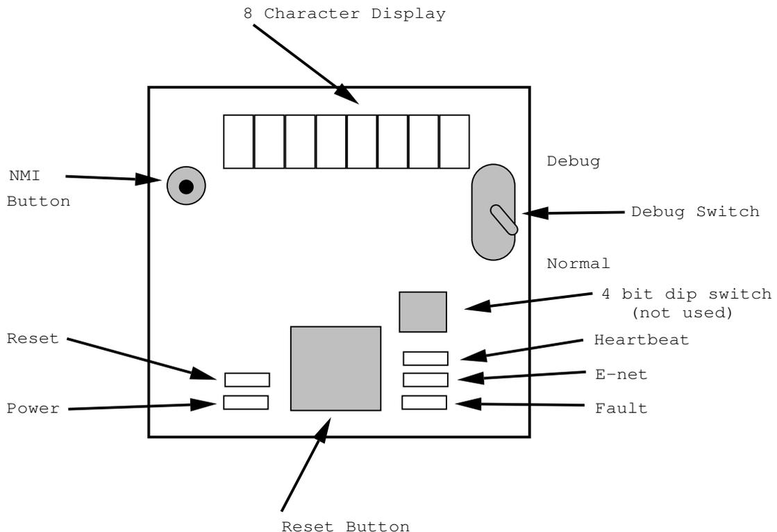
Figure 105. The Front Panel of the NXP1000
