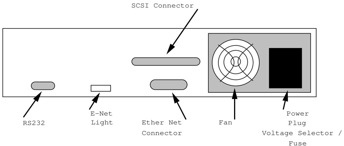
Figure 106. The Rear Panel of the NXP1000
