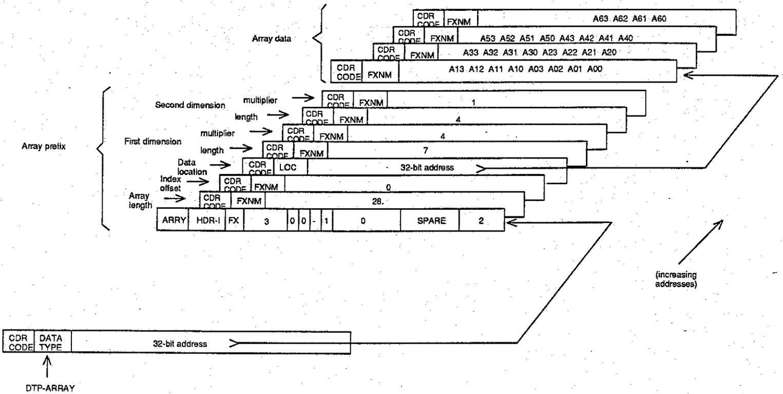
Figure 14. A two-dimensional array.
