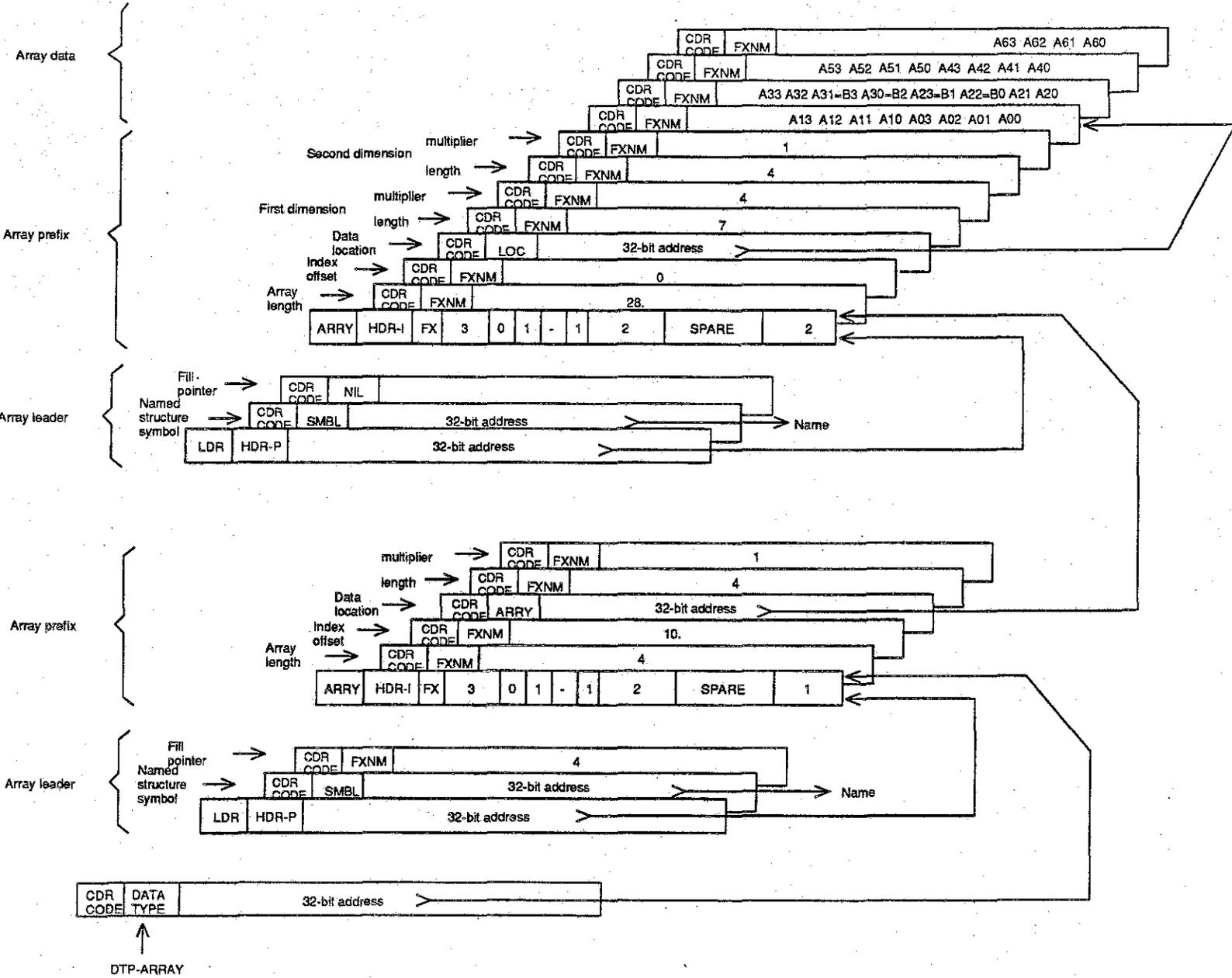
Figure 16. A one-dimensional array indirected to a two-dimensional array.
