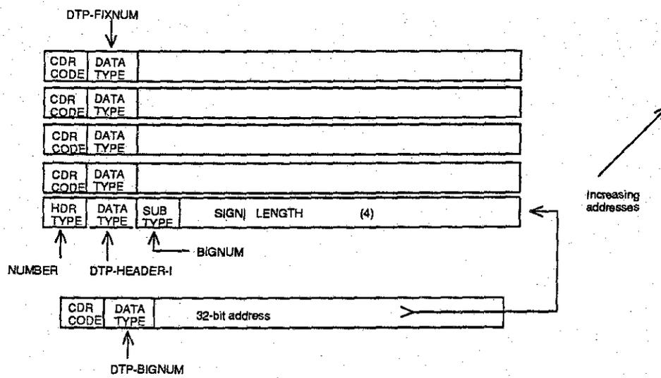
Figure 7. Structure of an object of type dtp-bignum
