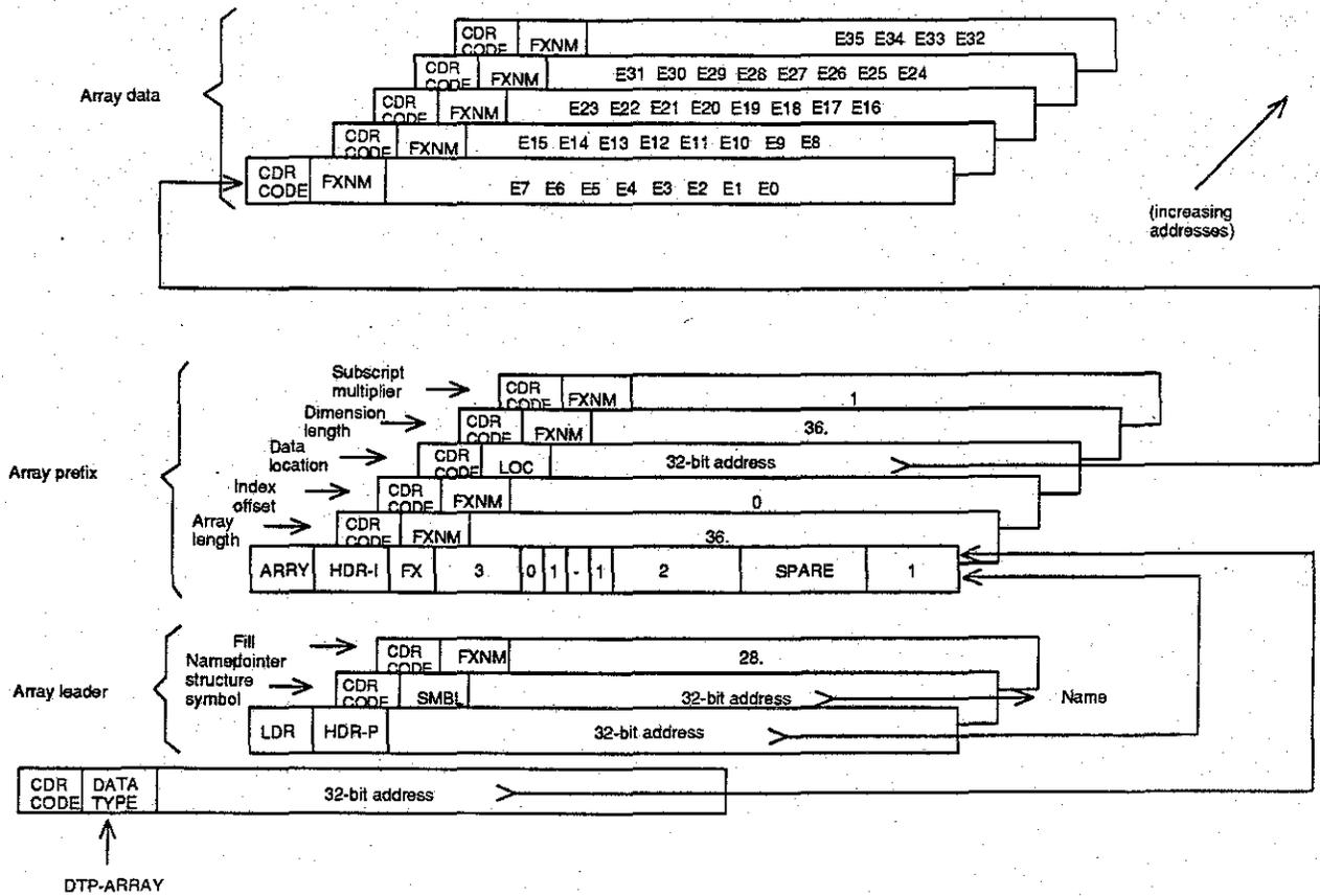
Figure 15. A simple displaced array.
