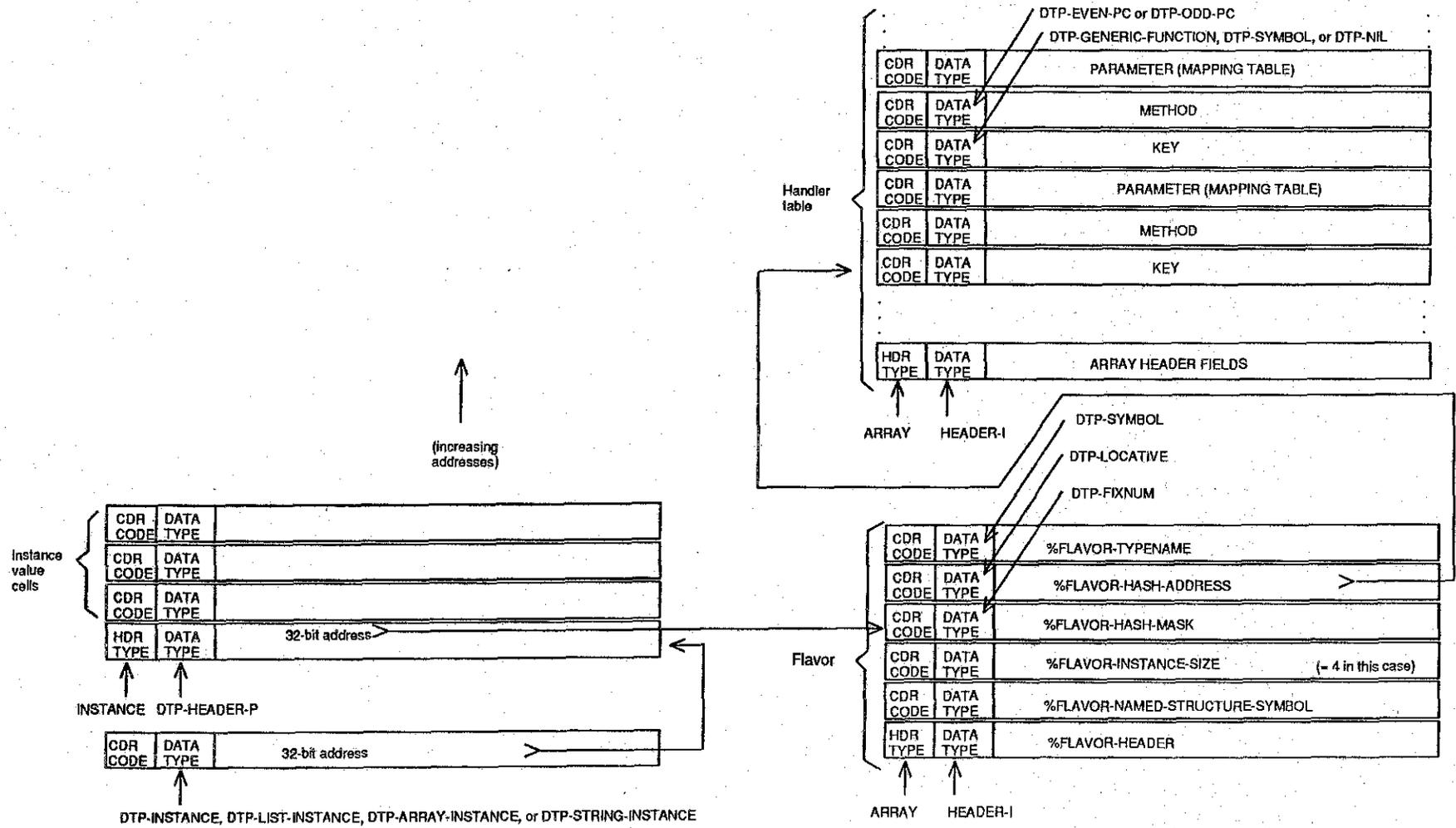
Figure 6. The structure of an instance.
