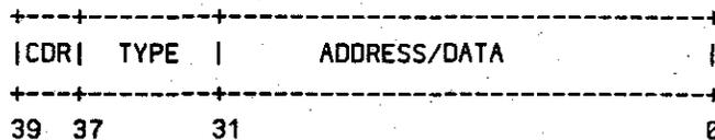
Words in actual physical memory may be more than 40 bits wide to allow for parity or ECC schemes. The architecture does not require the existence of parity or ECC nor does it specify any specific ECC algorithm. Such information and its implications are part of the documentation of each implementation and of the system units that support the implementation.
