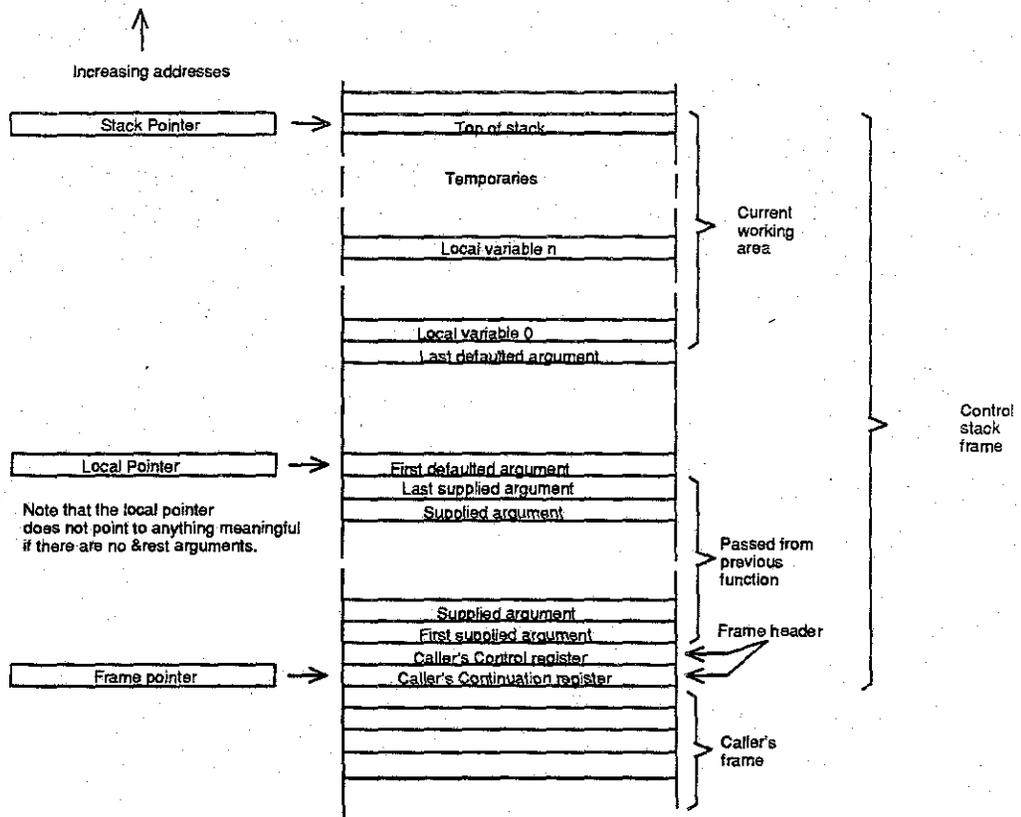
Figure 22. An I-machine control stack frame.
