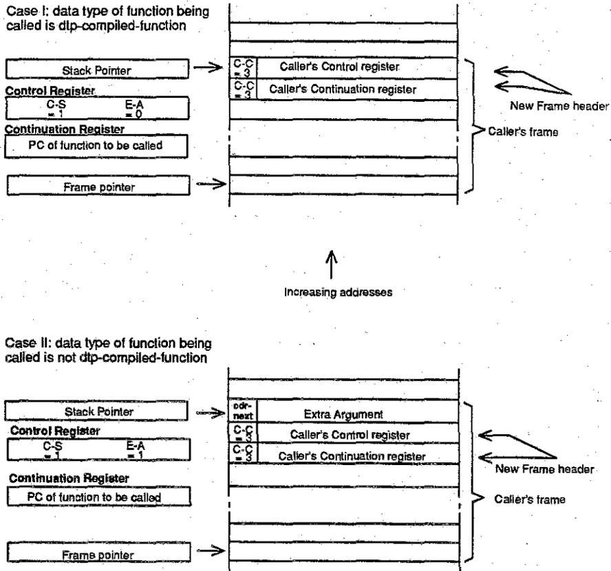
Figure 23. The stack at the end of a start-call instruction
