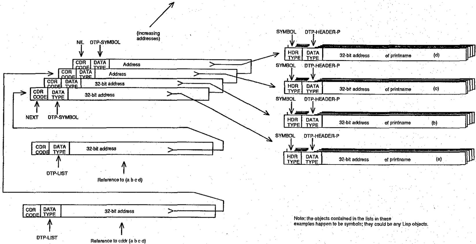
Figure 12. An object reference to the caddr of a list.
