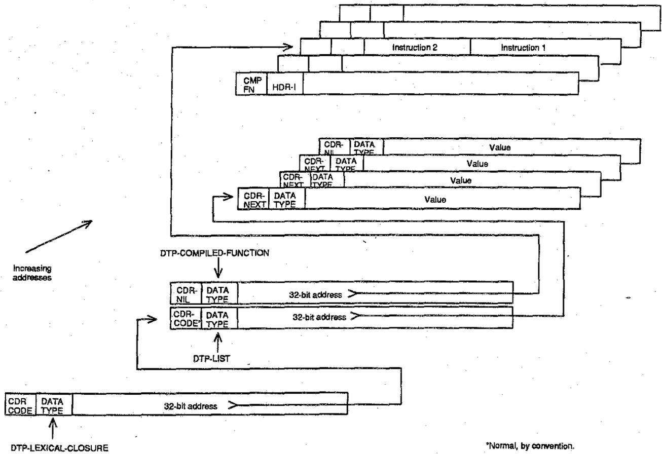
Figure 18. The structure of a lexical closure.
