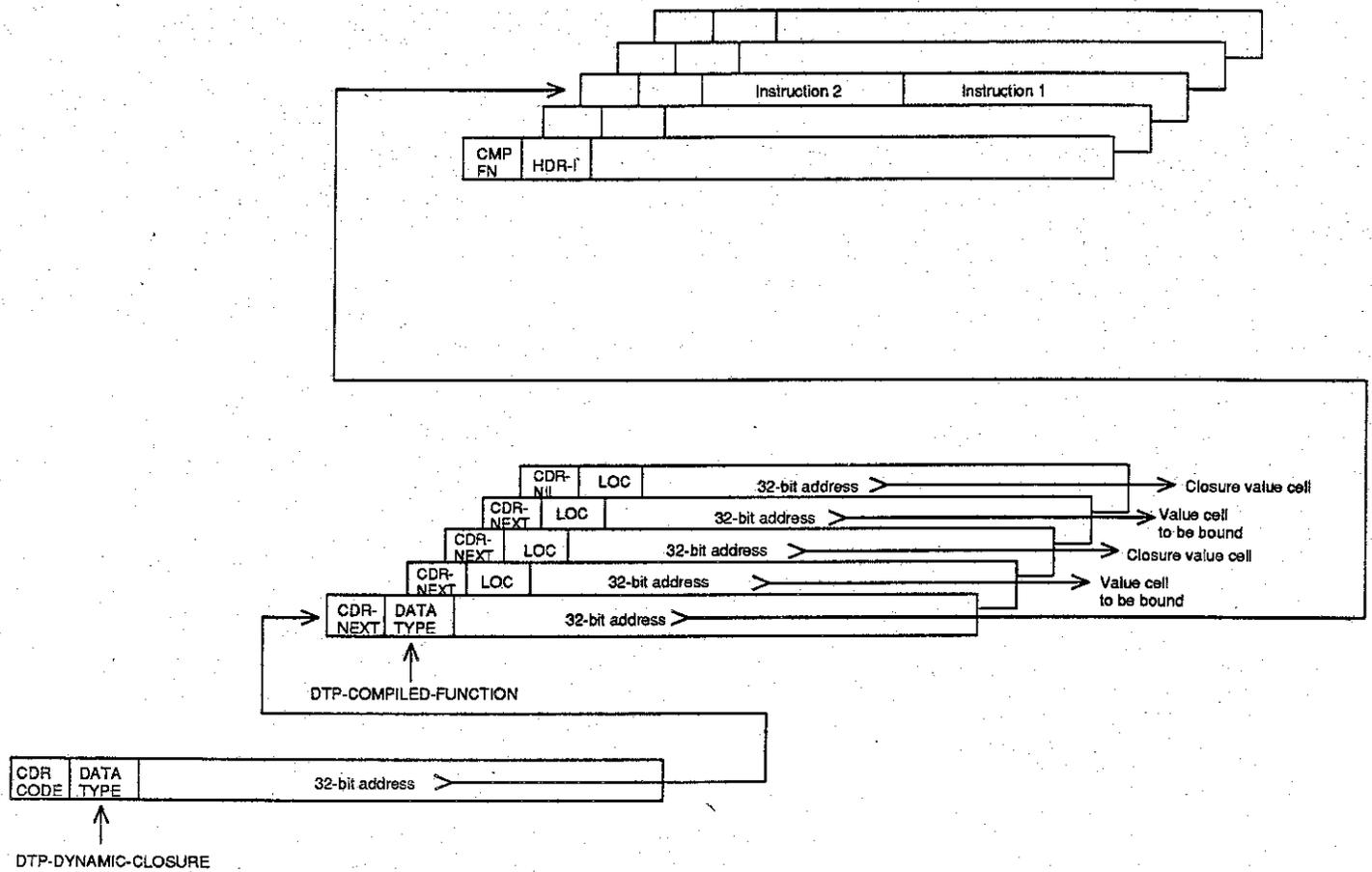
Figure 19. The structure of a dynamic closure.
