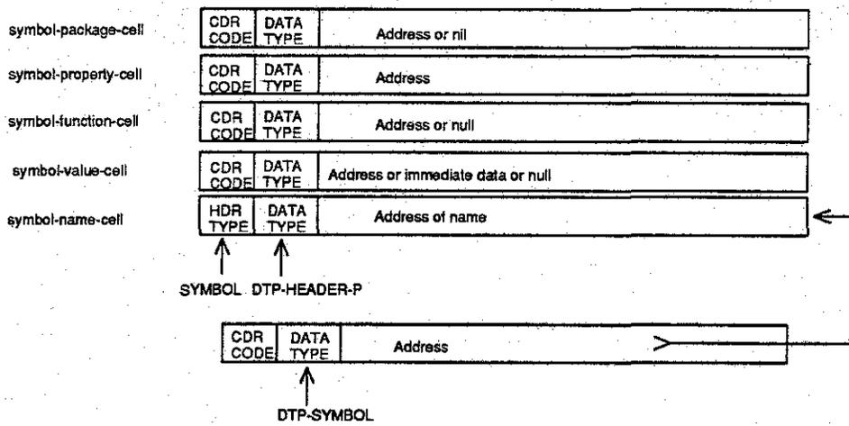
Figure 5. Structure of a symbol object.
