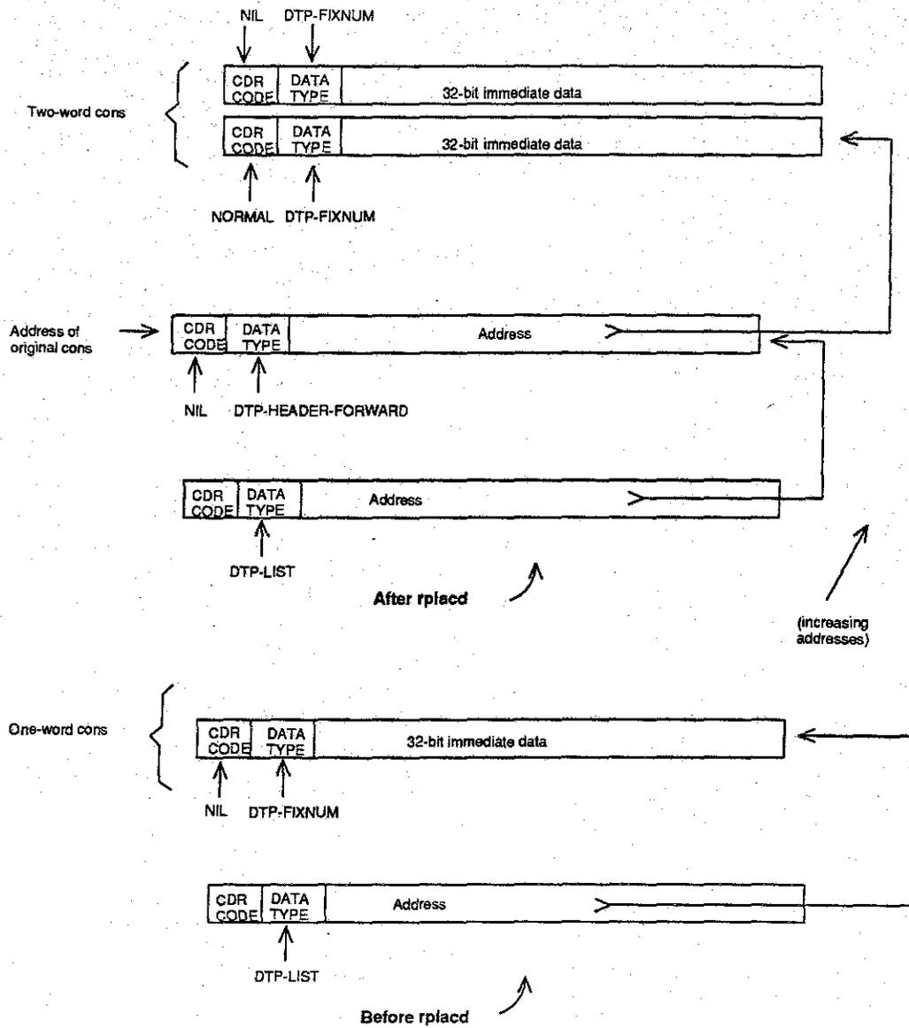
Figure 4. Use of forwarding pointers to expand a cons.
