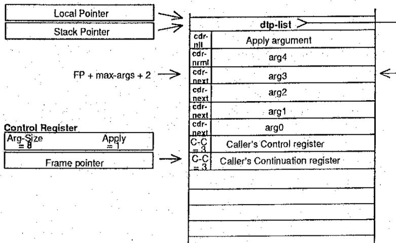
Figure 26. The push-apply-args operation
