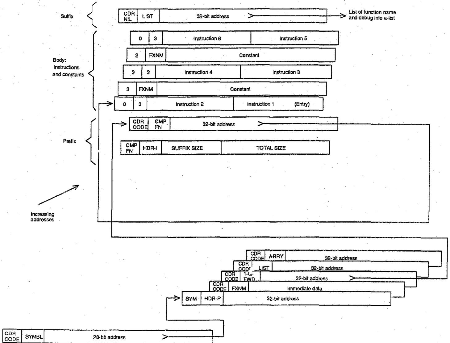
Figure 17. The structure of a compiled function.
