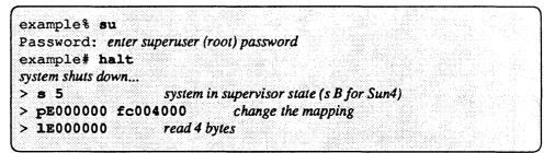
The p command establishes the mapping of virtual addresses to physical ones. The physical address, however, should be converted into *PTE* format. The conversion can be done as follows:
