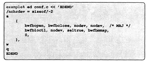
This file is really a table of all the device drivers. The functions of each driver are collected into an array called cdevsw (character device switch table). Each element of this array represents one device driver and the sequence number is the *major number* of the device.
