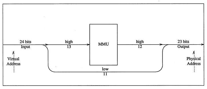
Figure 5-2 Sun-3 Address Mapping
