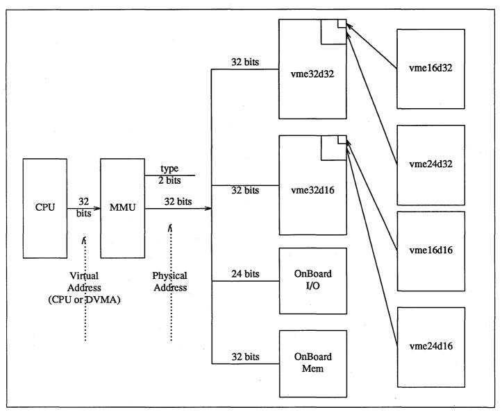
Figure 2-5 Sun-4 VMEbus Address Spaces
