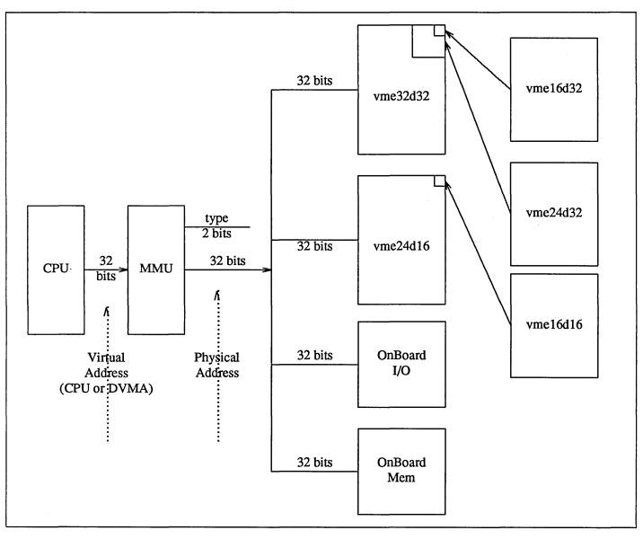
Figure 2-4 Sun-3x VMEbus Address Spaces
