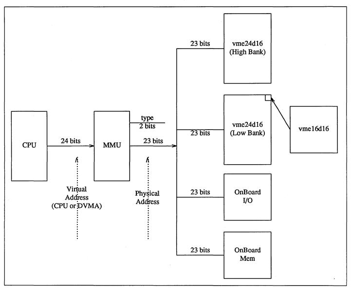
Figure 2-2 Sun-2 VMEbus Address Spaces
