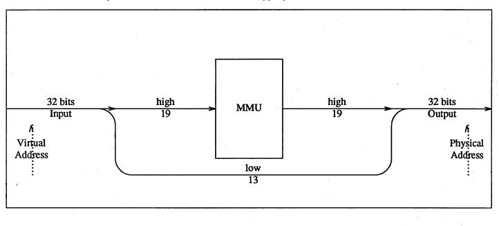
Figure 5-3 Sun-3x/Sun-4 Address Mapping
