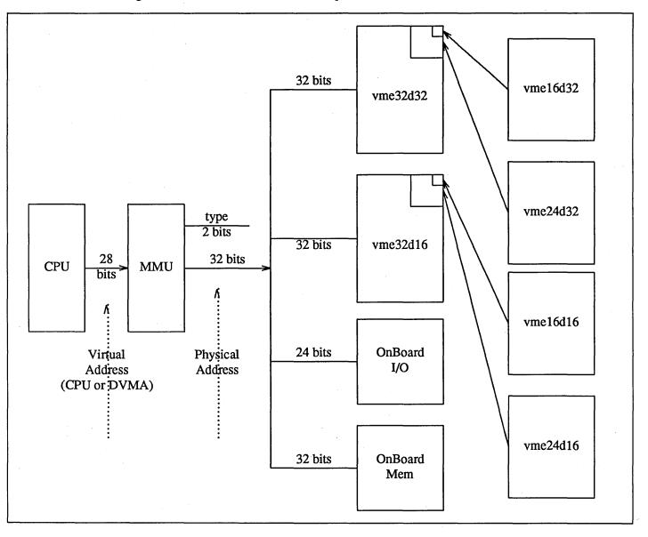
Figure 2-3 Sun-3 VMEbus Address Spaces
