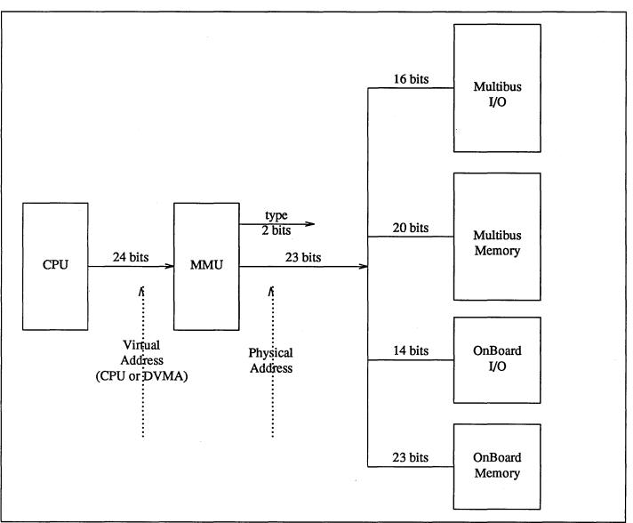
Figure 2-1 Sun-2 Multibus Address Spaces
