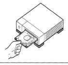
• Press the eject button on the front panel of the CD-ROM drive (a tray will emerge if you have this type of caddy).
