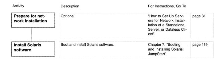
Figure 2-2 Task Map for JumpStart Installations
