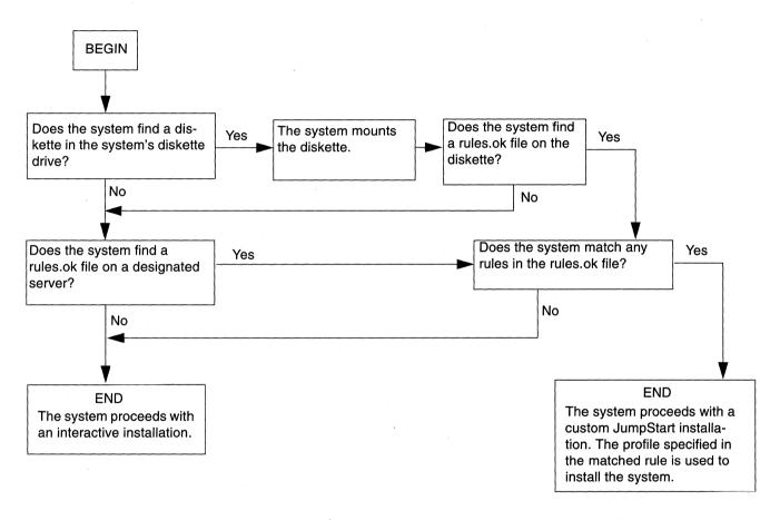
Figure 4-1 What Happens During a Custom JumpStart Installation
