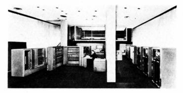
b. Tube-Type Machine: IBM 704 (Courtesy IBM Corporation)
