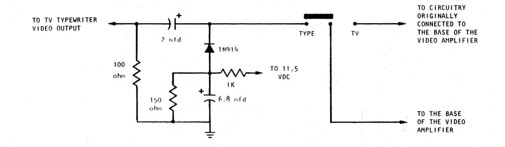
Figure 2 - Video Input Modification for Motorola K9TS-460Q Television
