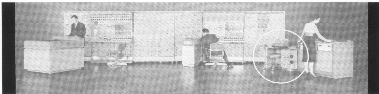
The ADIOS, circled in the photo, is an "Automatic Digital Input-Output System" produced for Electronic Associates, Inc., Long Branch, New Jersey, for integration into their PACE 231R analog computer line. A comparable Satellite Console which also uses a Soroban Computeriter, Keyboard, and Tape Reader is pictured on page 63. The ADIOS not only permits automatic tabulation of test data, but also permits potentiometer ratios to be automatically set from data prerecorded in punched tape.
