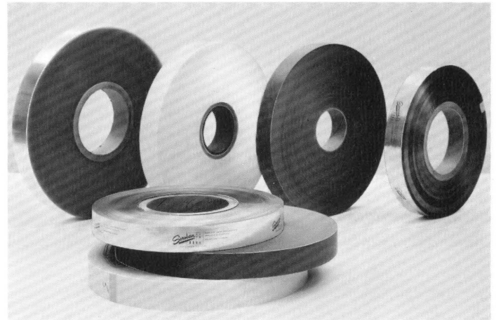
MYLAR AND PAPER TAPES — Both 0.004 inch thick yellow lubricated paper and 0.0025 inch thick Mylar-Aluminum-Mylar laminated tape, 10-25-10, are maintained in inventory in nominal 800 foot rolls, 11/16", 7/8", 1", and 2 1/8" in width.
