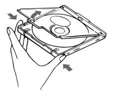
**2** Set a disc, with its label upward, in the caddy.
