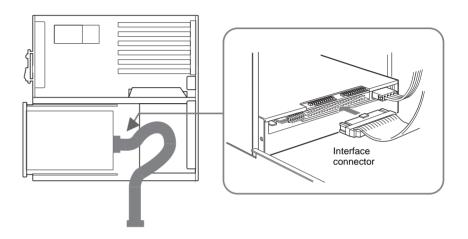
**2** Attach the other end of the cable to the host adapter.
