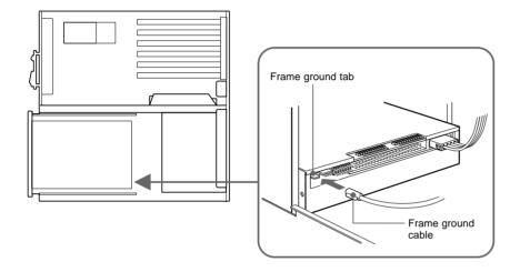
The frame ground cable recommended has a AMP 1-480435-0 housing and 170203-2 or 60711-1 contacts.
