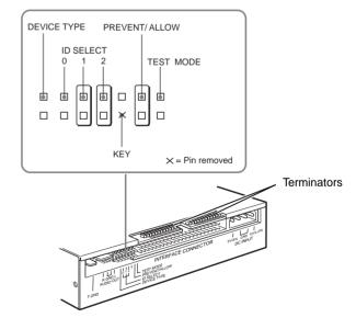
Remove the jumper to set to OFF, and install the jumper to set to ON. The recommended jumper is AMP\* Shunts (14227-1), JAE\*\* Short Socket (PS-2SH4-1) or equivalent.
