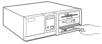
The drive begins reading the Table of Contents (TOC) data. The busy indicator lights amber while the TOC data is being read.
