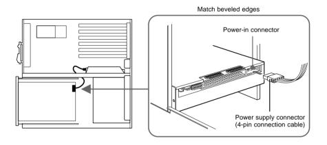
The power supply connector recommended has Molex 8980-3 contacts and a Molex 8981-04P housing.
