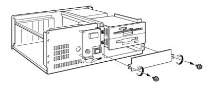
**2** If mounting rails are necessary, attach them to the drive unit in the same way as the ones on your floppy disk drive and slide the drive unit into the bottom half-height space. Otherwise screw the drive unit in place.
