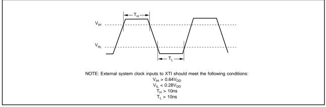
FIGURE 8. Operation Instruction For System Clock.
