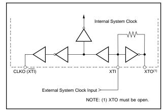
FIGURE 10. Oscillator Circuit Connection Diagram. External system clock.
