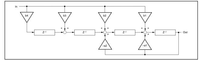
FIGURE 2. Block Diagram of the Hf(z).
