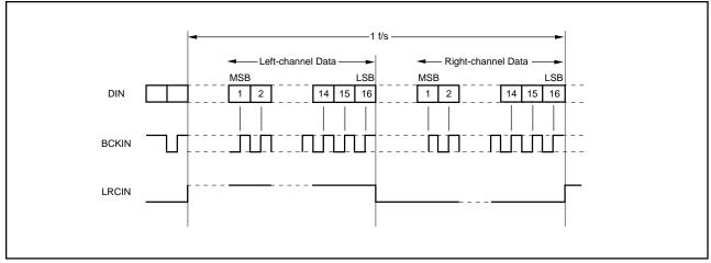
FIGURE 5. Data Input Timing, 16-Bit.
