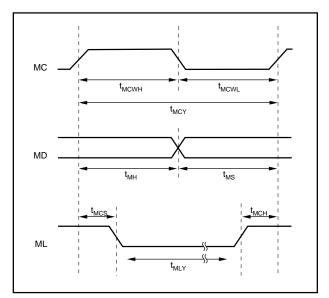
FIGURE 7. Serial Mode Control Timing.
