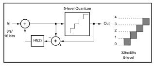
FIGURE 1. Block Diagram of 5-Level Delta-Sigma Quantizer.
