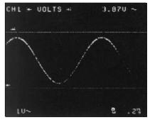
NOTES: (1) Measured at V<sub>out</sub> Pin (Pin 13 or 16). (2) The PCM1715 has internal analog low pass filter to reduce high frequency noise-shaped spectrum. Application of the PCM1715 requires external post analog low pass filter which has 2nd-Order or 3rd-Order attenuation performance to get low noise analog output.
