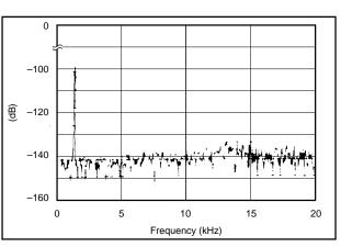
FIGURE 4. Quantization Noise Spectrum (384fs).
