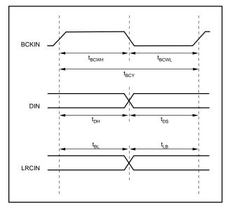
FIGURE 6. Data Input Timing.
