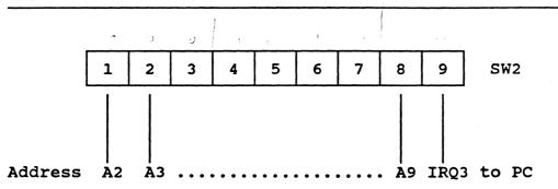
If the switch setting is depressed on the ON side then it indicates 'on' or a logic '1'. Similarly if the switch setting is depressed on the OFF side then it indicates 'off' or a logic '0'.
