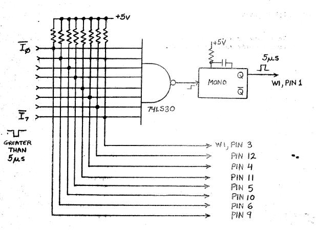
This two IC circuit will set the status flag of the input port and place the interrupt code (10 thru 17) into U30. No more interrupts will be generated until the one low going interrupt line is back to a logic one. The interrupt lines can be normally-open momentary switches for special console features.
