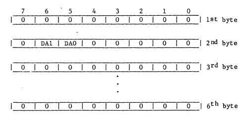
The TEST READY command selects the drive which is addressed by the DAO-1 bits and tests for ready. The returned status bytes will indicate an error if the drive is not ready.
