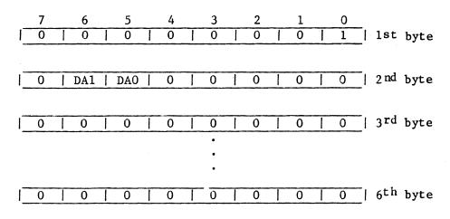
The RECAL command positions the heads of the addressed drive at cylinder zero. The normal two bytes of status are returned at command completion.
