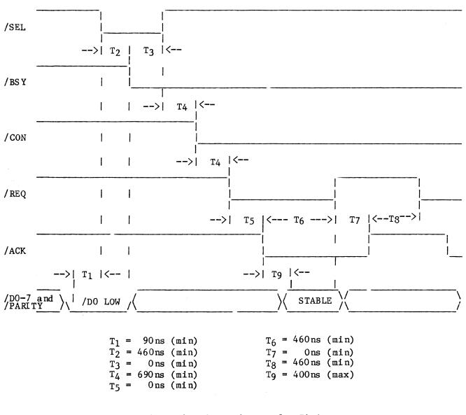
Figure 1. Command Transfer Timing
