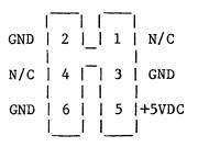
Figure 6. FWD5000 PC Board Power Connector
