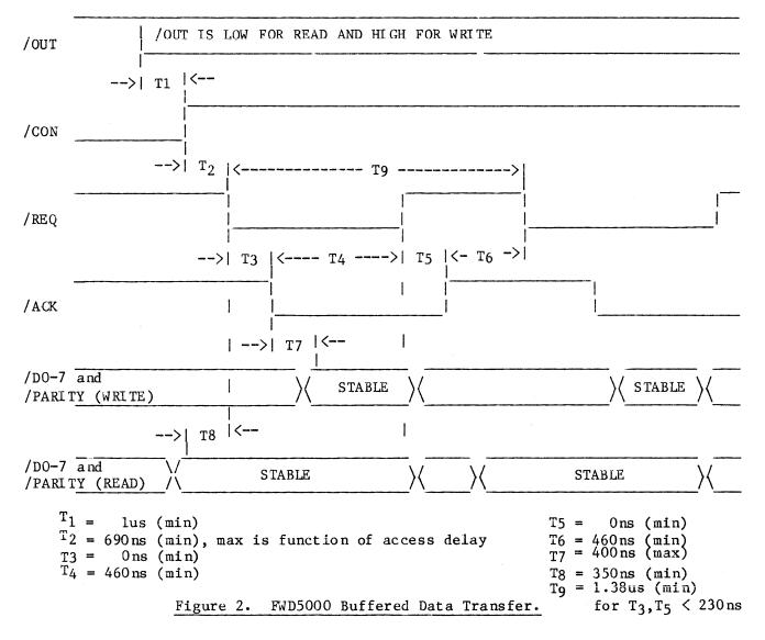
Figure 3 shows the timing for buffered reading and buffered writing when the fast handshake is enabled (FH bit set in command byte). Note that the host memory access is performed during T3 between the assertion of REQ by the controller and the assertion of ACK by the host. With the SA1403D compatible handshake shown in Figure 2, the amount of time allowed for the user memory access is:
