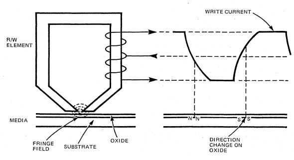
FIGURE 12 RECORDING CURRENT AND FLUX
