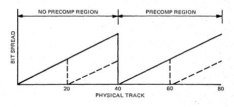
FIGURE 18 WRITE PRECOMPENSATION
