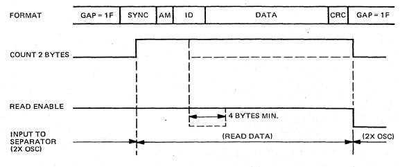
FIGURE 20 ADDRESS MARK DETECTION TIMING DIAGRAM
