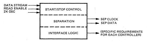
FIGURE 19 SEPARATOR FUNCTIONAL BLOCK DIAGRAM
