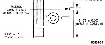
FIGURE 8-3. WRITE PROTECT NOTCH SPECIFICATIONS
