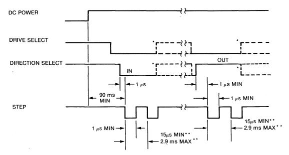
\*After the last step pulse has been issued the drive may be deselected. The drive ignores any change to the DIRECTION SELECT line when no further step pulses are received. This frees the controller to issue instructions to other drives while the first drive completes the step commands stored in the buffer.
