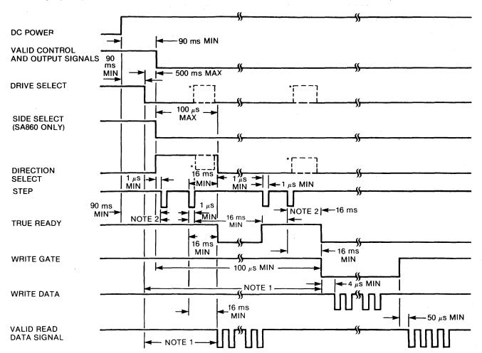
NOTE 1: 165 ms minimum delay must be introduced after DRIVE SELECT to allow time for the dc motor to reach 360 rpm or the optional TRUE READY line must be monitored.
