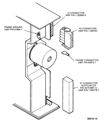
FIGURE 3-1. INTERFACE CONNECTORS - PHYSICAL LOCATIONS
