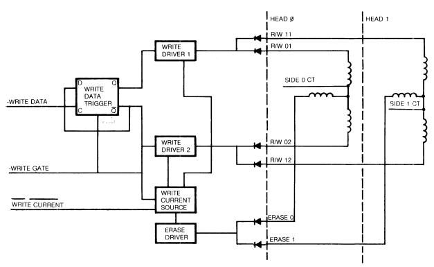
FIGURE 32. WRITE CIRCUIT FUNCTIONAL DIAGRAM
