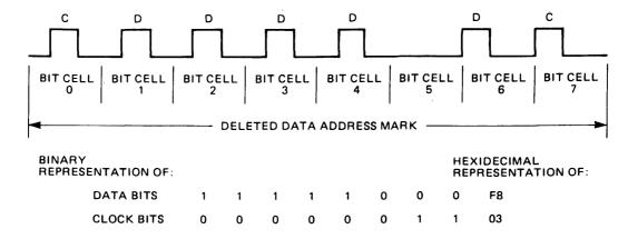
FIGURE 18. MFM DELETED DATA ADDRESS MARK
