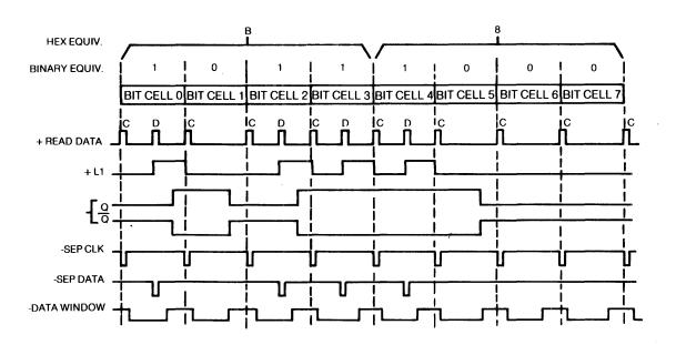
FIGURE 34. DATA SEPARATION TIMING DIAGRAM
