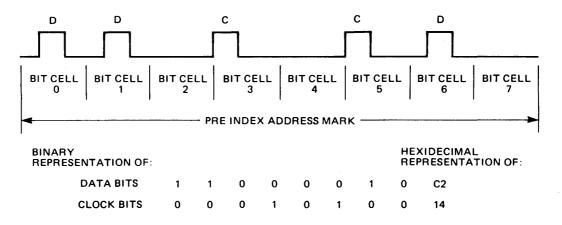
FIGURE 19. MFM INDEX PRE ADDRESS MARK
