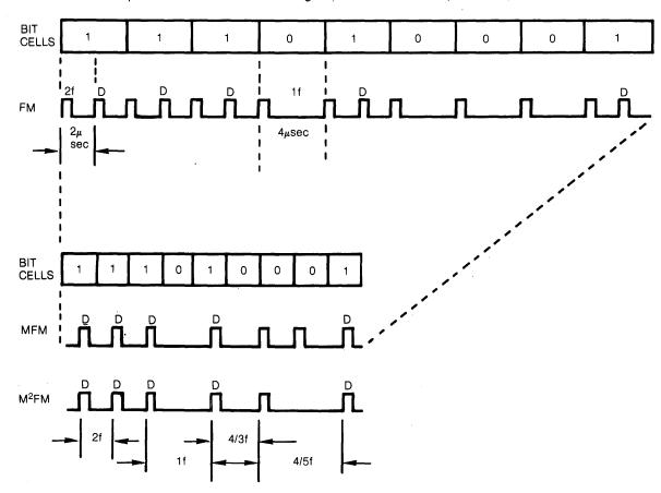
FIGURE 7. FM. MFM AND M2FM ENCODING
