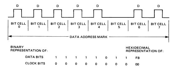
FIGURE 17. MFM DATA ADDRESS MARK
