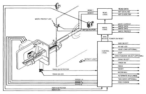
FIGURE 1. SA850/851 FUNCTIONAL DIAGRAM
