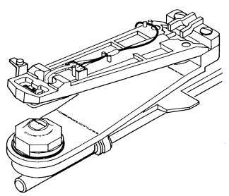
FIGURE 2. BI-COMPLIANT READ/WRITE HEAD
