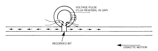
FIGURE 29. READING A BIT
