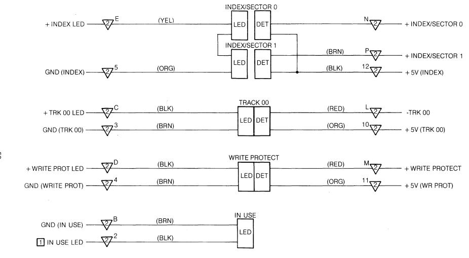
**NOTES:**[1] GND WHEN INACTIVE AND +1.5VDC WHEN ACTIVE.
