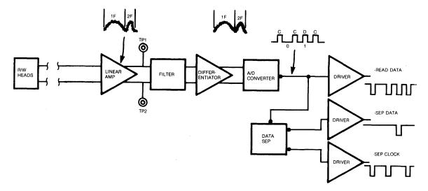
FIGURE 33. READ CIRCUIT FUNCTIONAL DIAGRAM
