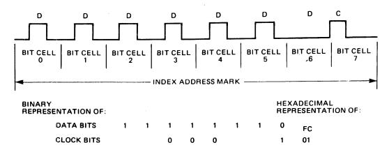
FIGURE 15. MFM INDEX ADDRESS MARK
