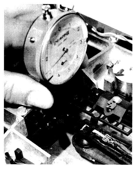
FIGURE 42. DIAL INDICATOR INSTALLATION
