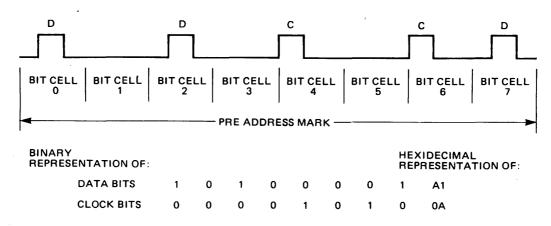
FIGURE 20. MFM PRE ID/DATA ADDRESS MARK
