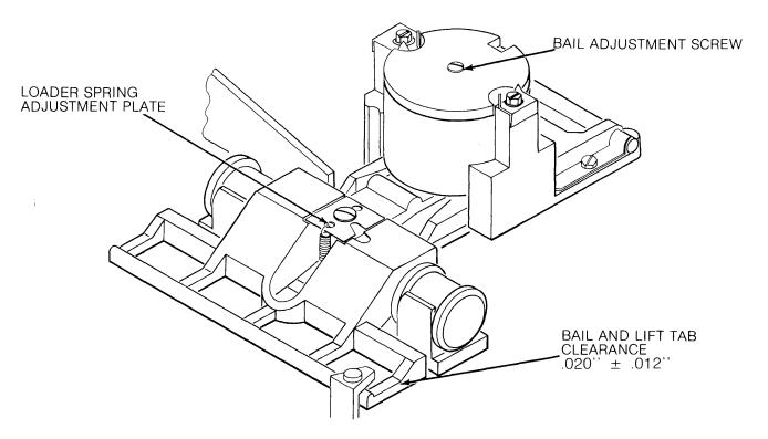
FIGURE 37. HEAD LOAD MECHANISM ADJUSTMENT
