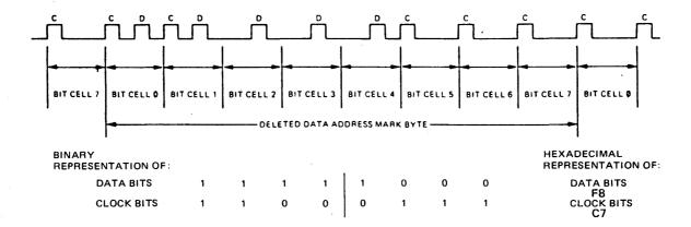
FIGURE 14. DELETED DATA ADDRESS MARK FM
