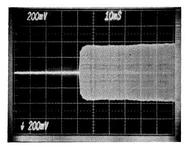
FIGURE 38. HEAD LOAD TIMING
