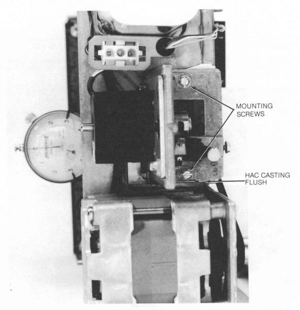
FIGURE 44. PENETRATION ADJUSTMENT
