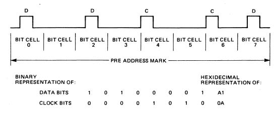
FIGURE 19. MFM PRE ID/DATA ADDRESS MARK
