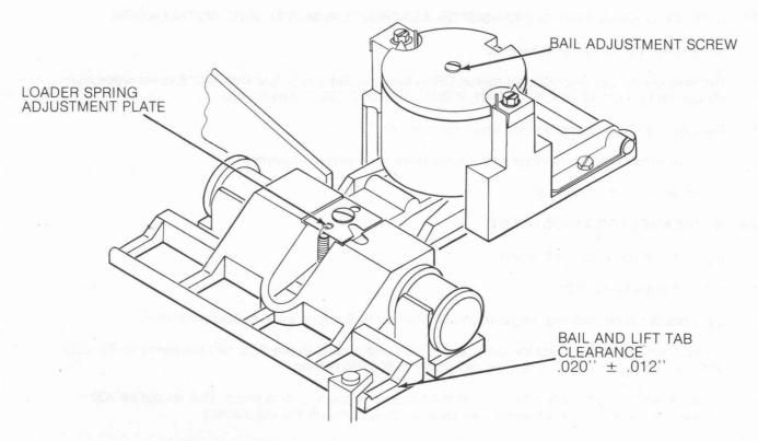
FIGURE 36. HEAD LOAD MECHANISM ADJUSTMENT
