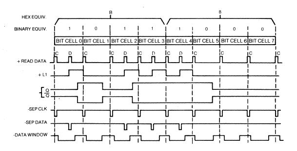
FIGURE 33. DATA SEPARATION TIMING DIAGRAM
