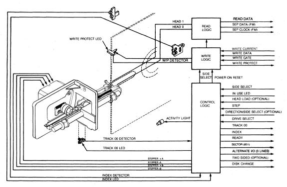
FIGURE 1. SA850/851 FUNCTIONAL DIAGRAM
