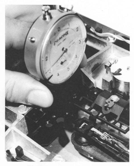
FIGURE 41. DIAL INDICATOR INSTALLATION
