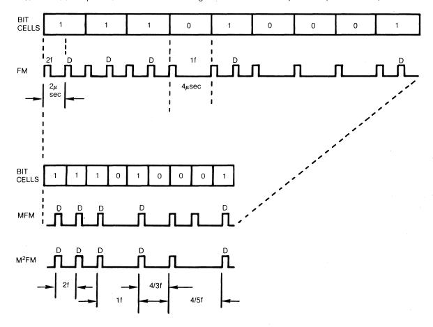
FIGURE 7. FM. MFM AND M2FM ENCODING
