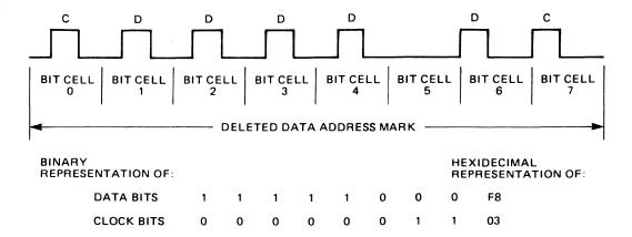
FIGURE 17. MFM DELETED DATA ADDRESS MARK
