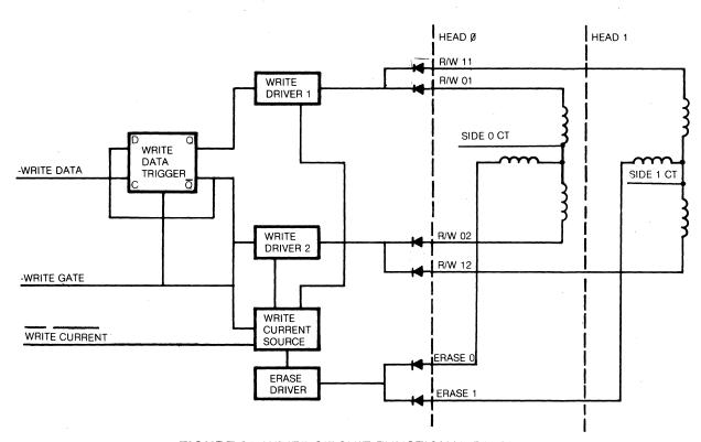
FIGURE 31. WRITE CIRCUIT FUNCTIONAL DIAGRAM
