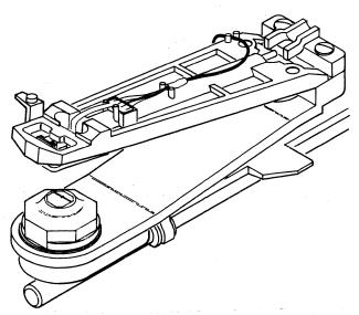
FIGURE 2. BI-COMPLIANT READ/WRITE HEAD
