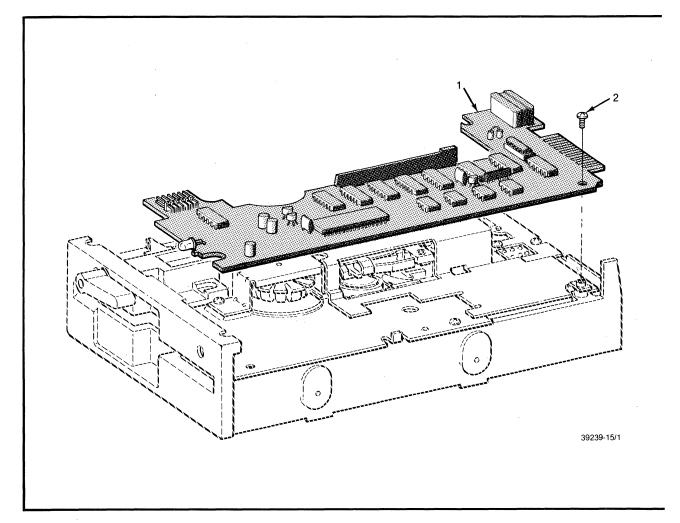
FIGURE 12-1. 455/465 BASIC DRIVE ASSEMBLY (SHEET 1 OF 4)
