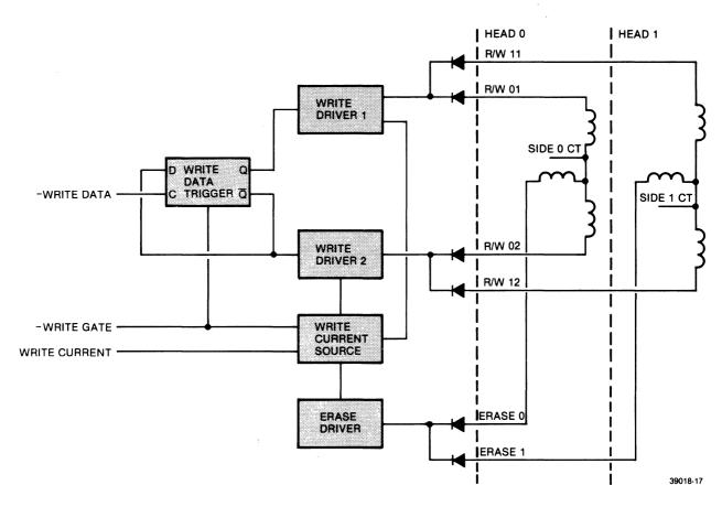
FIGURE 8-7. WRITE CIRCUIT FUNCTIONAL DIAGRAM
