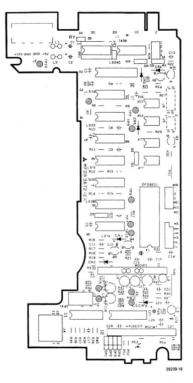
FIGURE 10-12. PCB COMPONENT/TEST POINT LOCATIONS, P/N 25284 (455), P/N 25286 (465)
