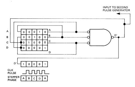
FIGURE 17. STEP IN LOGIC
