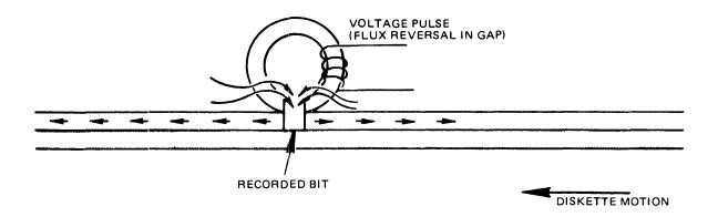
FIGURE 21. READING A BIT
