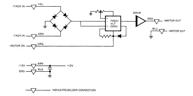
MOTOR SPEED CONTROL PCB LOGIC DIAGRAM AMPLITUDE MODULATION PCB P/N 25129
