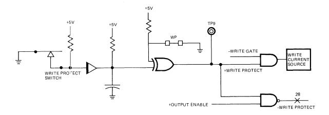
FIGURE 26. WRITE PROTECT FUNCTIONAL DIAGRAM
