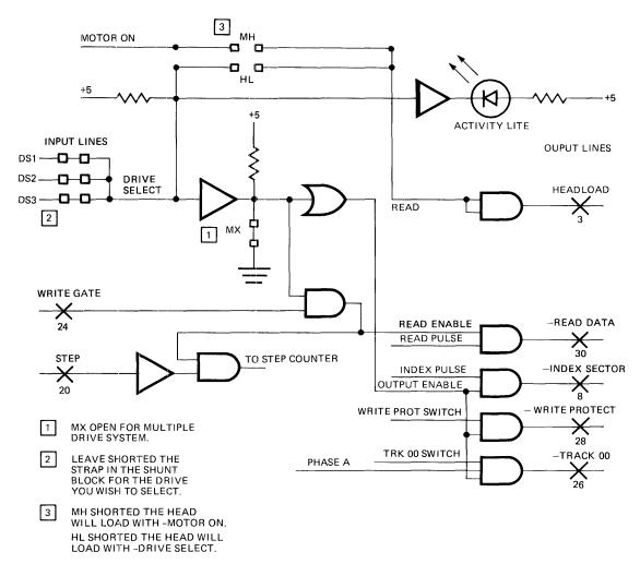
FIGURE 9. DRIVE SELECT FUNCTIONAL DIAGRAM
