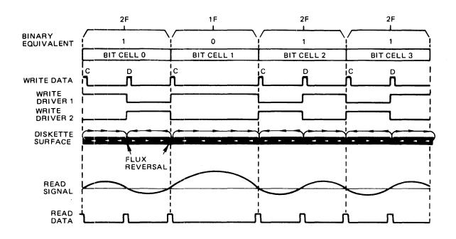
FIGURE 22. 1F AND 2F RECORDING FLUX AND PULSE RELATIONSHIP
