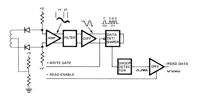
FIGURE 25. READ CIRCUIT FUNCTIONAL DIAGRAM
