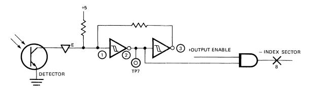
FIGURE 10. INDEX DETECTOR LOGIC
