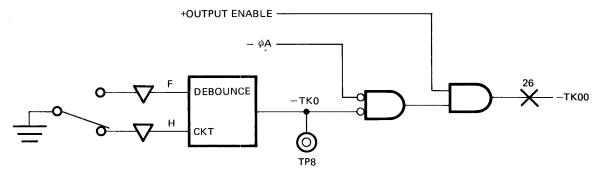
FIGURE 12. TRACK 00 INDICATION DIAGRAM
