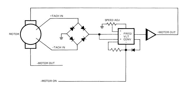
FIGURE 8. MOTOR CONTROL FUNCTIONAL DIAGRAM
