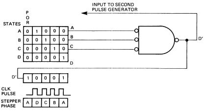
FIGURE 14. STEP OUT LOGIC
