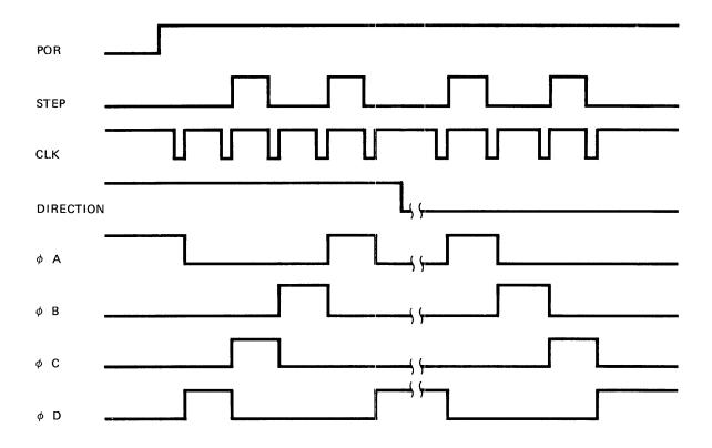
FIGURE 16. STEP TIMING DIAGRAM
