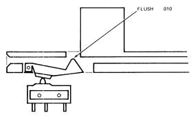
FIGURE 13. WRITE PROTECT SWITCH ADJUSTMENT
