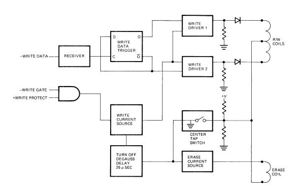
FIGURE 24. WRITE CIRCUIT FUNCTIONAL DIAGRAM
