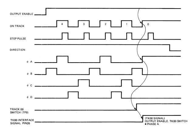
FIGURE 13. TRACK 00 TIMING DIAGRAM
