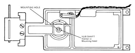
FIGURE 3. HUB FRAME ADJUSTMENT
