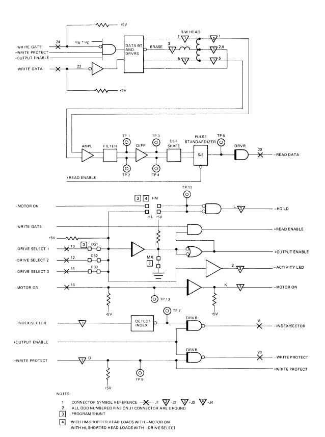
DRIVE PCB LOGIC DIAGRAM PCBP/N 25060 READ/WRITE, INDEX, WRITE PROTECT, DRIVE SELECTION
