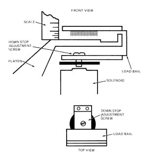
FIGURE 14. HEAD LOAD BAIL ADJUSTMENT
