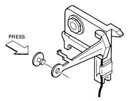
FIGURE 2. HEAD LOAD BUTTON REPLACEMENT
