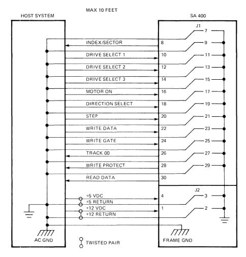
FIGURE 28. SA400 INTERFACE CONNECTIONS
