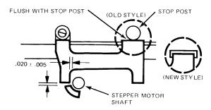
FIGURE 6. CARRIAGE LIMITER ADJUSTMENT
