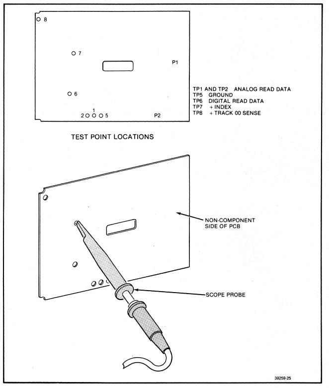
FIGURE 5-6. TEST POINT LOCATIONS AND PROBE POSITIONING
