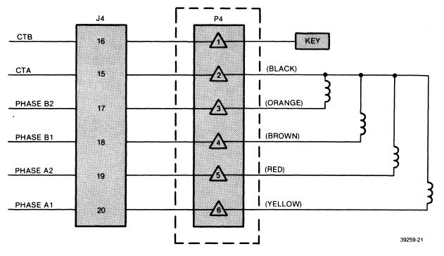
FIGURE 10-3. STEPPER MOTOR HARNESS CONNECTIONS
