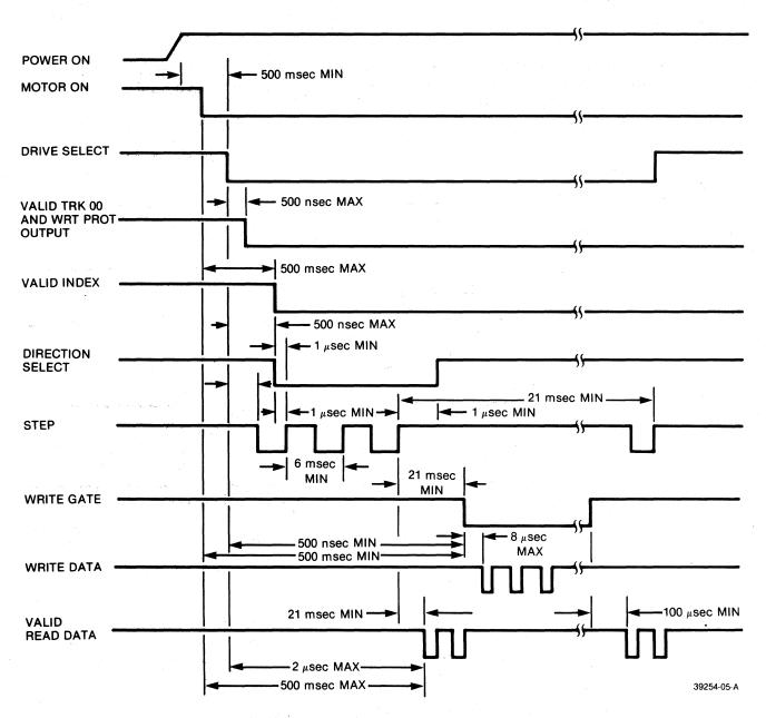
FIGURE 1-11. GENERAL CONTROL AND DATA TIMING REQUIREMENTS
