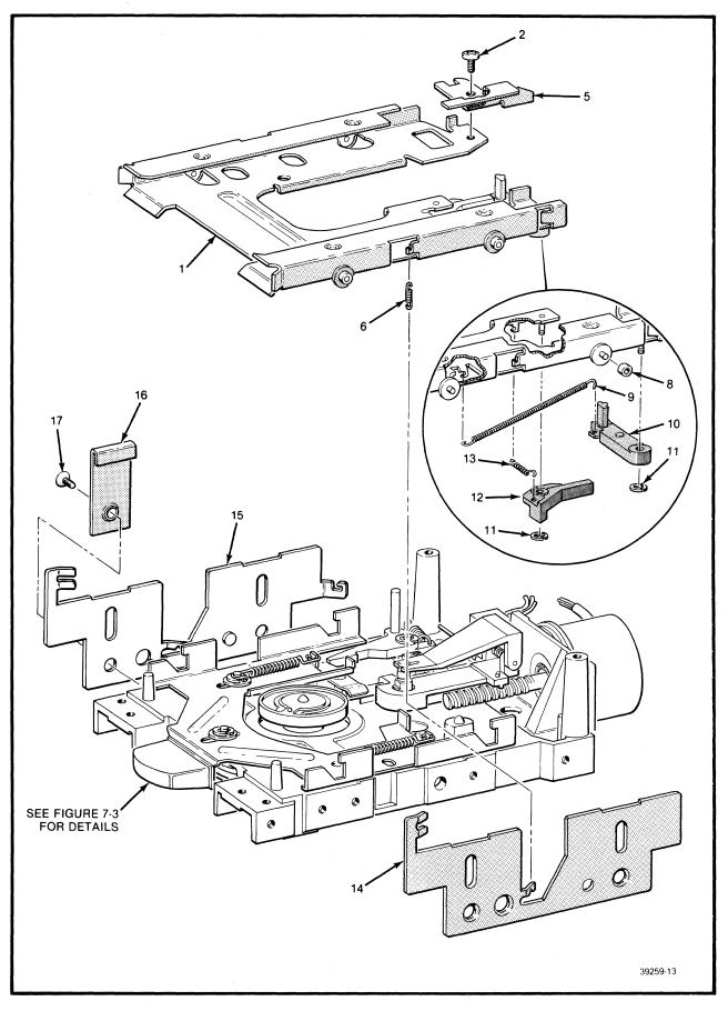
FIGURE 7-2. PLATFORM EJECTOR/ELEVATOR ASSEMBLY
