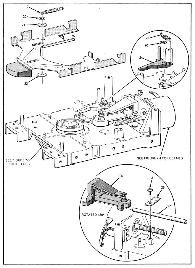
FIGURE 7-3. EJECTOR HEAD AND CARRIAGE ASSEMBLY
