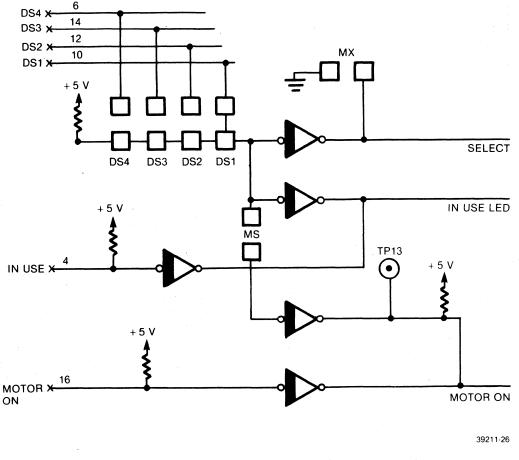
FIGURE 4-12. DRIVE SELECT, MOTOR ON AND IN USE
