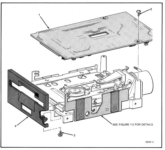
FIGURE 7-1. DRIVE PCB AND FACE PLATE ASSEMBLY
