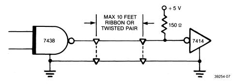
FIGURE 2-2. INTERFACE SIGNAL DRIVER/RECEIVER
