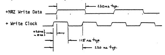
Figure 9. MFM ENCODE TIMING
