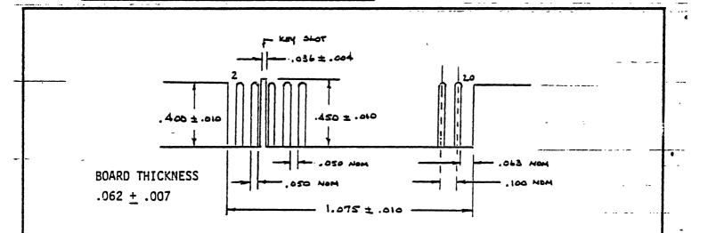
Figure 1. J1, J2, J3, and J4 CONNECTOR DIMENSIONS
