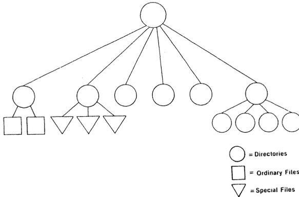
Figure 1-3: The Hierarchical Structure of the File System
