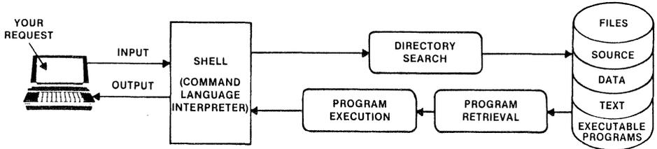
Figure 1-5: Execution of a UNIX System Command
