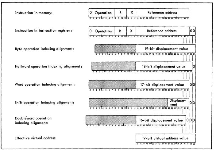
Figure 4. Index Displacement Alignment
