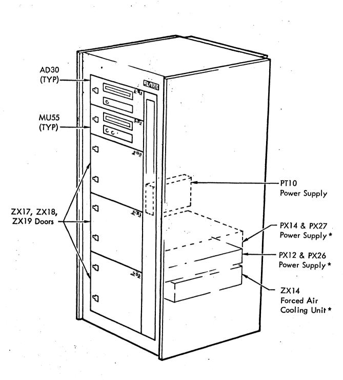
\* Power Supply and Cooling Unit Mount from Rear
