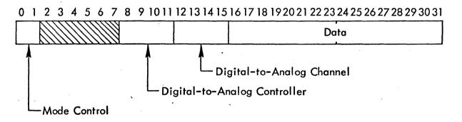
Load the first-rank register of the addressed converter but perform no other action.
