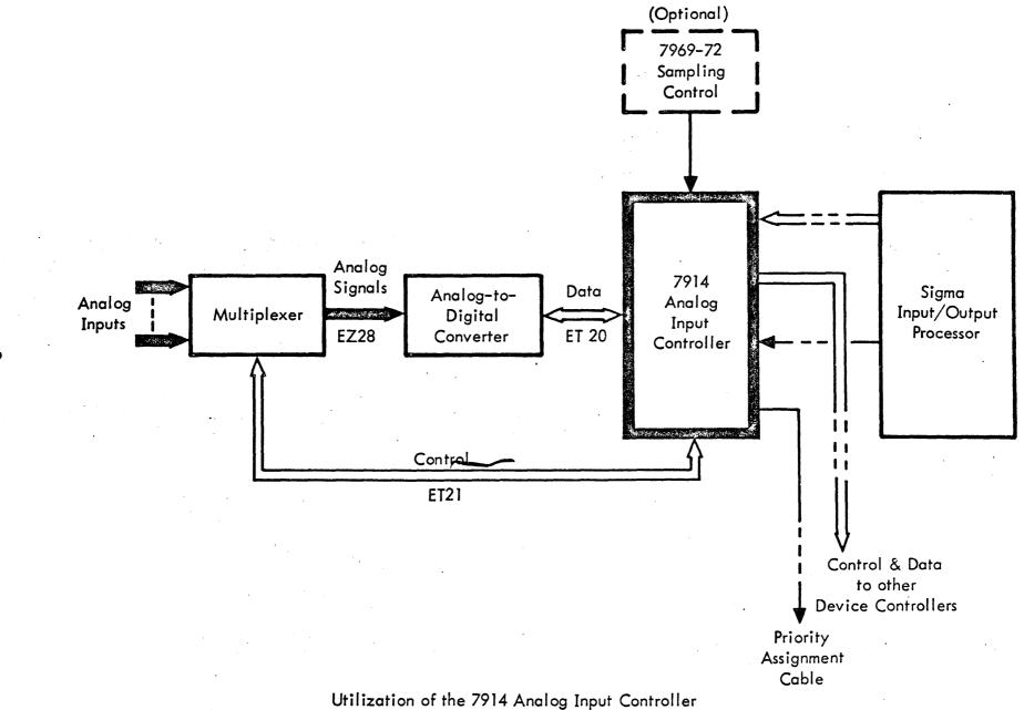
Control of the 7914 is dependent upon the program stored in the Sigma computer. An I/O Command Doubleword is placed in the register for the selected I/O channel. This IOCD contains the memory address of the first byte to be output, the number of bytes to be trans-ferred, and certain control information.
