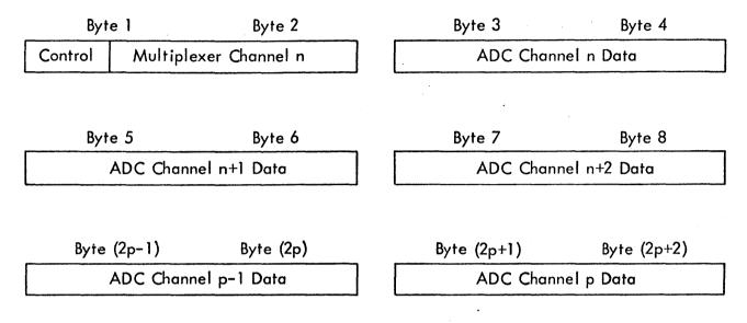
The multiplexer selects channels in sequence by channel number; however, any section of the multiplexer "list" can be selected for readout. The 12-bit field indicates the starting channel number, and the IOCD specifies the number of sequential channels to multiplex.
