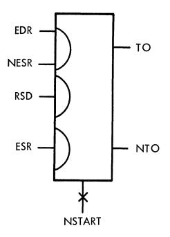
Figure 3-6. Terminal Order Control Flip-Flop
