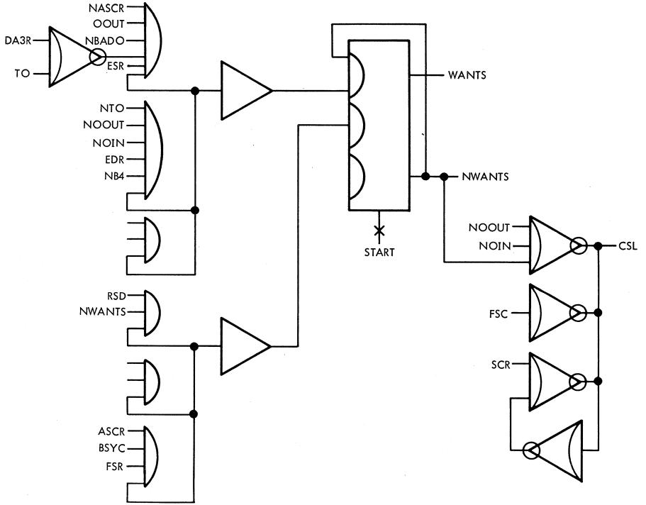
Figure 3-9 "WANT SERVICE" Control Flip-Flop
