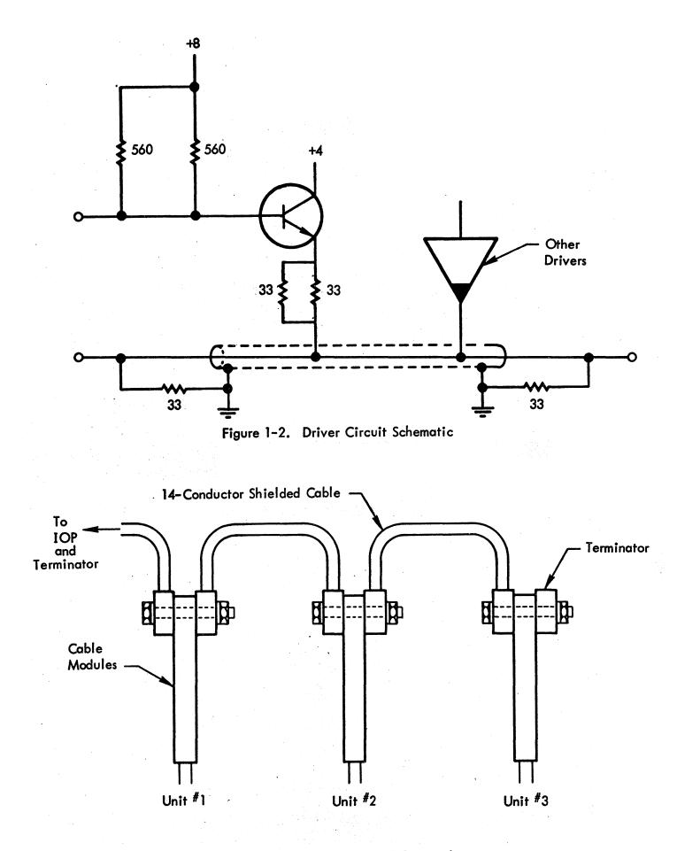
Figure 1–3. Cable and Terminator Connections
