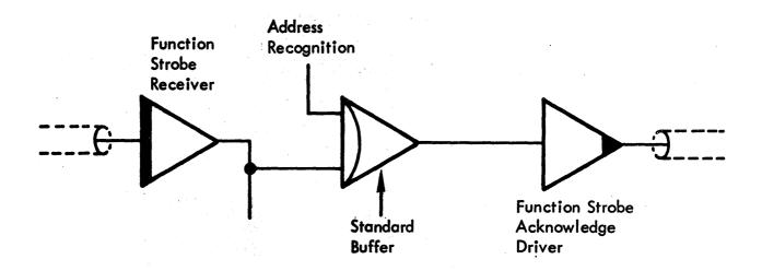
Figure 2-1. Function Strobe Acknowledge Circuit
