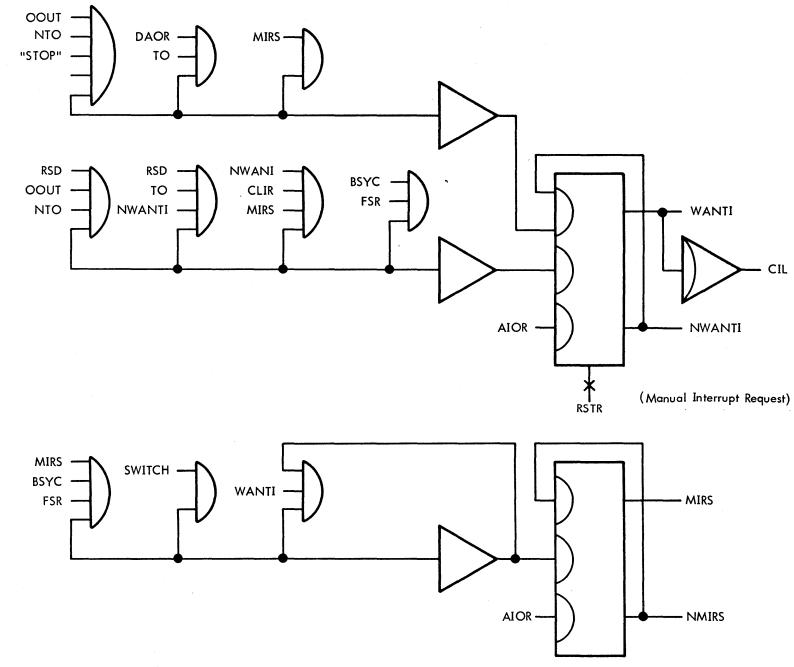
Figure 3-15. "WANT INTERRUPT" Control Flip-Flop
