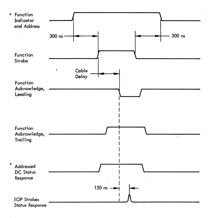
\*No output address for AIO or ASC; DC returns its address with status response.
