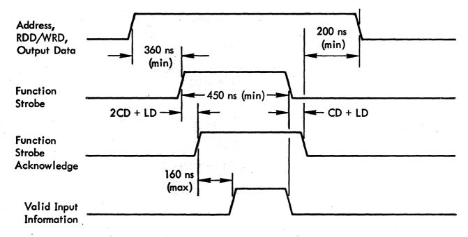
Figure 2-2. Read Direct Timing and Write Direct Timing
