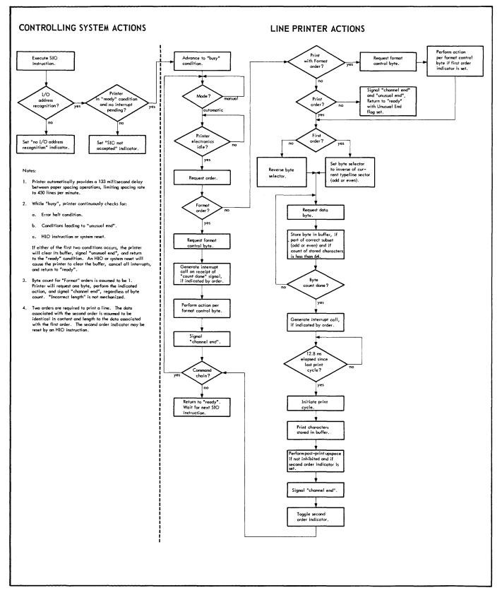
Figure 1. Controlling System/Line Printer Actions
