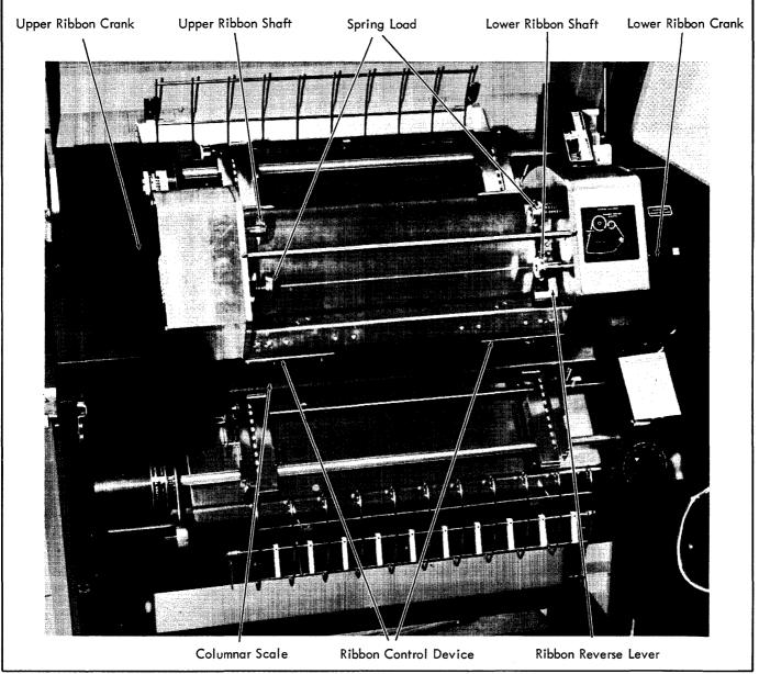
Figure 6. Line Printer Mechanism
