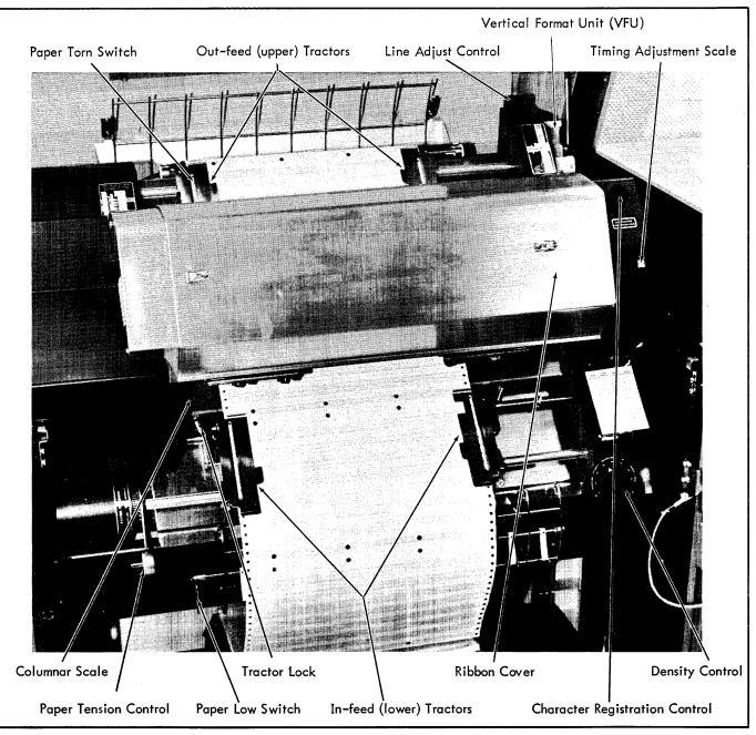
Figure 3. Line Printer Mechanism with Paper Loaded
