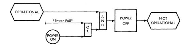
Figure 10. Device State Sequence From "Operational"
