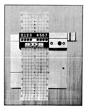
Figure 8. Tape Alignment in VFU Tape Punch
