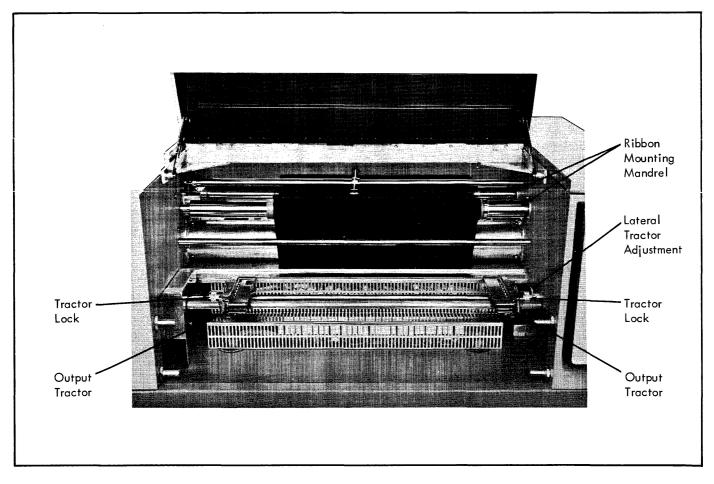
Figure 3. Printer Mechanism, Front View
