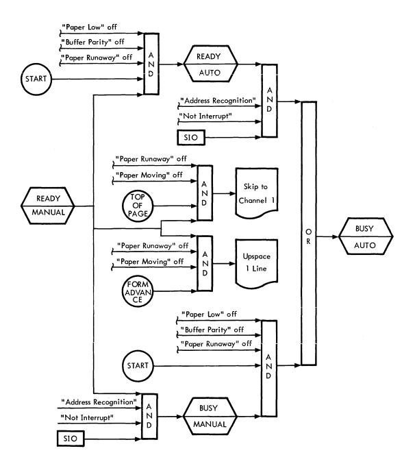
Figure 11. Device State Sequence From "Ready-Manual"
