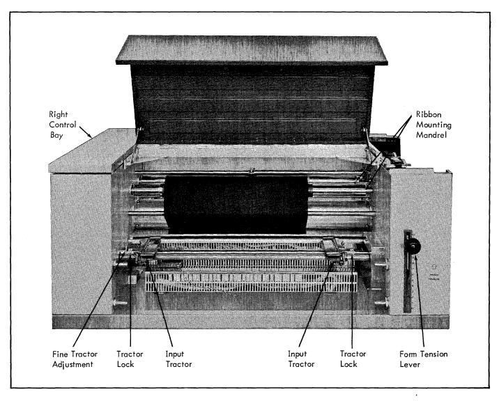
Figure 4. Printer Mechanism, Rear View
