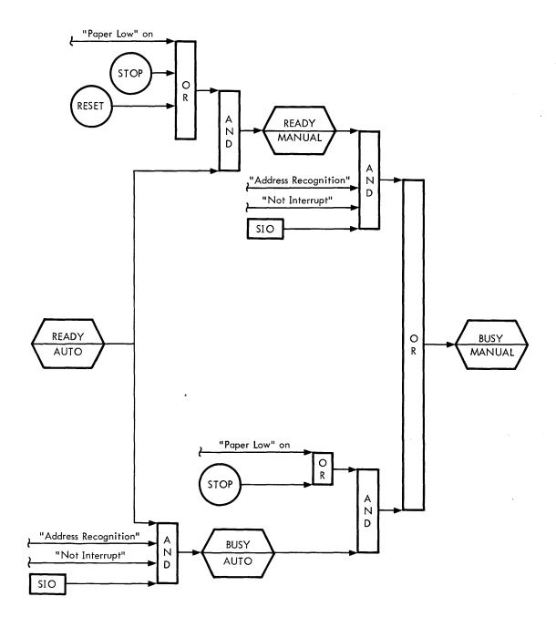
Figure 12. Device State Sequence From "Ready-Auto"
