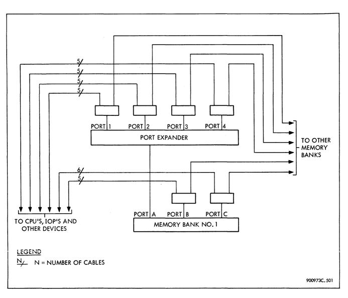
Figure 6-1. Memory Port Expander, Installation Block Diagram
