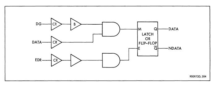
Figure 6-4. Read and Hold Memory Data, Logic Diagram
