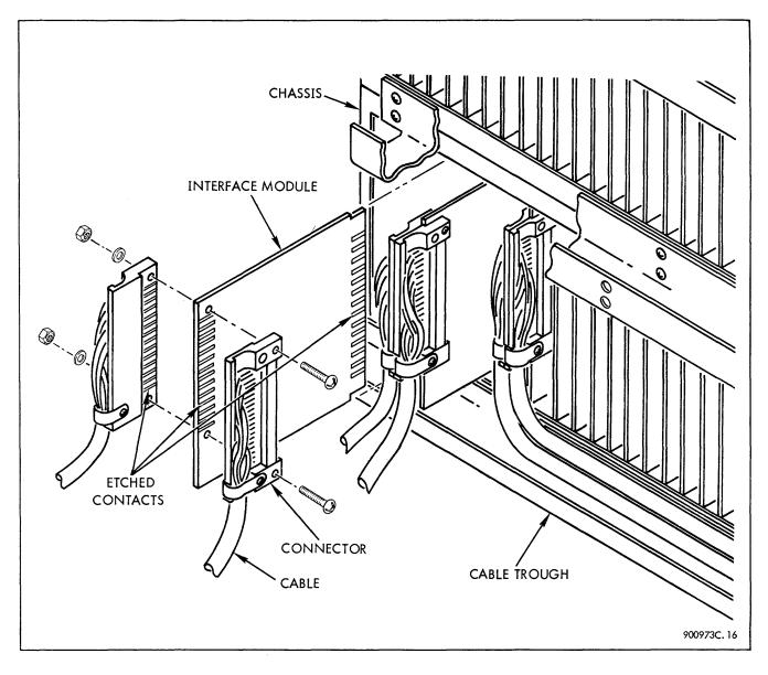
Figure 1-6. Interface Cable Connectors
