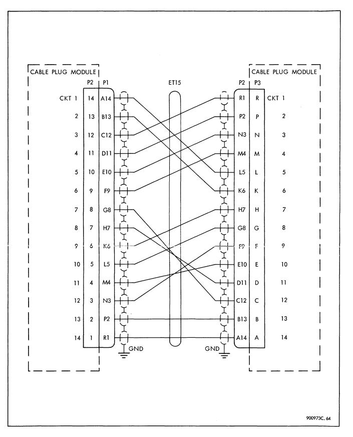
Figure 7-4. ET15 Priority Interrupt, Cable Diagram
