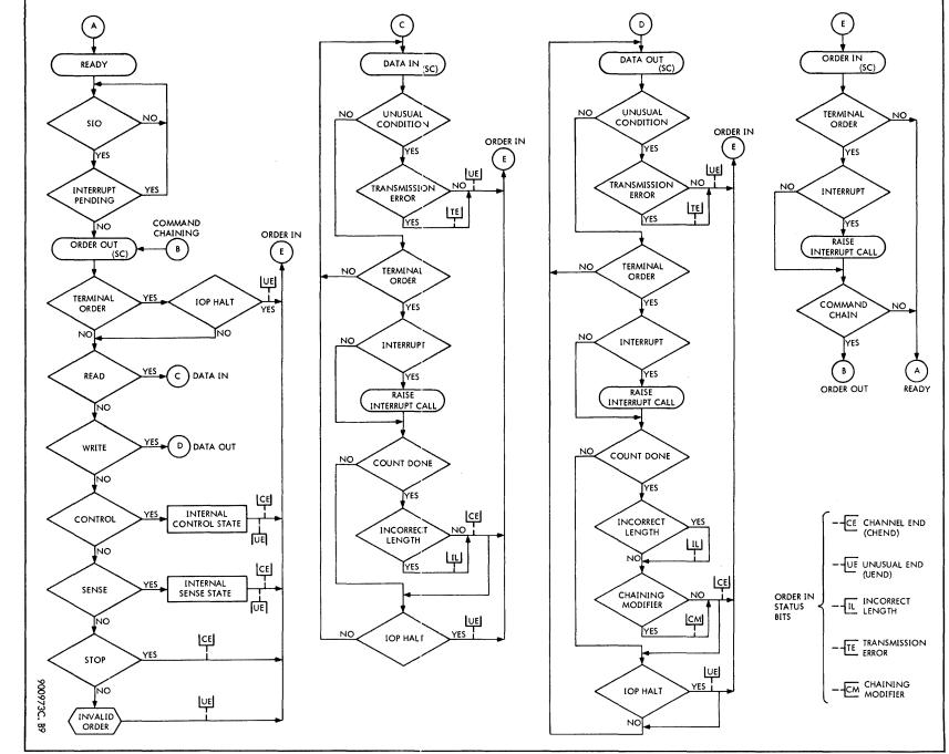
Figure 9-1. Eight-Bit I/O Operational State, Flow Diagram
