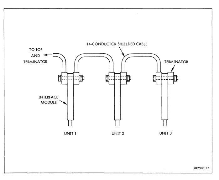
Figure 1-7. Cable and Terminator Connections
