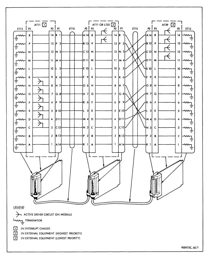
Figure 7-5. Priority Interrupt Interface Connections (Sheet 1 of 4)
