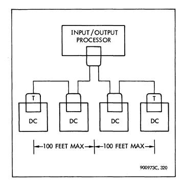
Figure 3-3. Data Transmission Cable Twin Installation
