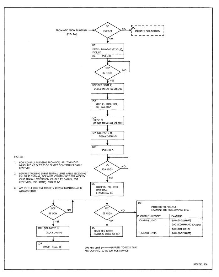
Figure 9-8. Service - Order Input, Flow Diagram
