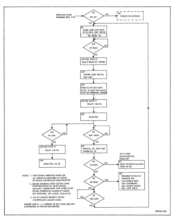
Figure 9-5. Service - Data Input, Flow Diagram
