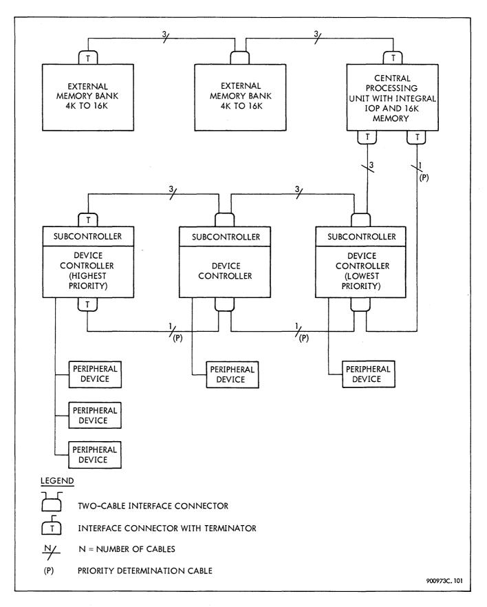
Figure 1-1. Typical Sigma 2 Cabling Scheme
