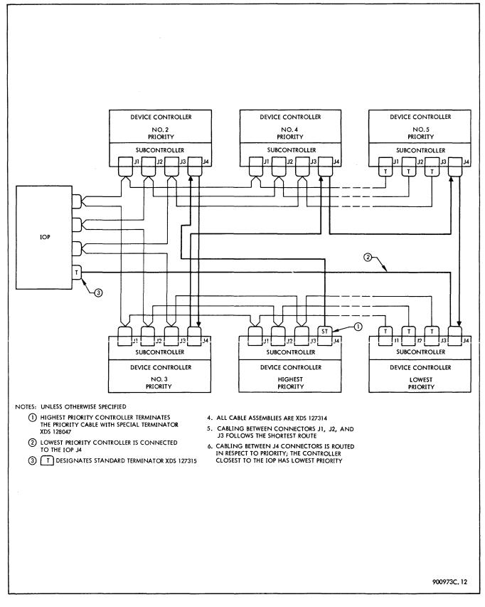
Figure 3-2. Typical I/O Interconnections
