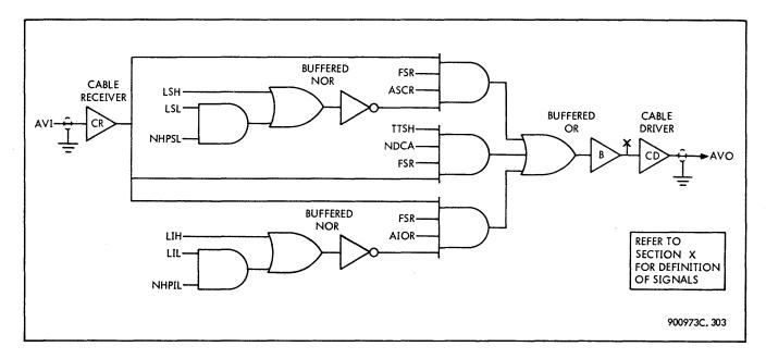
Figure 3-4. Priority Chain, Logic Diagram
