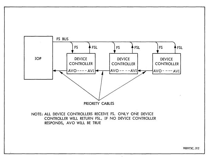
Figure 3-5. Strobe Acknowledge, Interface Diagram
