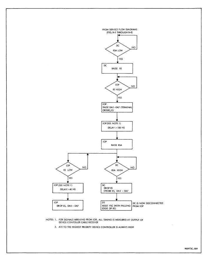
Figure 9-9. Terminal Order, Flow Diagram
