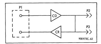
Figure 7-3. AT11 Cable Driver-Cable Receiver Circuit, Schematic Diagram
