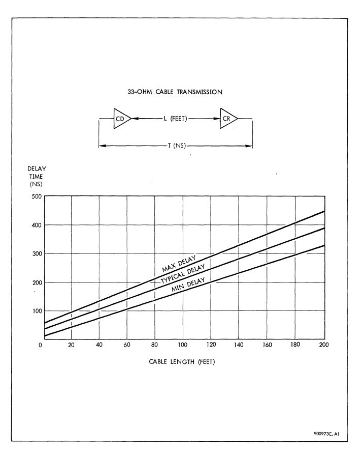
Figure 8-2. Delay as a Function of Cable Length
