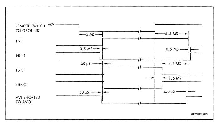
Figure 3-10. Connect-Disconnect, Timing Diagram
