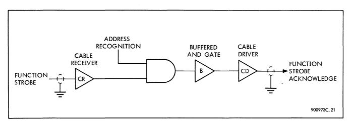
Figure 2-3. Function Strobe Acknowledge, Logic Diagram
