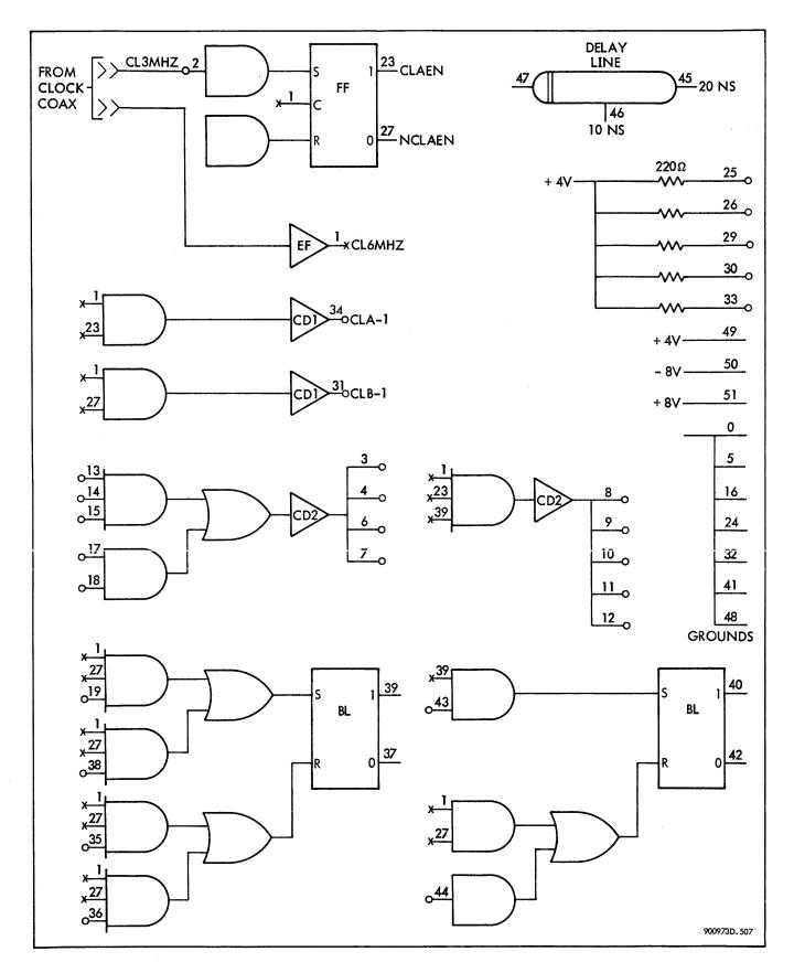
Figure 5-3. AT59 Module, Logic Diagram
