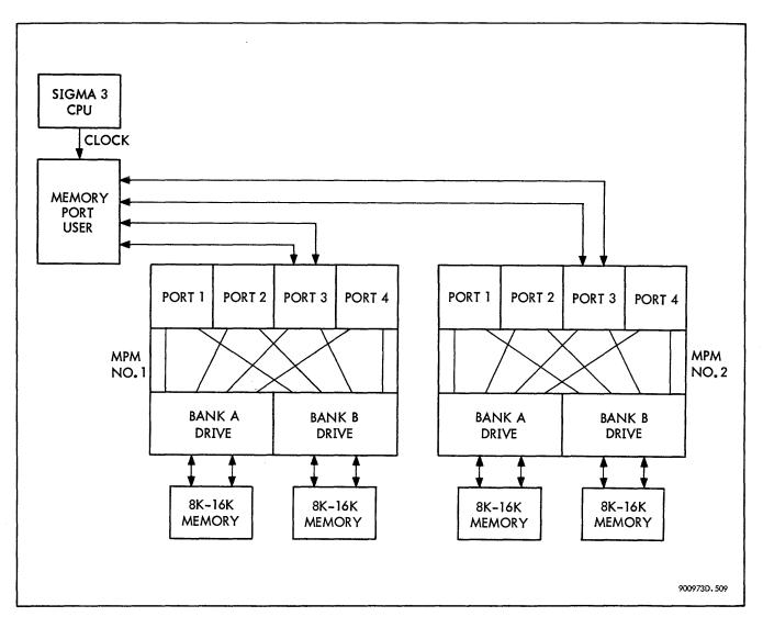
Figure 5-1. Sigma 3 Memory Configuration (Large), Block Diagram
