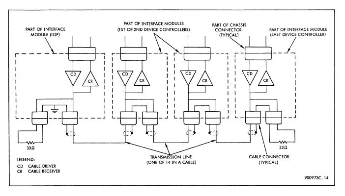
Figure 1-4. Typical Transmission Line Connections
