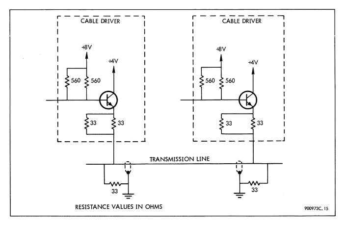
Figure 1-5. Cable Driver Circuit, Simplified Schematic Diagram
