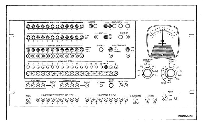
Figure 8-1. Peripheral Equipment Tester Control Panel
