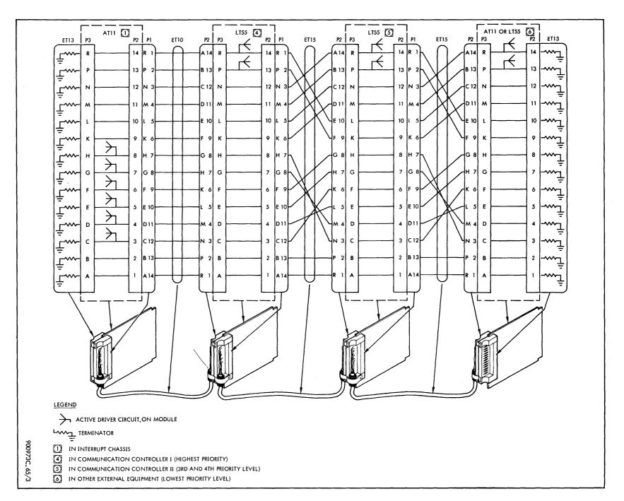
Figure 7-5. Priority Interrupt Interface Connections (Sheet 4 of 4)
