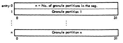
entries point to the location of a segment's partition (if created) either in core or on the program file. T:GRAN has the following format:
