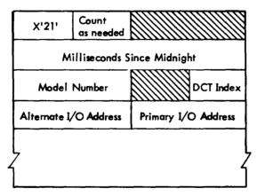
One pair of words per device in DCT order; multiple records may occur (maximum five devices per record).
