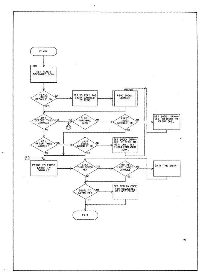
Figure 91. Flow Diagram of FINDX
