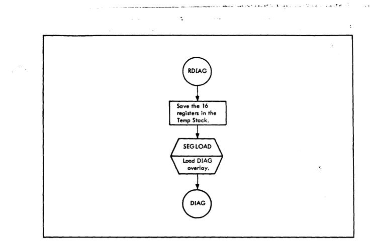
Figure 61. Overlay Loader Flow, RDIAG
