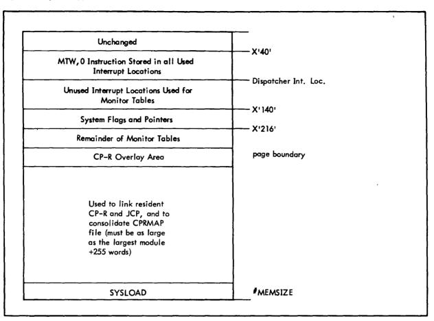
Figure 106 depicts a typical core layout after SYSGEN and SYSLOAD have executed.
