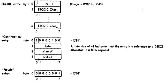
Note that the first byte contains the byte count of the entry (in bits 1-7).
