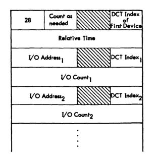
Recorded once per hour and at recovery. Maximum of 5 entries per record. Counts are reset to zero at Boot.
