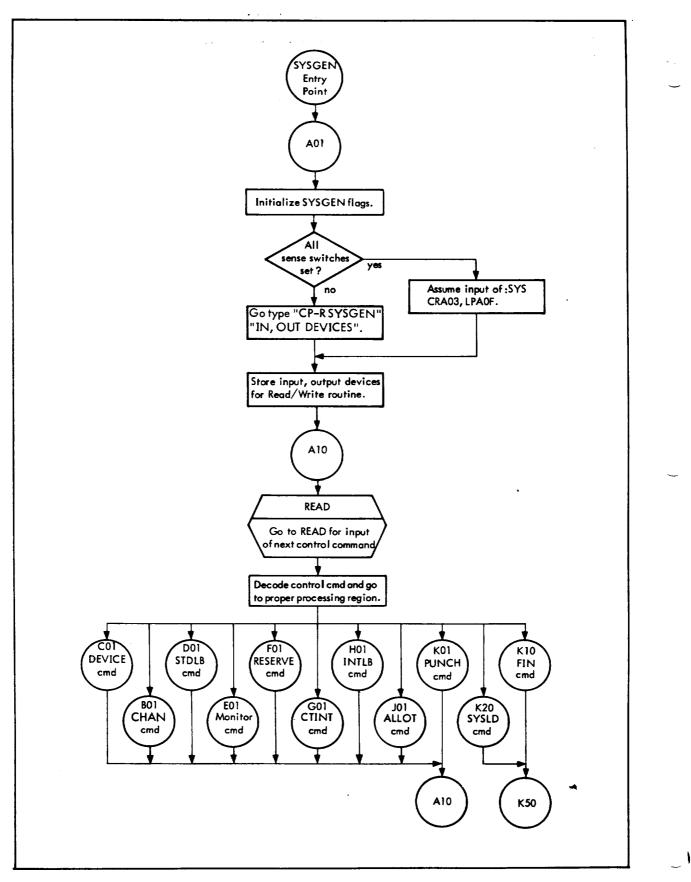
Figure 106. SYSGEN/SYSLOAD Flow
