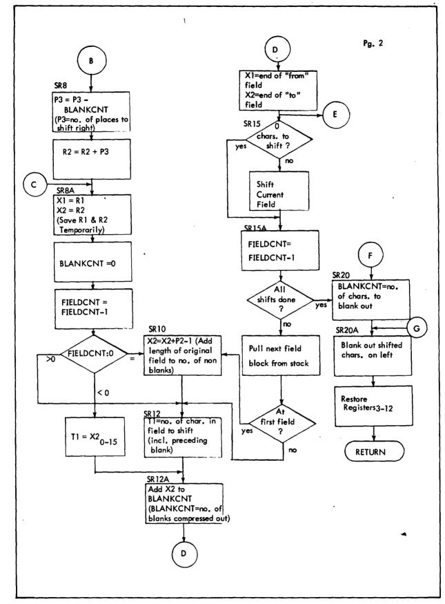
Figure 84. Flow Diagram of SHIFTRIGHT (cont.)
