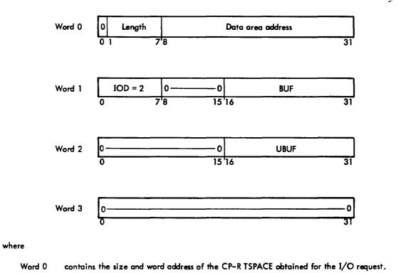
Word 1 IOD = 2 means that the I/O is a READ request and the data record is to be read into a buffer in the TSPACE pointed to from word 0. The data record is moved to the user's virtual buffer address at CHECK time.
