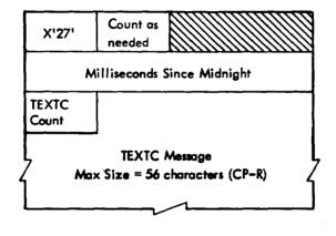
A facility is provided to inject messages from the computer operator (or diagnostic program) into the error log. The operator may enter these messages from the operator console via the ERRSEND key-in.
