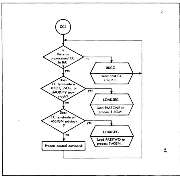
Figure 57. Overlay Looder Flow, CCI
