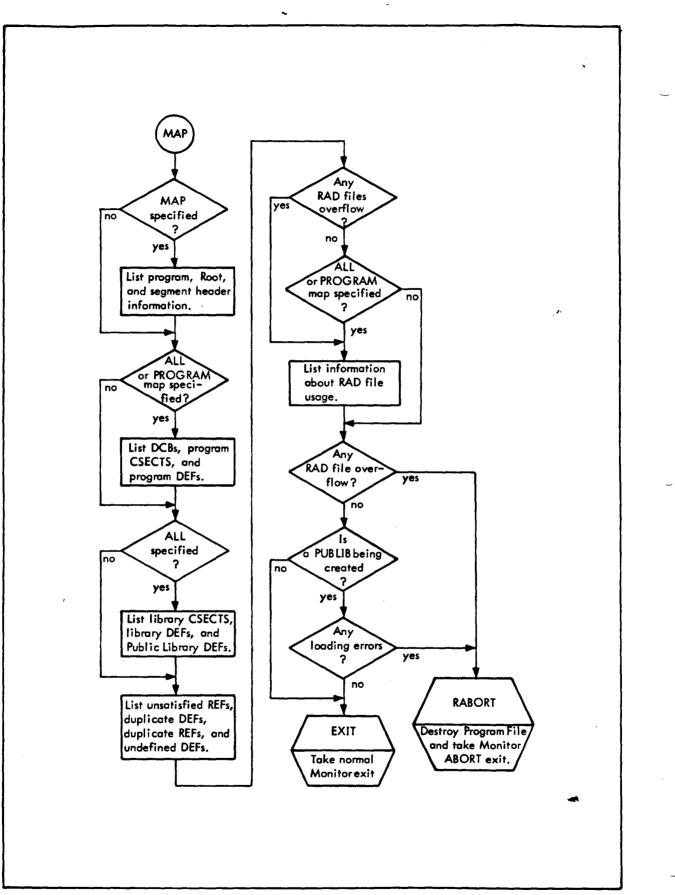
Figure 60. Overlay Loader Flow, MAP
