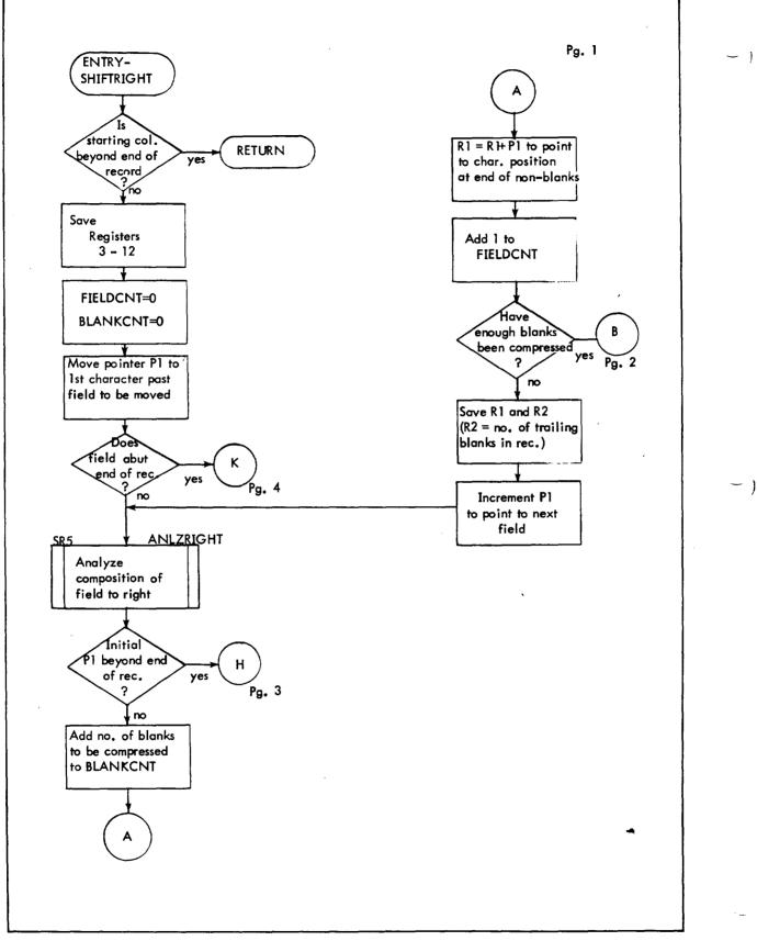
Figure 84. Flow Diagram of SHIFTRIGHT
