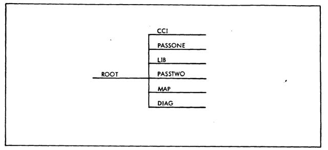
Figure 50. Overlay Structure of the Overlay Loader
