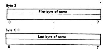
This item declares a label (in EBCDIC code) that is an external definition within the current object module. The name may not exceed 63 bytes in length.
