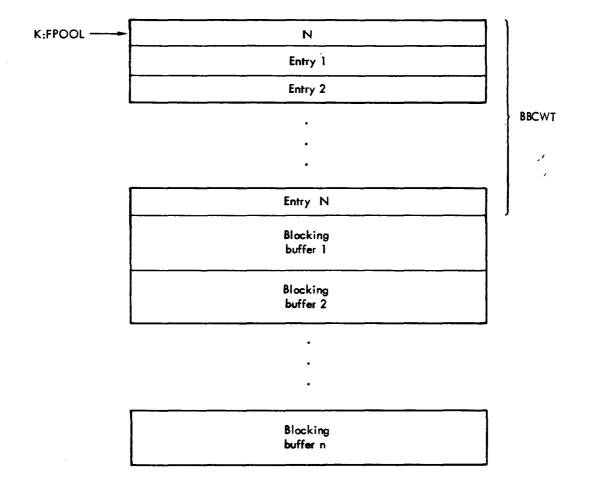
In addition, a maximum of twelve pages will be made available to each job for blocking buffers from the job's Reserved Pages. Secondary tasks will be allocated blocking buffers from these pages as they are needed. The BBCW table is kept in the job's JCB and is constructed and maintained as blocking buffers are required and released.
