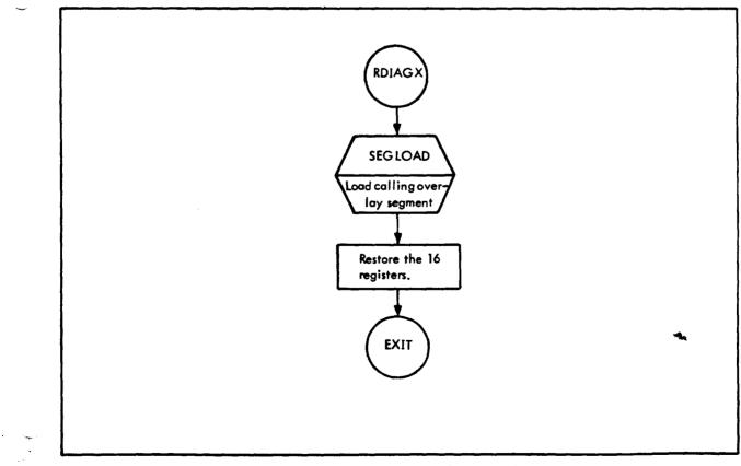
Figure 62. Overlay Loader Flow, RDIAGX
