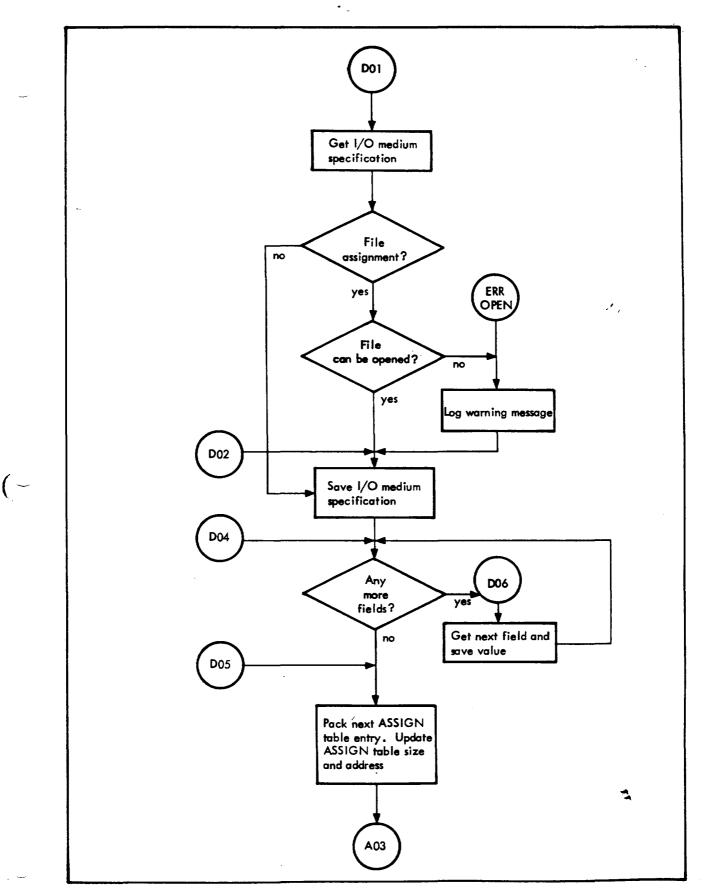
Figure 24. ASSIGN Command Flow
