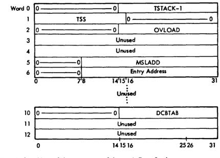
The PCB exists as part of the Root segment and is initialized as shown below by PASSTWO, when the Root segment is created.
