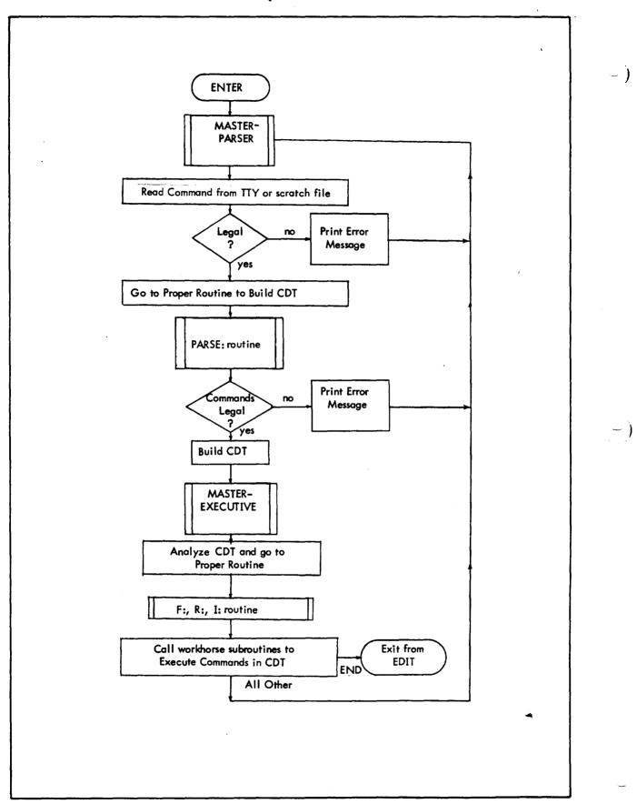
Figure 73. Overall Flow Diagram of EDIT
