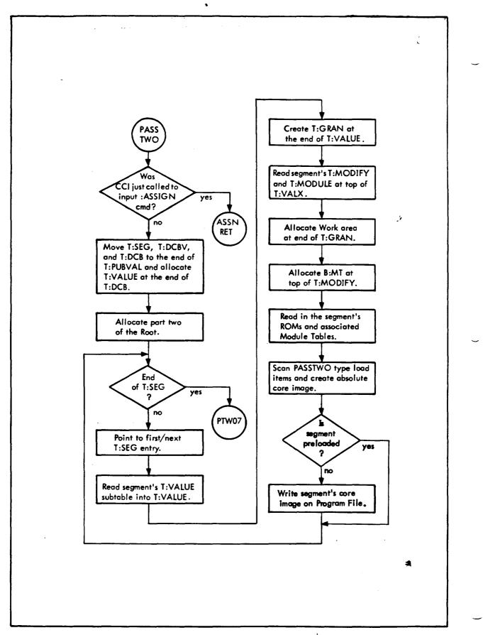
Figure 59. Overlay Loader Flow, PASSTWO
