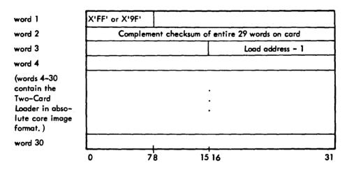
The CPR Tables, SYSLOAD, and the CPR Symbol Table are output in the core image format
