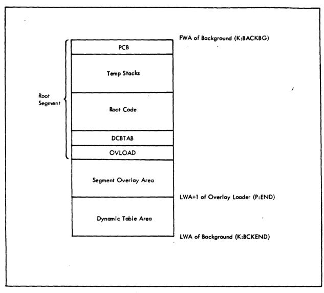
Figure 51. Overlay Loader Core Layout
