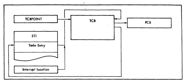
Figure 45. Relationship between a Primary Task Control Block and Other Control Blocks
