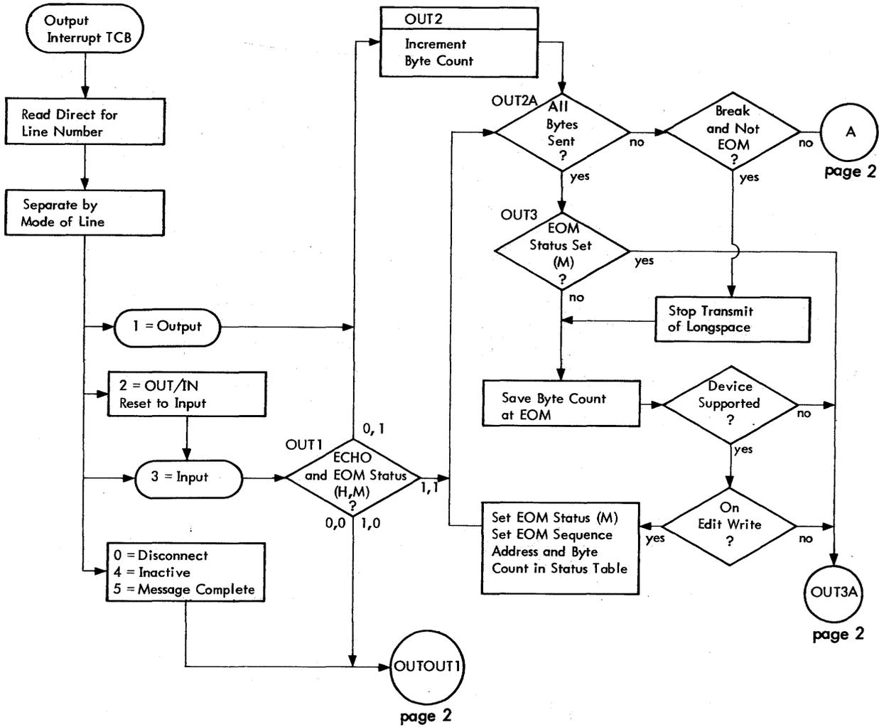
Figure 74. R:COG Output Interrupt Handler
