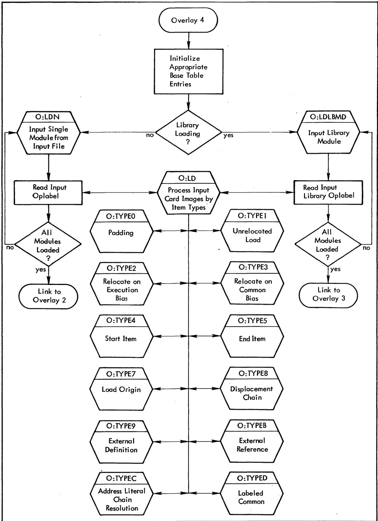
Figure 62. BLOAD Overlay 4 Structure
