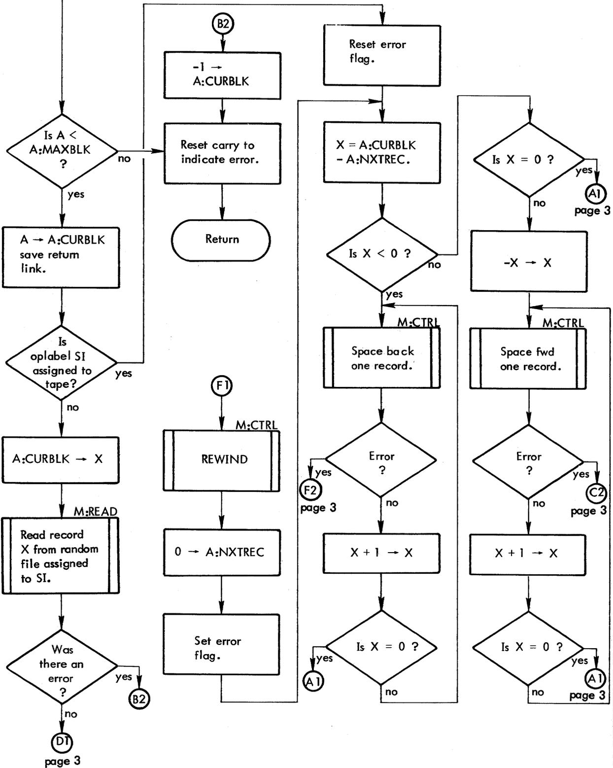
Figure 78. Data Acquisition Subroutines LDWD and LDNXT (cont.)
