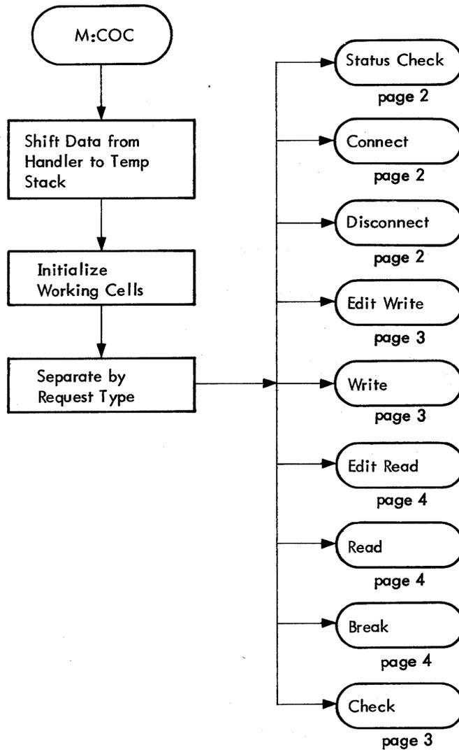
Figure 76. M:COC Request Processing
