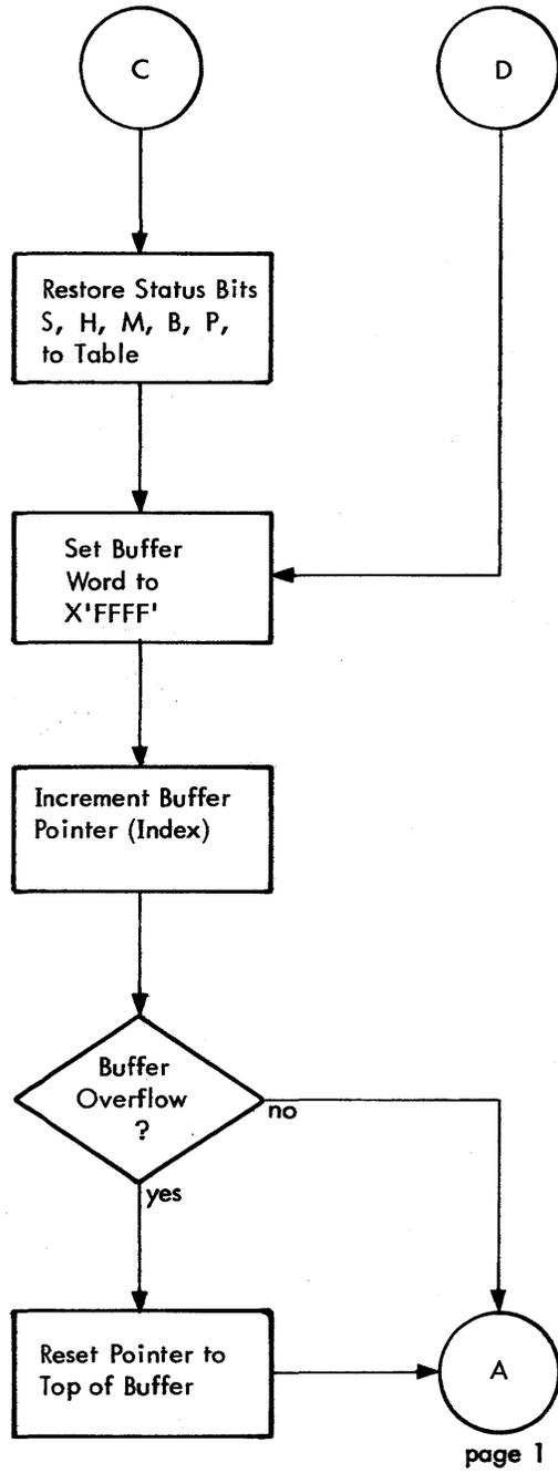
Figure 73. R:COC Input Interrupt Handler (cont.)
