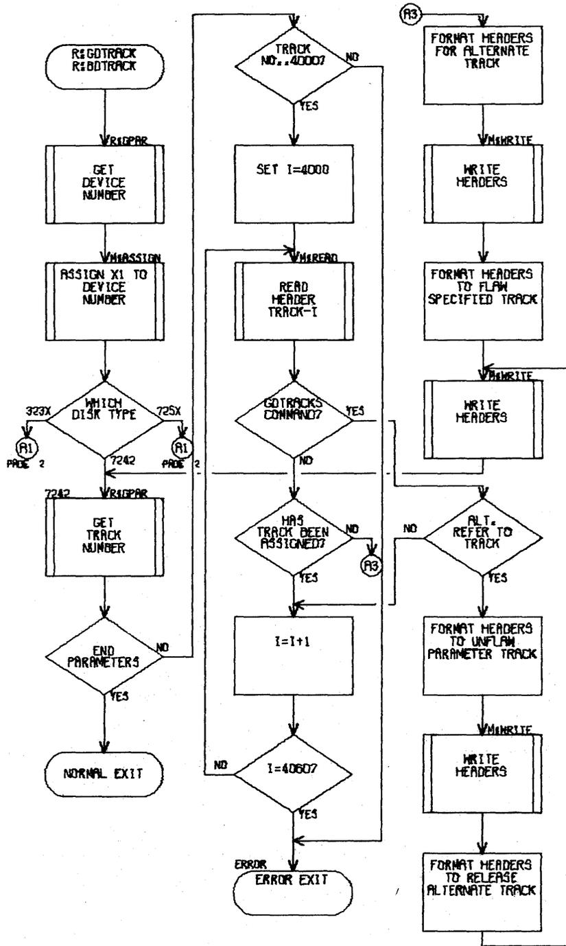
Figure 72. GDTRACKS, BDTRACKS Command Flow Diagram
