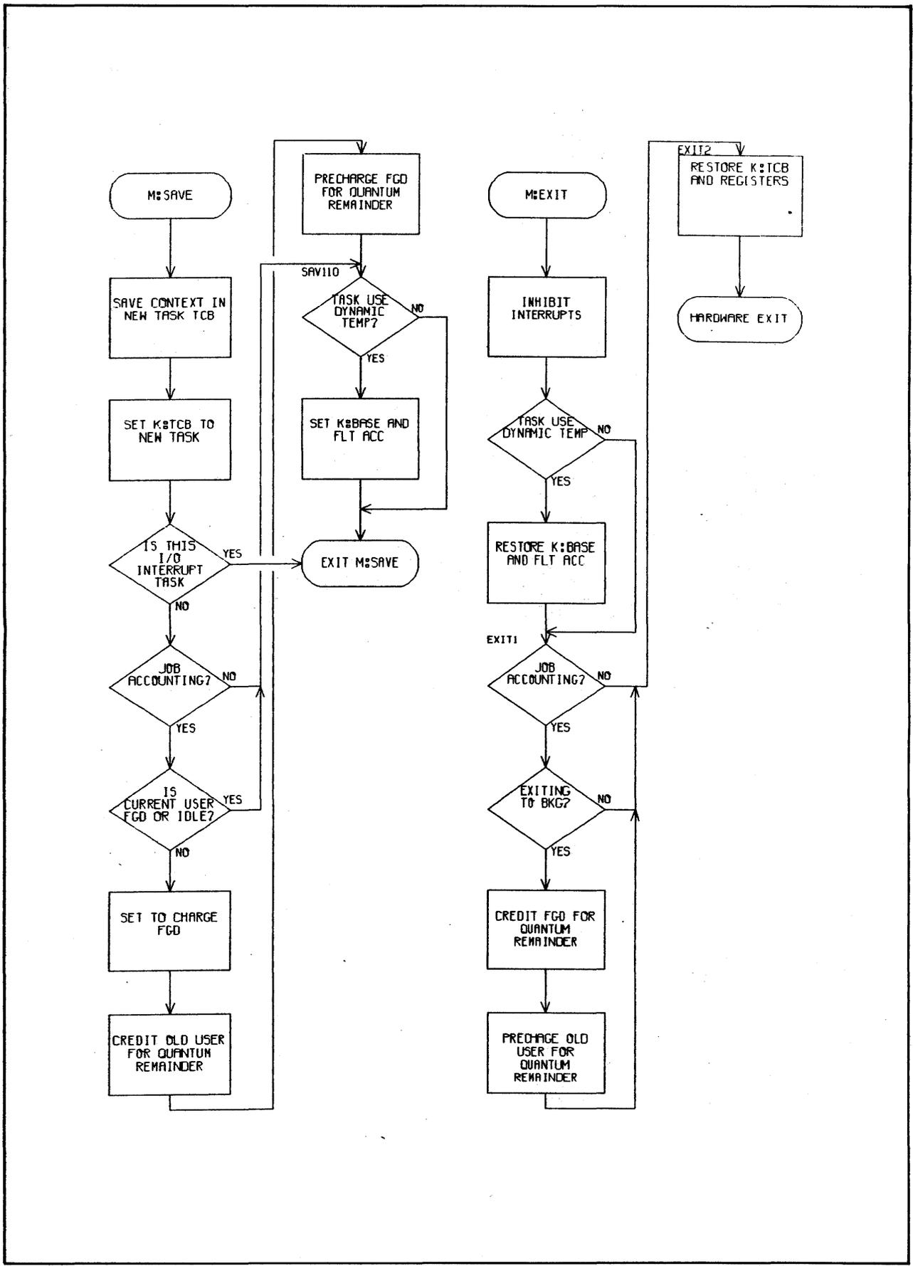
Figure 7. RBM M:SAVE/M:EXIT Task Flow
