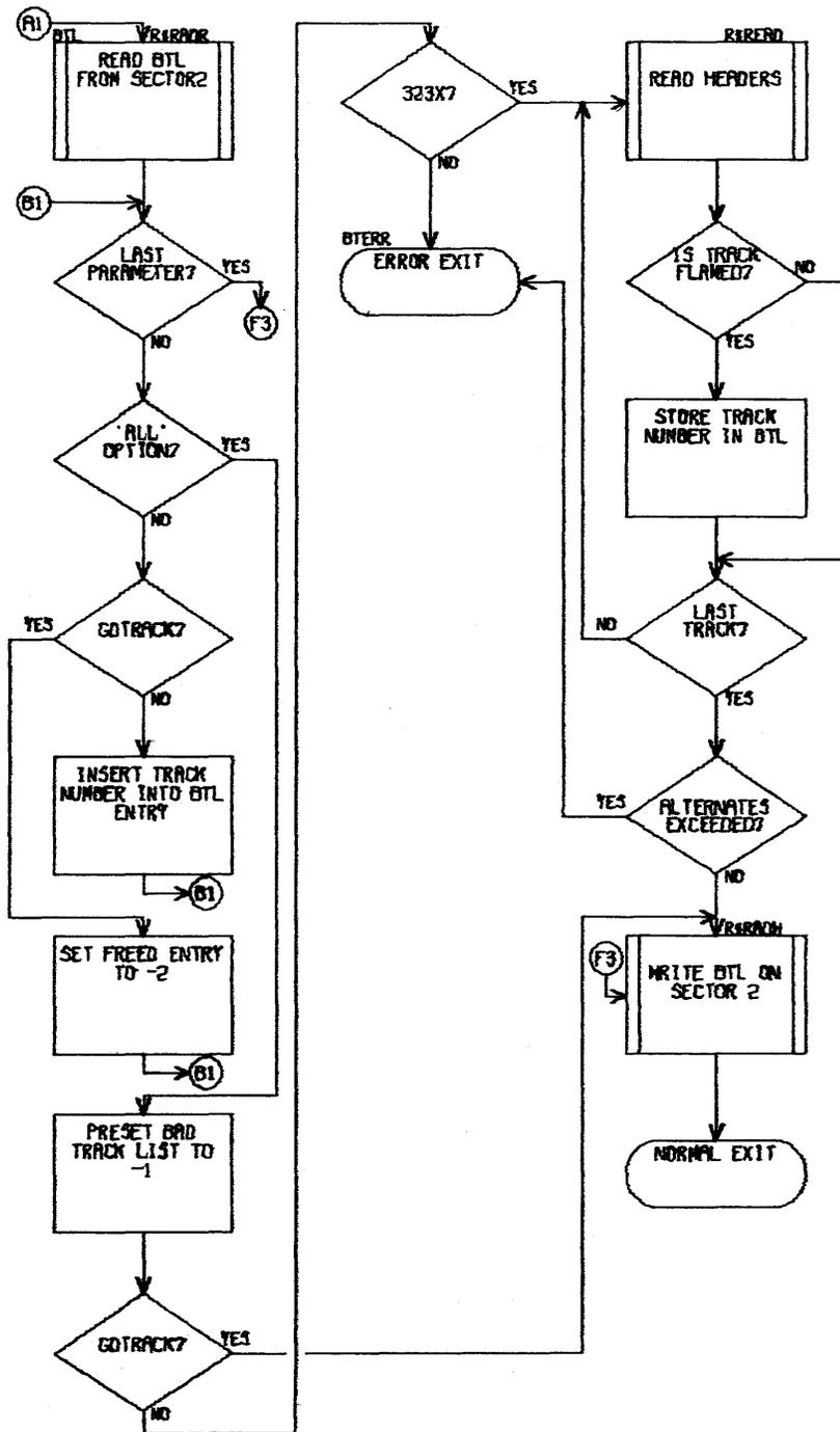
Figure 72. GDTRACKS, BDTRACKS Command Flow Diagram (cont.)
