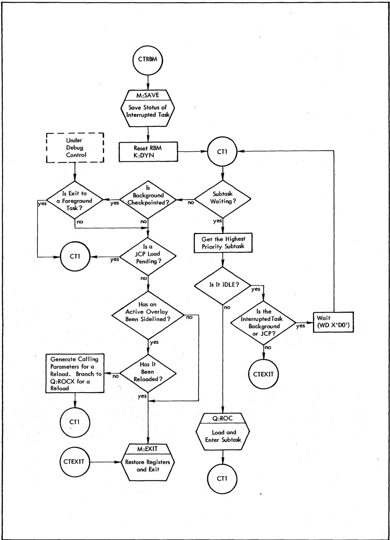
Figure 6. RBM Control Task Flow
