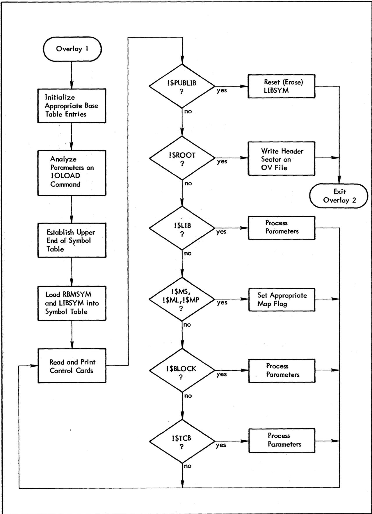
Figure 46. Overlay 1 Structure
