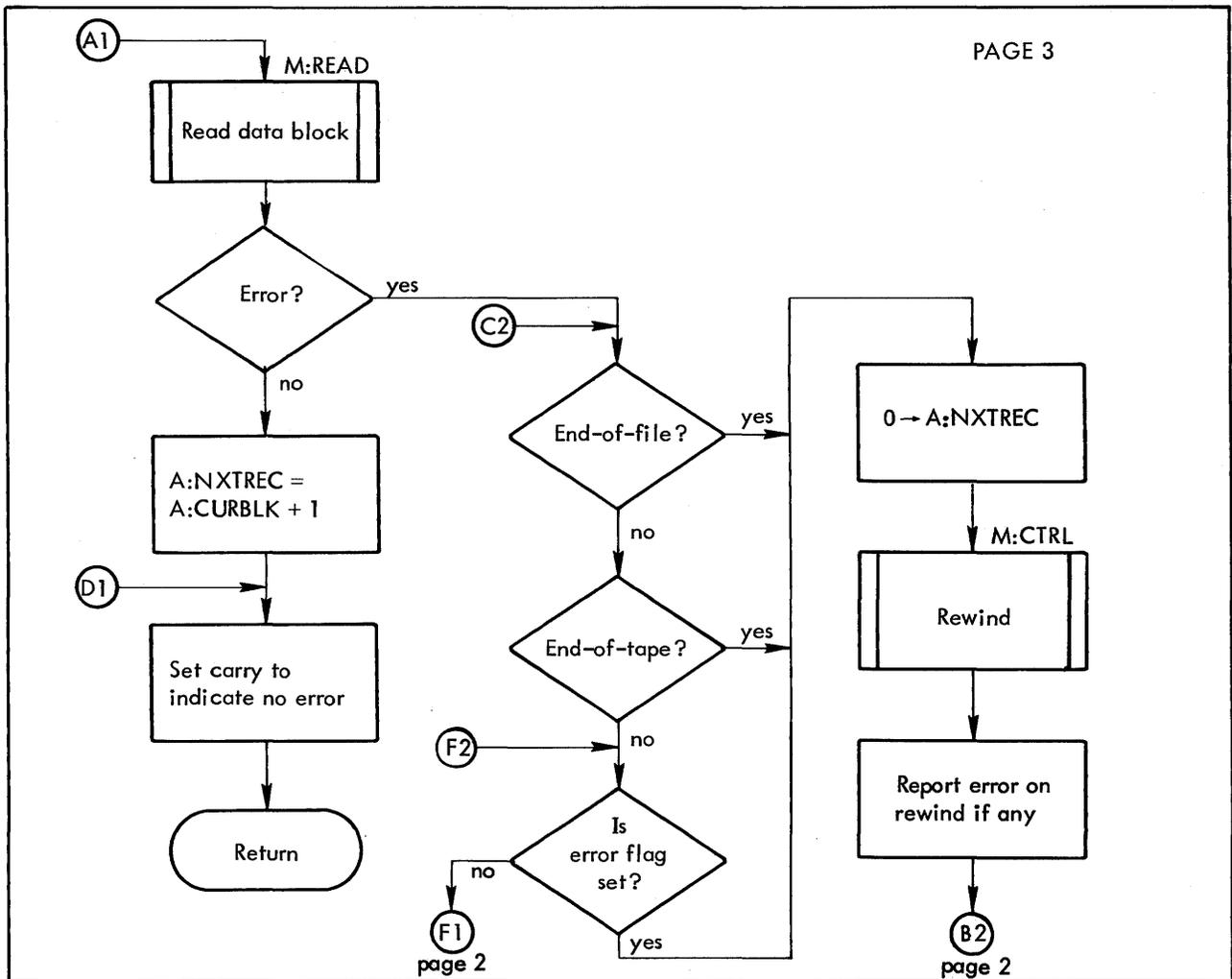
Figure 78. Data Acquisition Subroutines LDWD and LDNXT (cont.)
