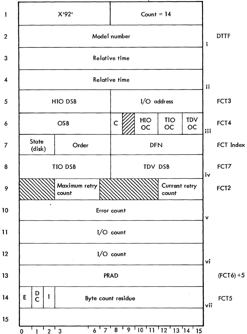
Figure 88. Device-Timeout Entry
