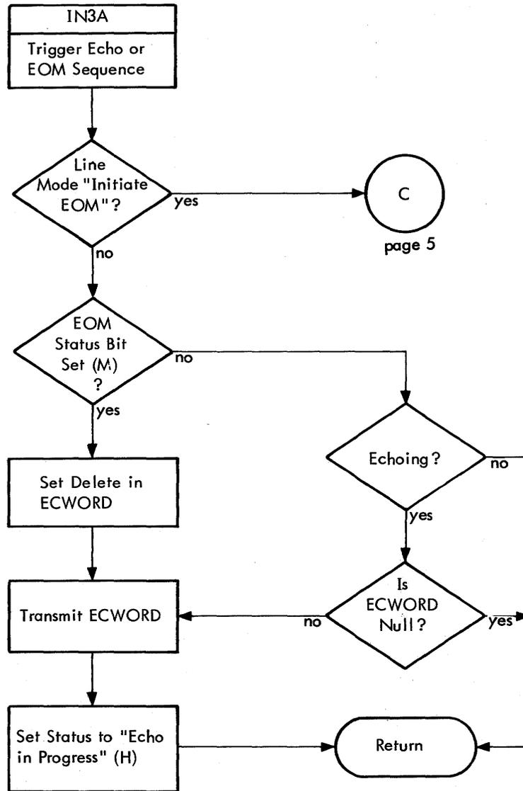
Figure 73. R:COG Input Interrupt Handler (cont.)
