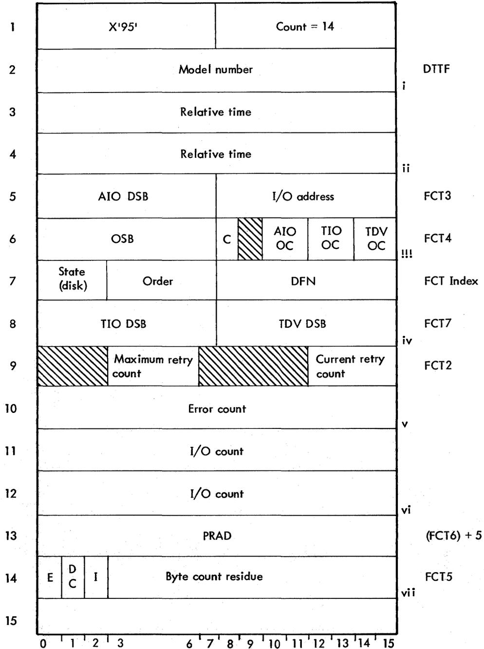
Figure 90. I/O-Error Entry
