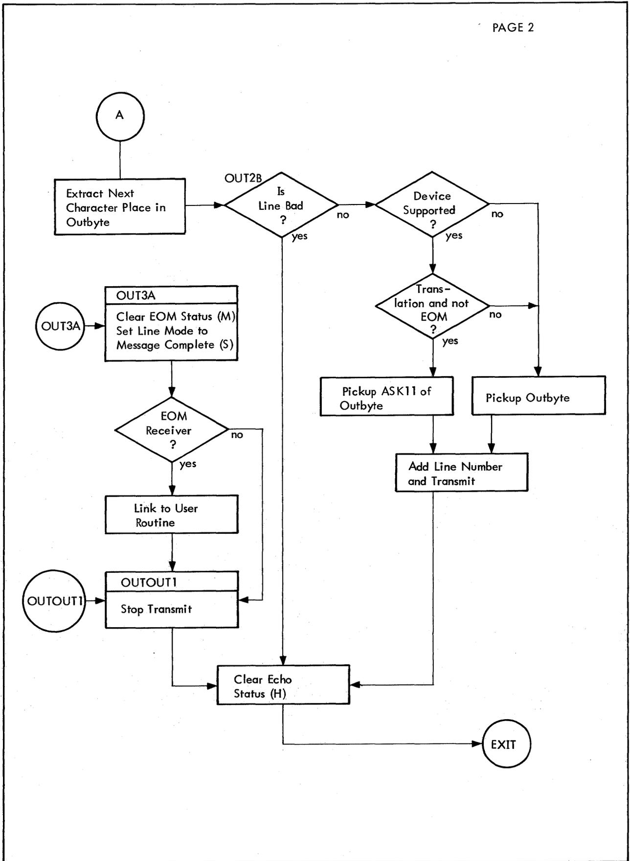
Figure 74. R:COG Output Interrupt Handler (cont.)
