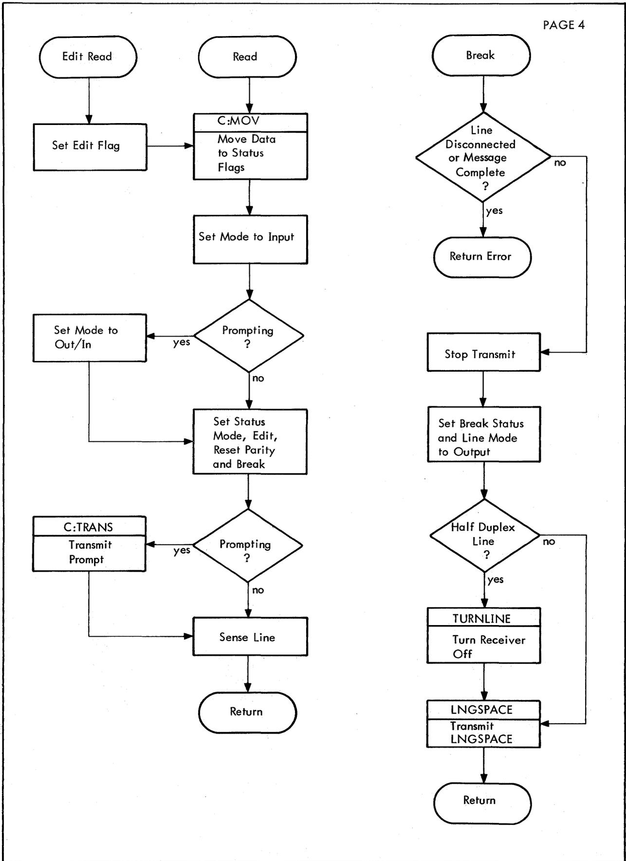
Figure 76. M:COC Request Processing (cont.)
