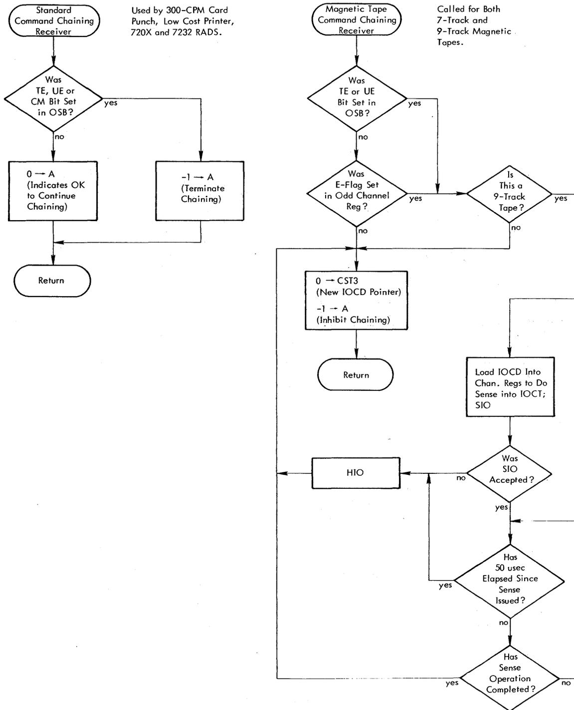
Figure 3. RBM Input/Output Task Flow (cont.)
