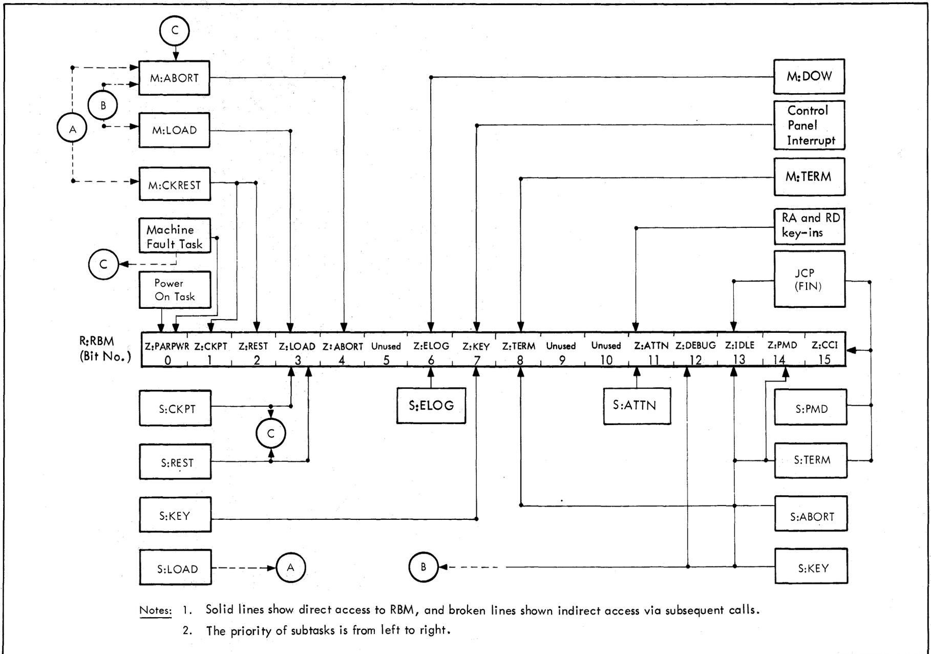
Figure 13. RBM Control Task Status Word (R:RBM)
