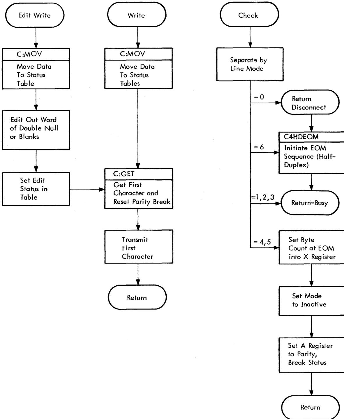
Figure 76. M:COC Request Processing (cont.)
