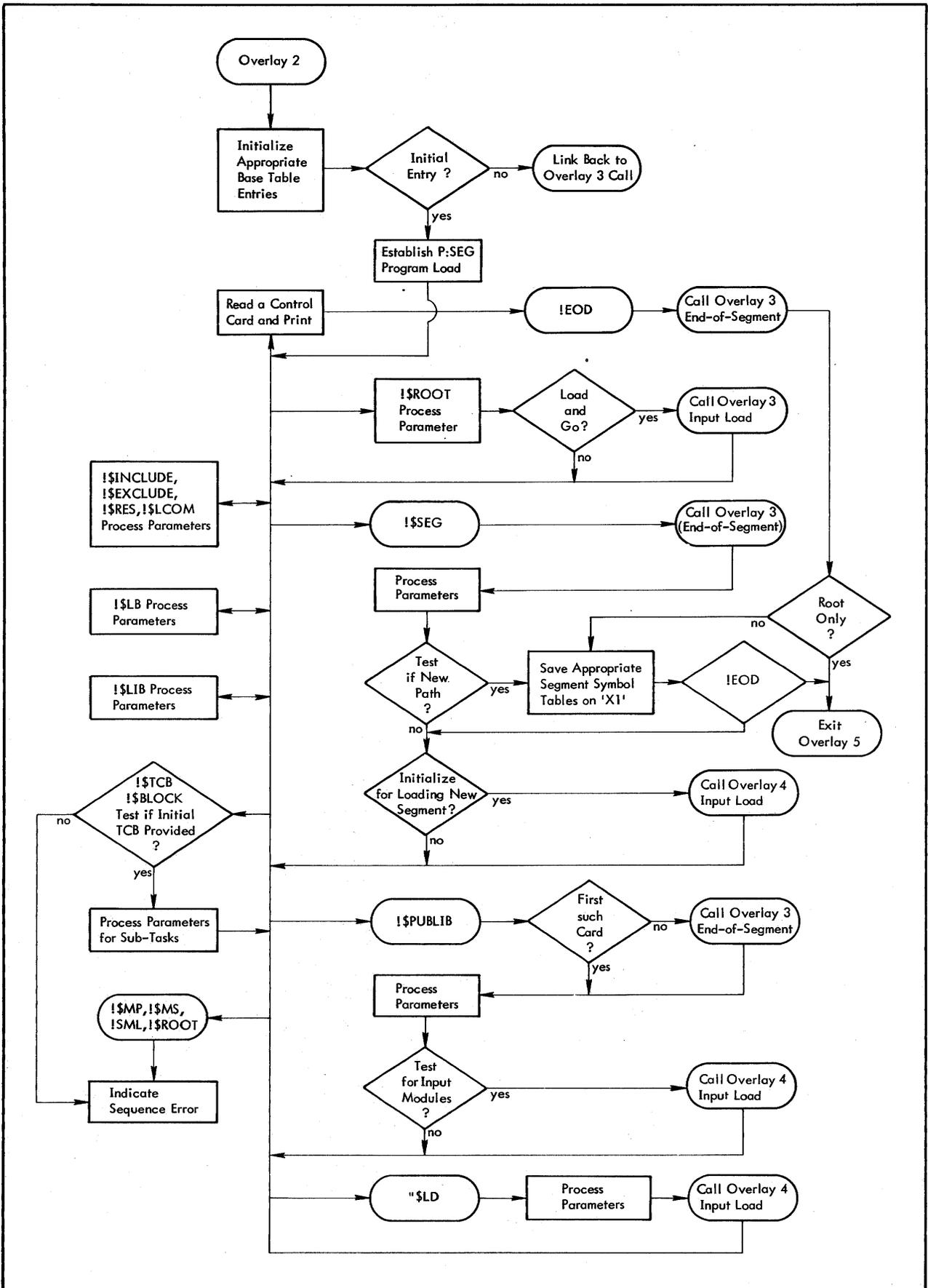
Figure 47. Overlay 2 Structure
