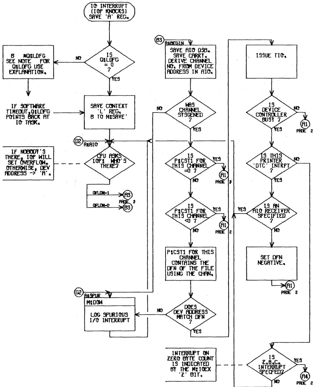
Figure 3. RBM Input/Output Task Flow
