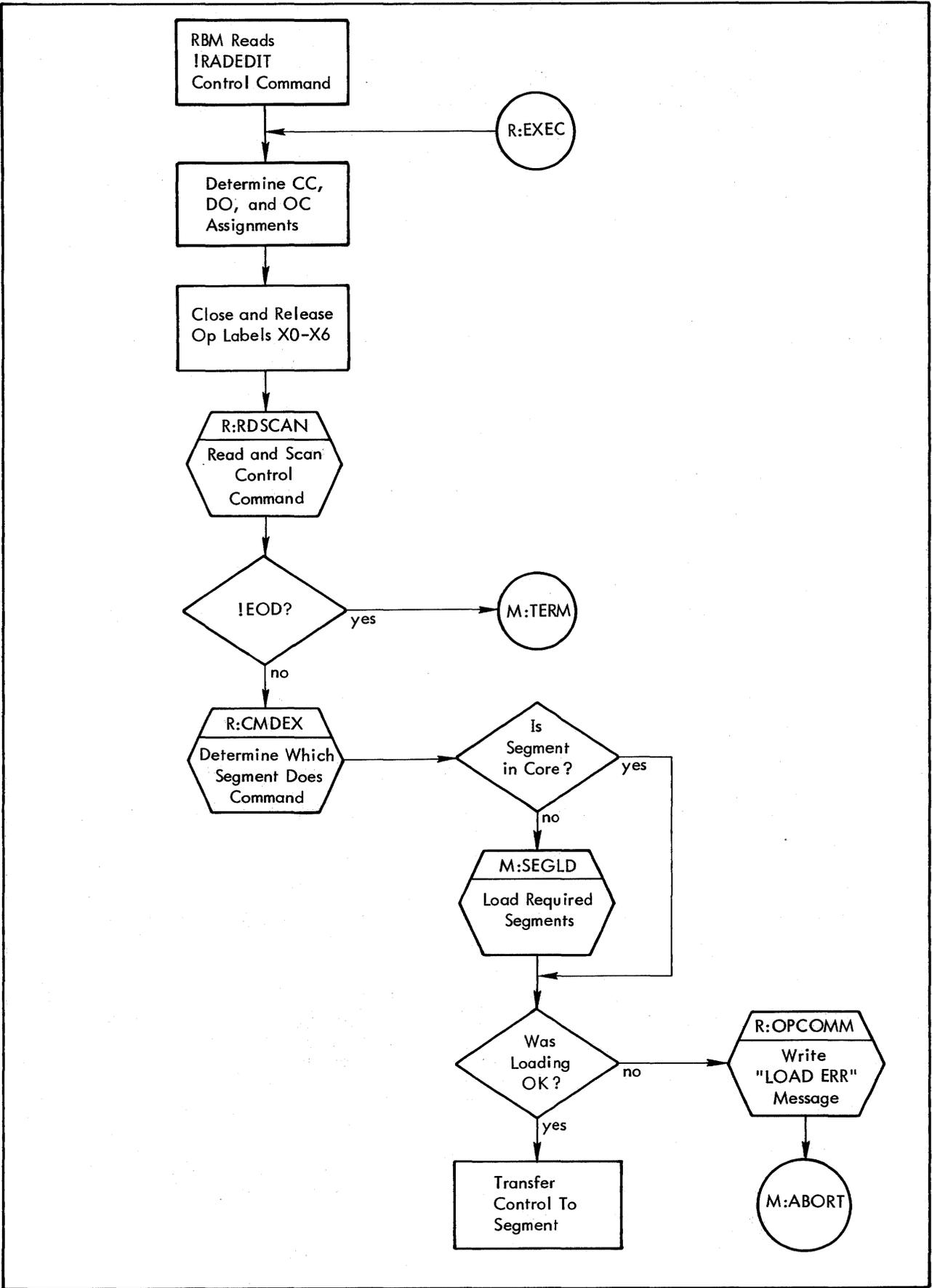
Figure 69. Control Command Execution Flow
