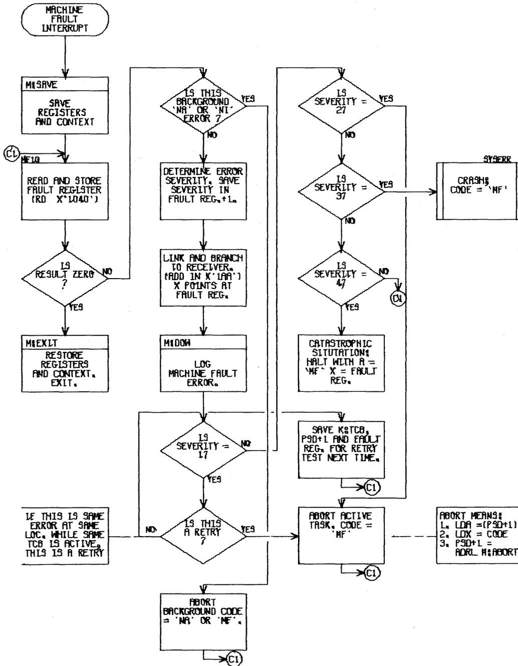
Figure 1. RBM Machine Fault Task Flow
