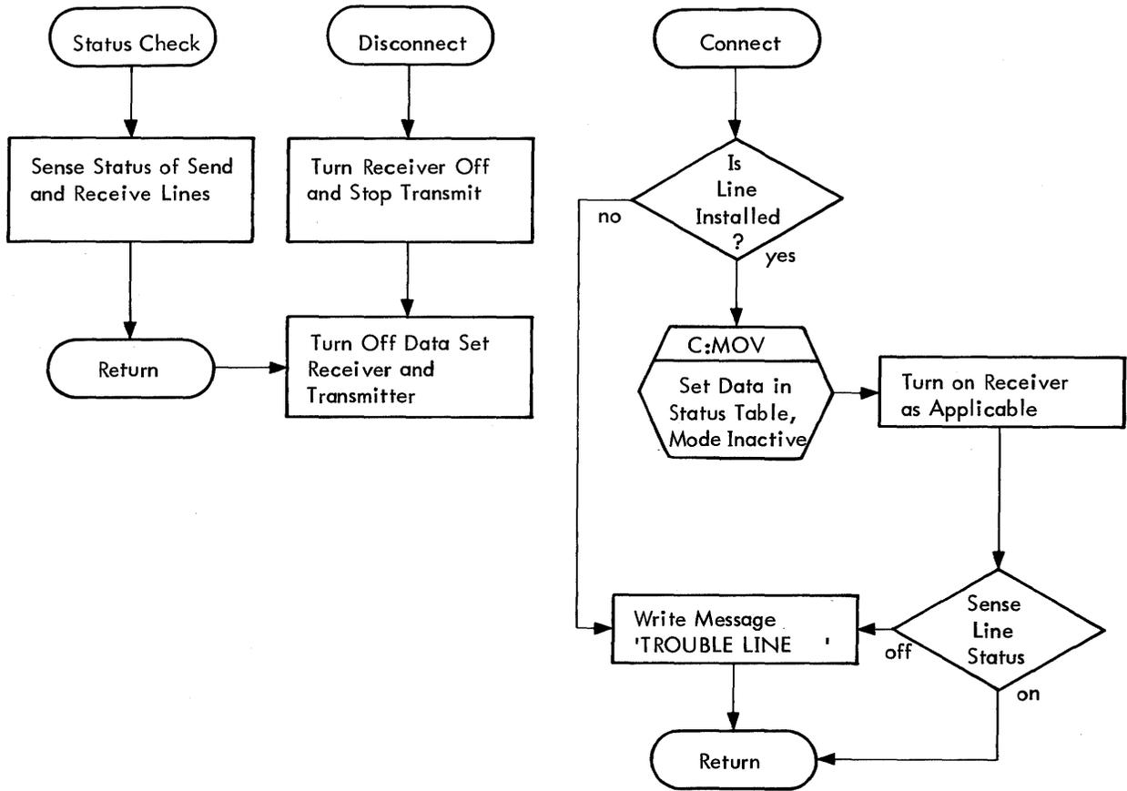
Figure 76. M:COC Request Processing (cont.)
