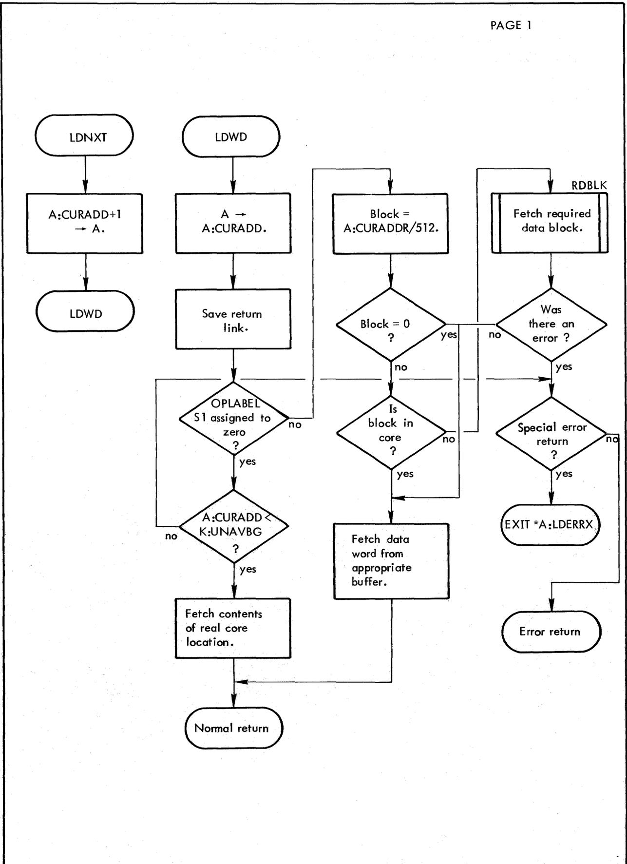
Figure 78. Data Acquisition Subroutines LDWD and LDNXT
