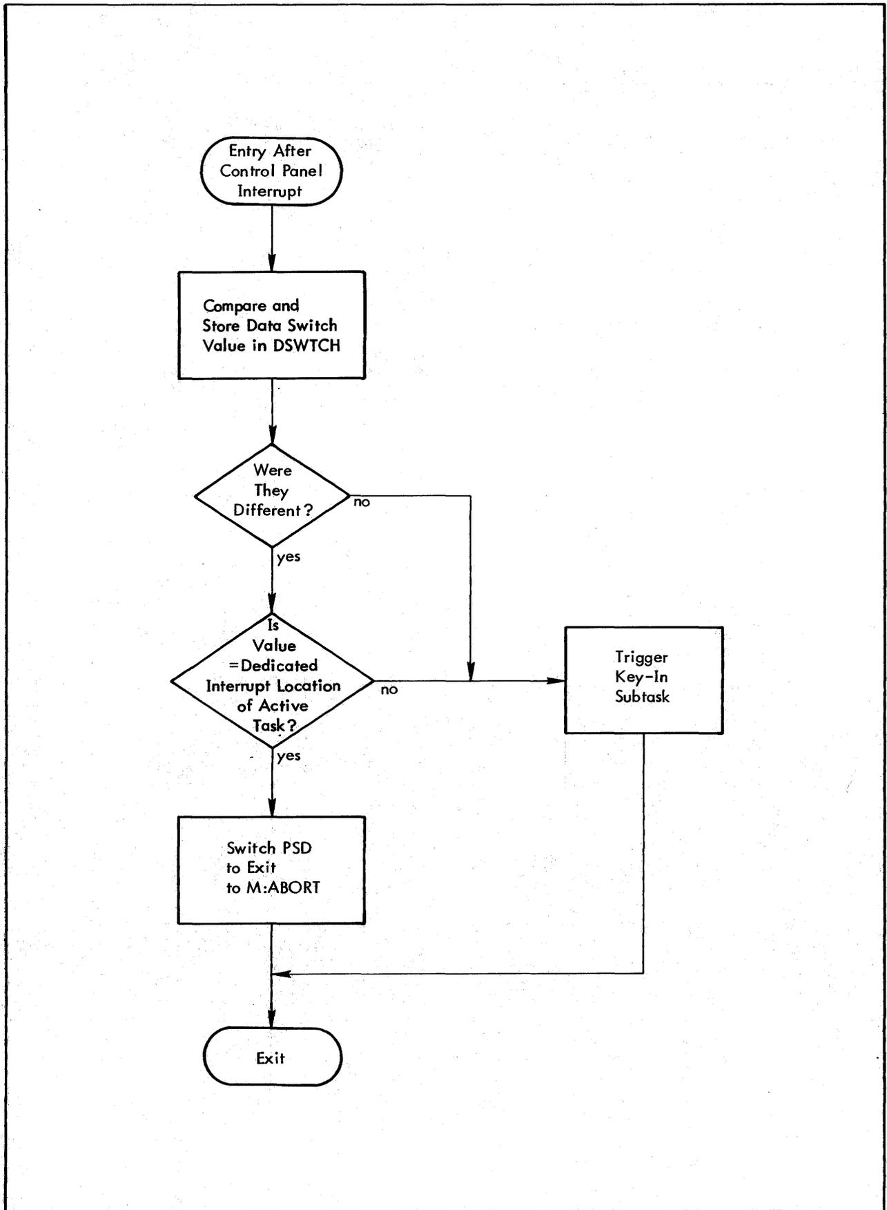
Figure 4. RBM Control Panel Task Flow
