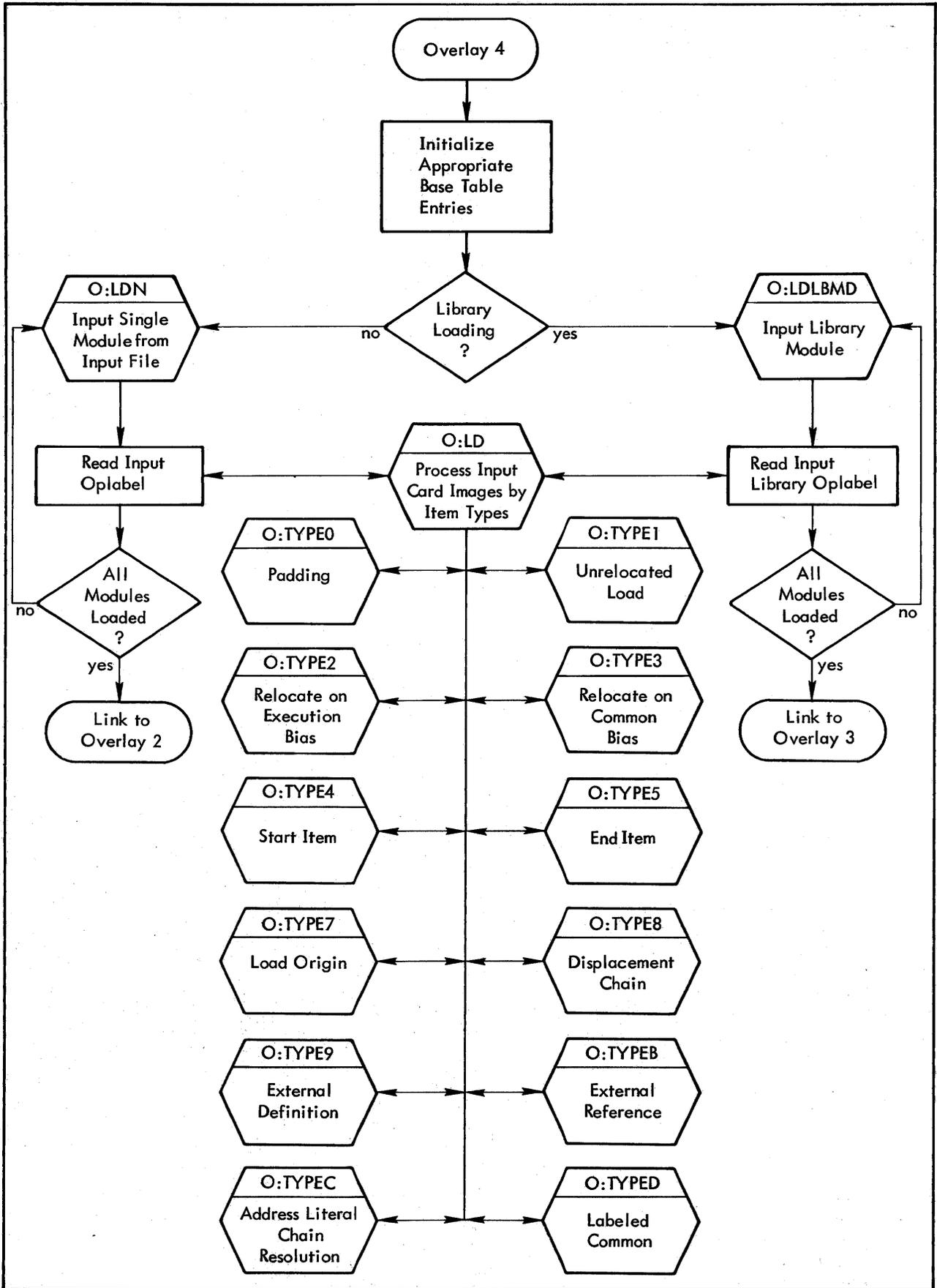
Figure 49. Overlay 4 Structure
