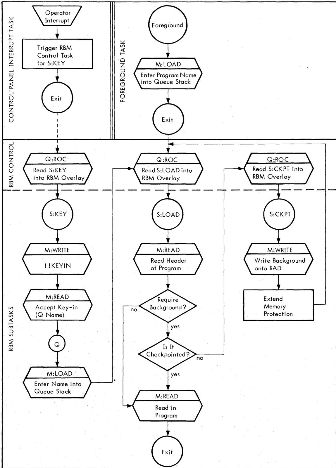
Figure 18. Queue Stack Loading of Foreground Processors
