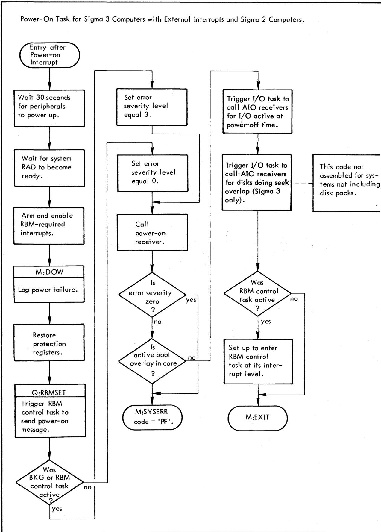
Figure 14. Power-On/Power-Off Tasks
