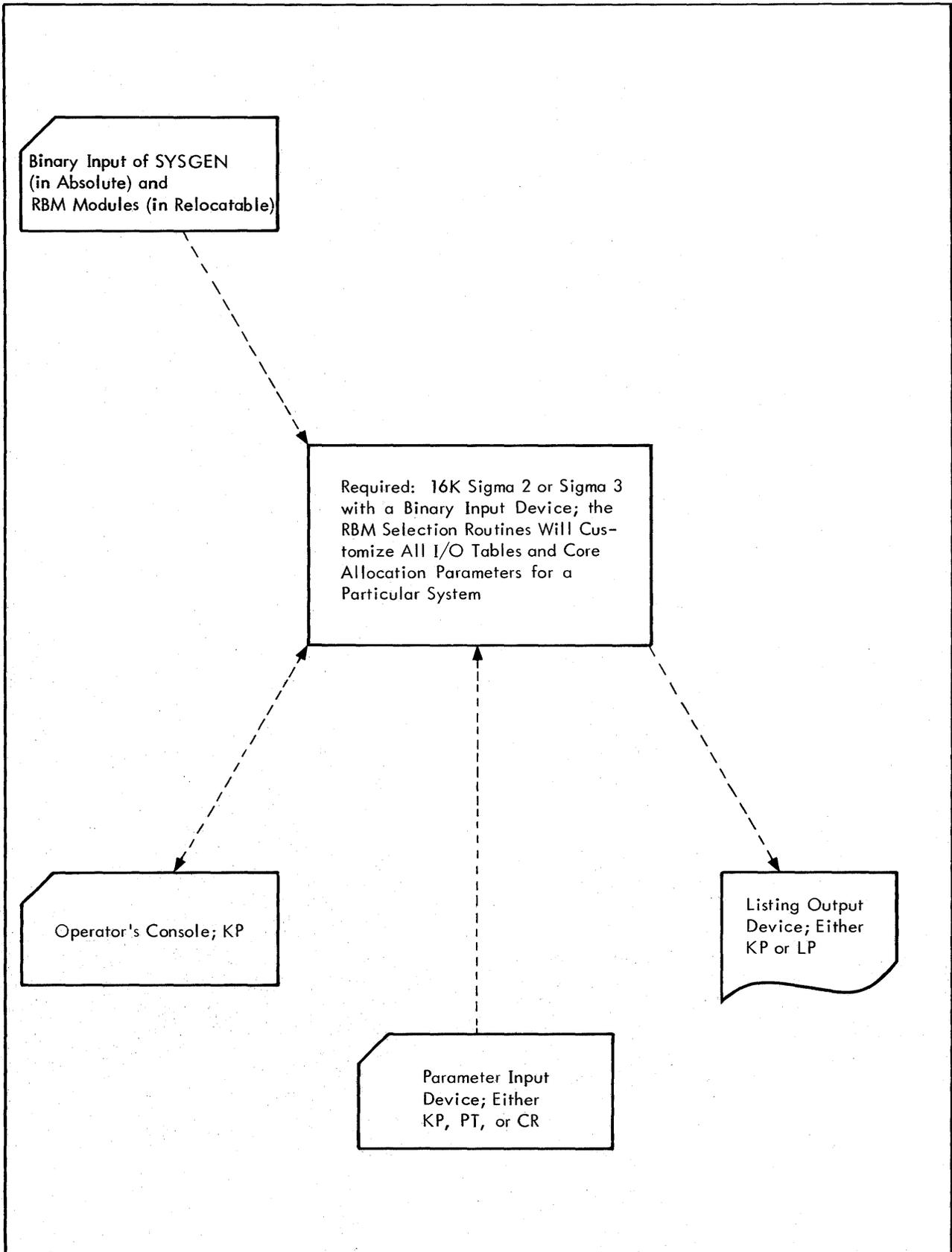
Figure 11. RBM Selection Operation
