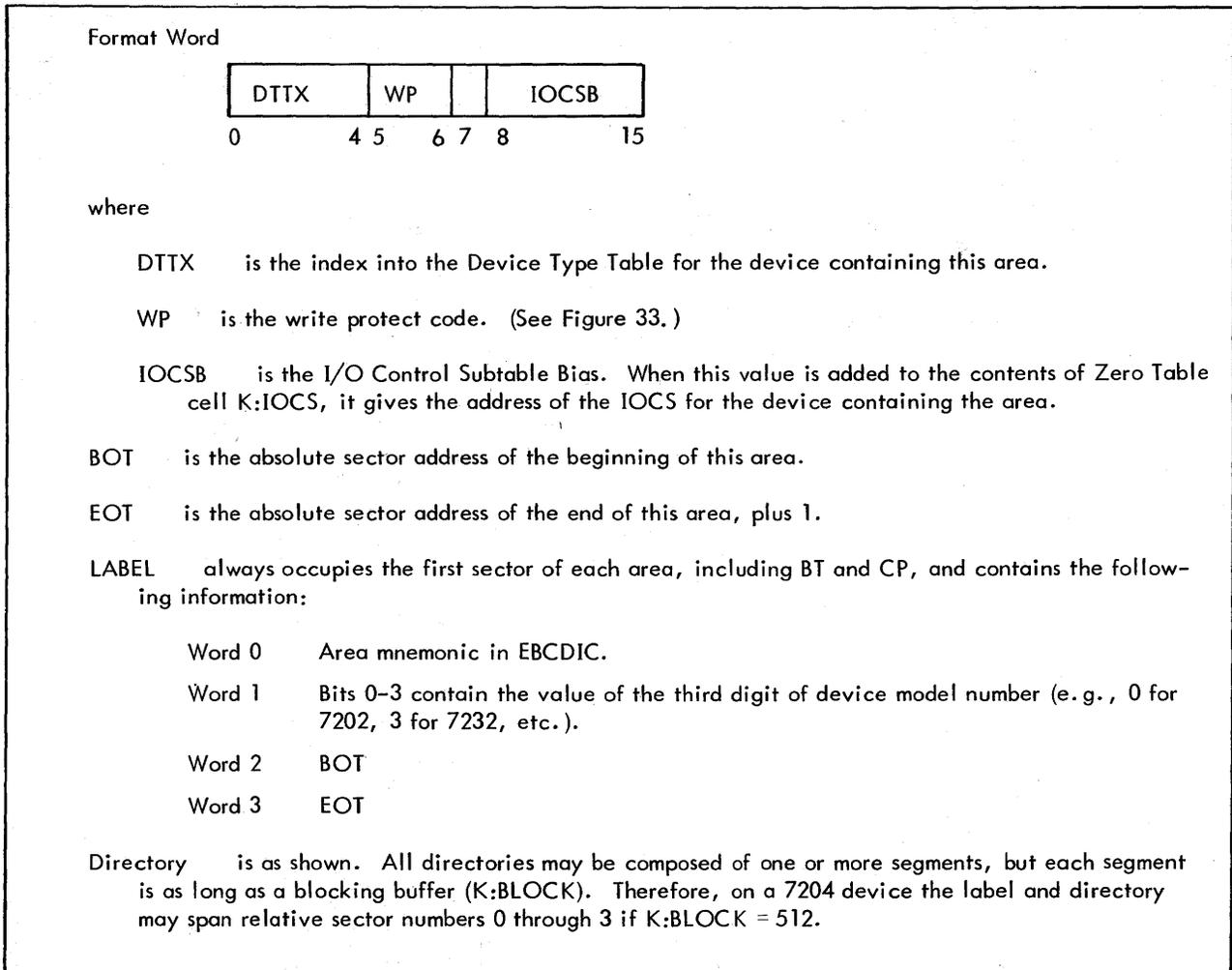
Figure 39. Permanent RAD File Layout (RAD Area N Containing M Files) (cont.)
