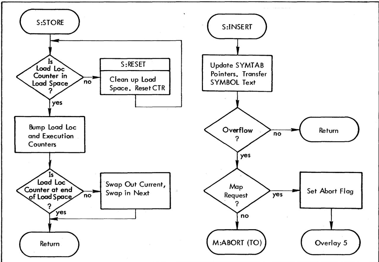
Figure 65. Overlay 10 Structure
