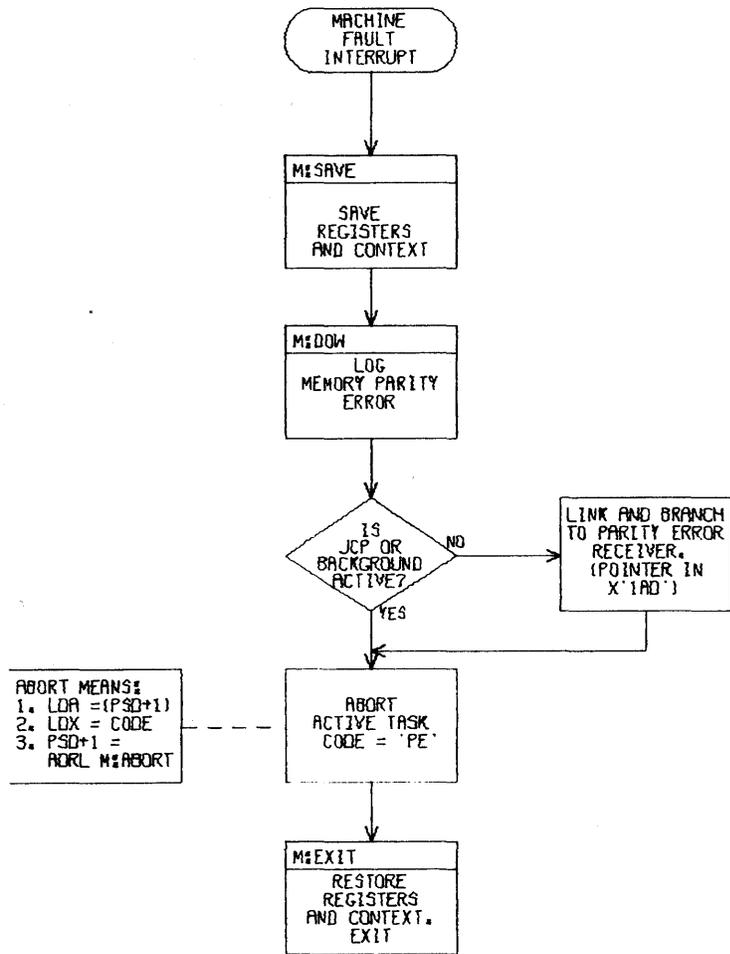
Figure 1. RBM Machine Fault Task Flow (cont.)
