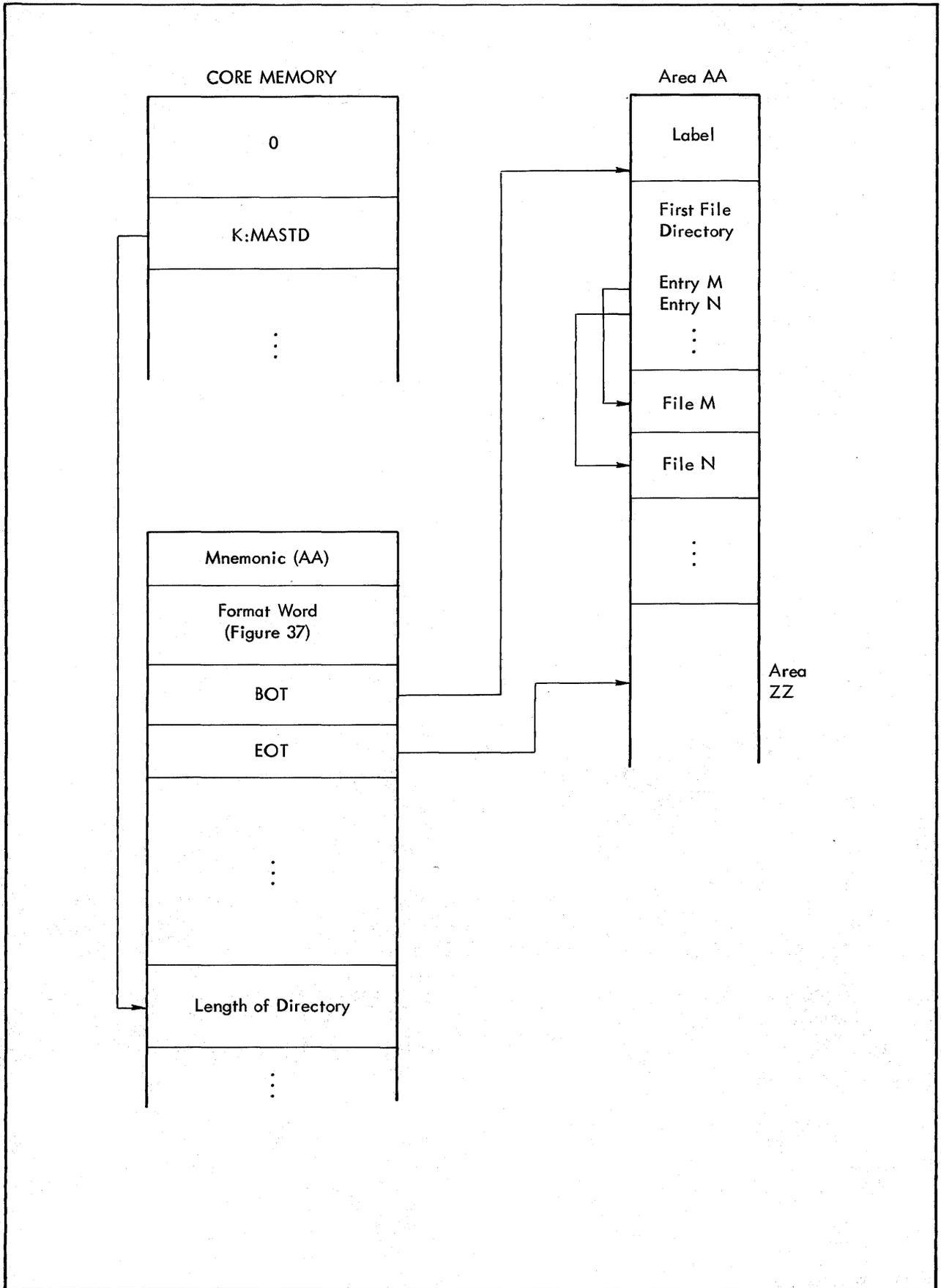
Figure 67. RBM File Structure
