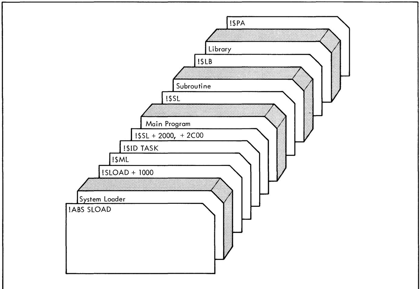
Figure 10. Deck Set-up to Generate a Foreground Program
