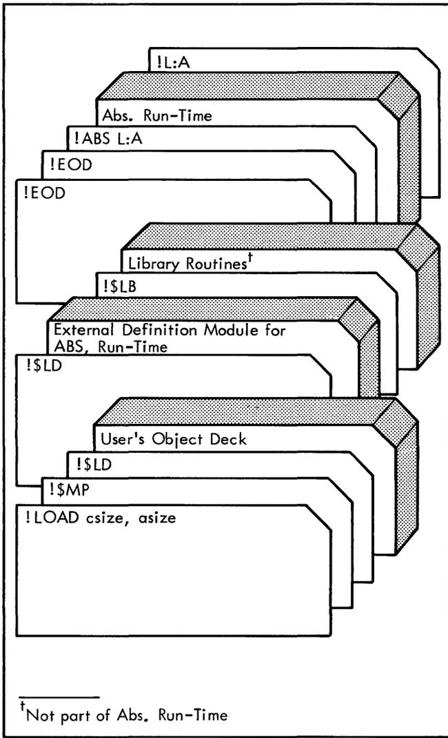
Figure 7. Overlaying Linking Loader for Absolute Run-Time
