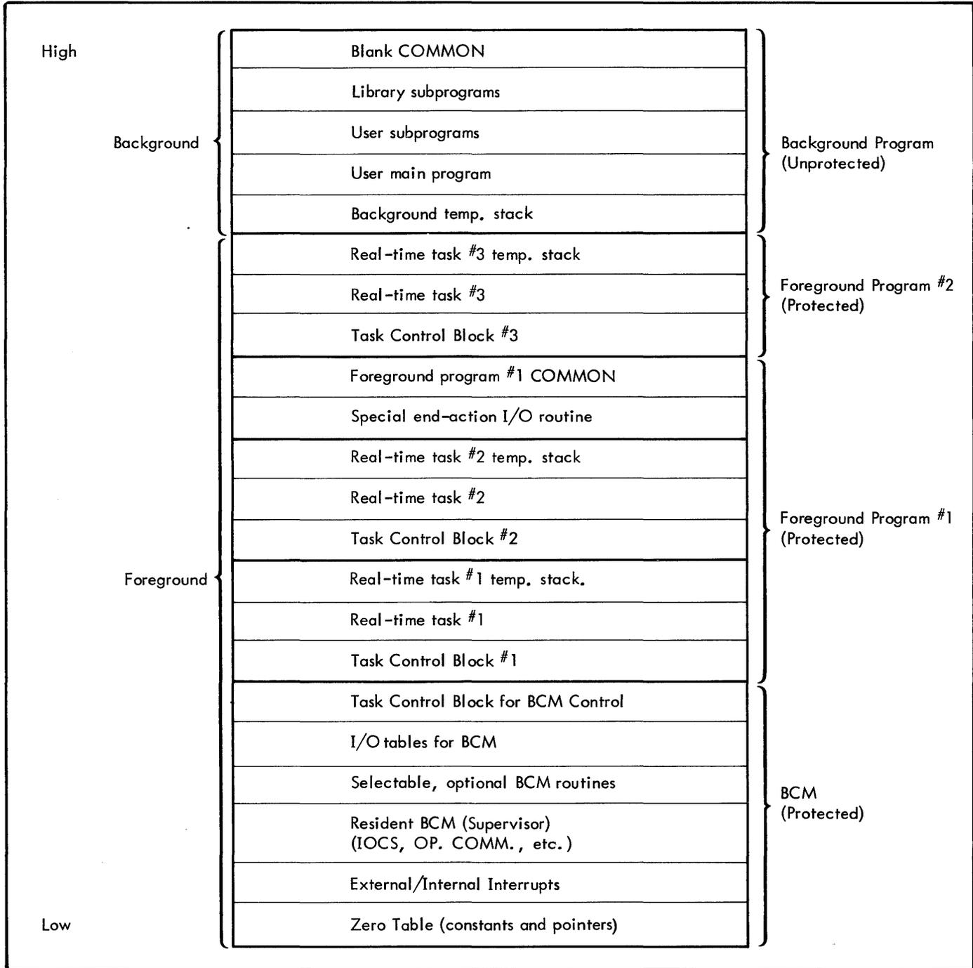
Figure 2. BCM Core Memory Allocation (Example)
