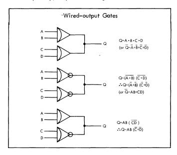
The trade-off for this additional logic capability is a reduction of fan-out. Each additional output absorbs 2 unit loads due to the additional 560 ohm pull-up resistor that is placed in parallel at the node. No more than seven outputs can be connected since seven pull-ups absorb 14 unit loads, leaving 2 unit loads for useful output.
