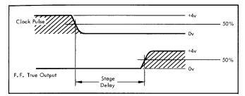
Minimize Delay Due To Wiring
