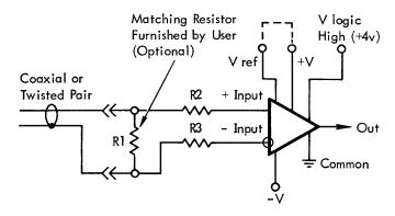
Connection Diagram, One Circuit
