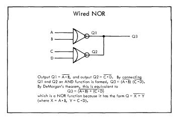
The basic wired functions that can be formed with two outputs are given below. Up to seven outputs, each having a 560 ohm pull-up, may be wired together.
