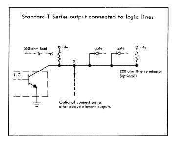
If all outputs are inverter outputs the wired gate can be considered a NOR as shown below.
