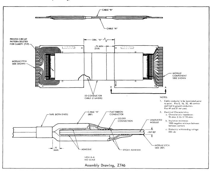
Two ribbons are always run in parallel; their edges are sewn together with nylon thread for handling convenience. This provides a total of 104 conductors per cable: Fiftyfour ground conductors and fifty signal conductors.
