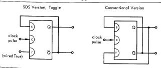
The flip-flop may also be used as a straight clocked set-reset (R-S)flip-flop with the s and r inputs activated directly, or asynchronously with d-c inputs, mark (m) and erase (e), which override the s and r inputs. Note that in clocked R-S operation there is no ambiguity because set overrides reset.
