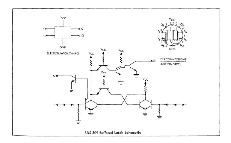
This type of logic is commonly referred to as set-overridereset logic. If the set and reset inputs are true at the same time, the output will follow the set input.
