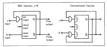
The same feature saves an inverter and reduces wiring in the Delay mode of operation. When the reset input is left open (wired True) the set input operates the circuit as a delay flip-flop--that is, the Q output state follows the set input state, delayed by one clock pulse period.
