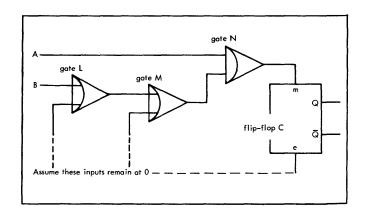
Obviously the problem is avoided if the output of gate N is not allowed to change flip-flop C state until after all signals have settled. The trailing edge trigger clock technique provides the longest possible settling time.
