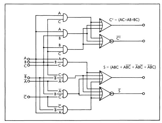
Single Full-adder Circuit (four per module)
