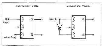
This feature also saves wiring in the Toggle mode. In this mode the clock input operates the circuit, causing it to change state at each clock trigger.
