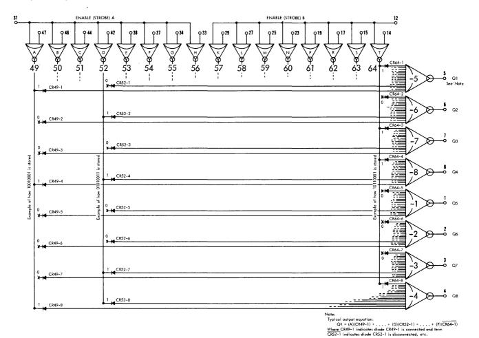
The ORing characteristic makes it possible to store more than sixteen 8-bit bytes per module, providing that more than one input is raised at once, and providing the resulting pattern is not already present on the module.
