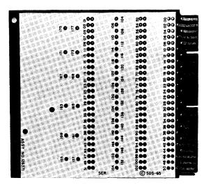
ZTI5 Cable Plug Module (Soldered Connections)
