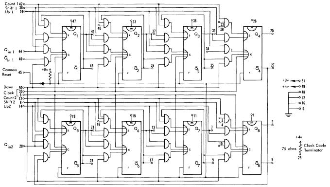
1. Mark inputs must be grounded when not in use. 2. Subscripts refer to ckt. number. Example: Up 2 is Up control line for ckt. 2
